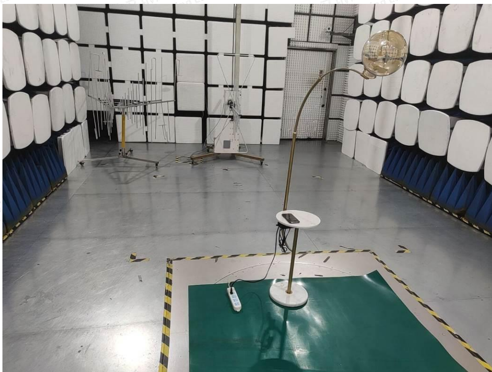
Radiated Emission from 30MHz to 1GHz
