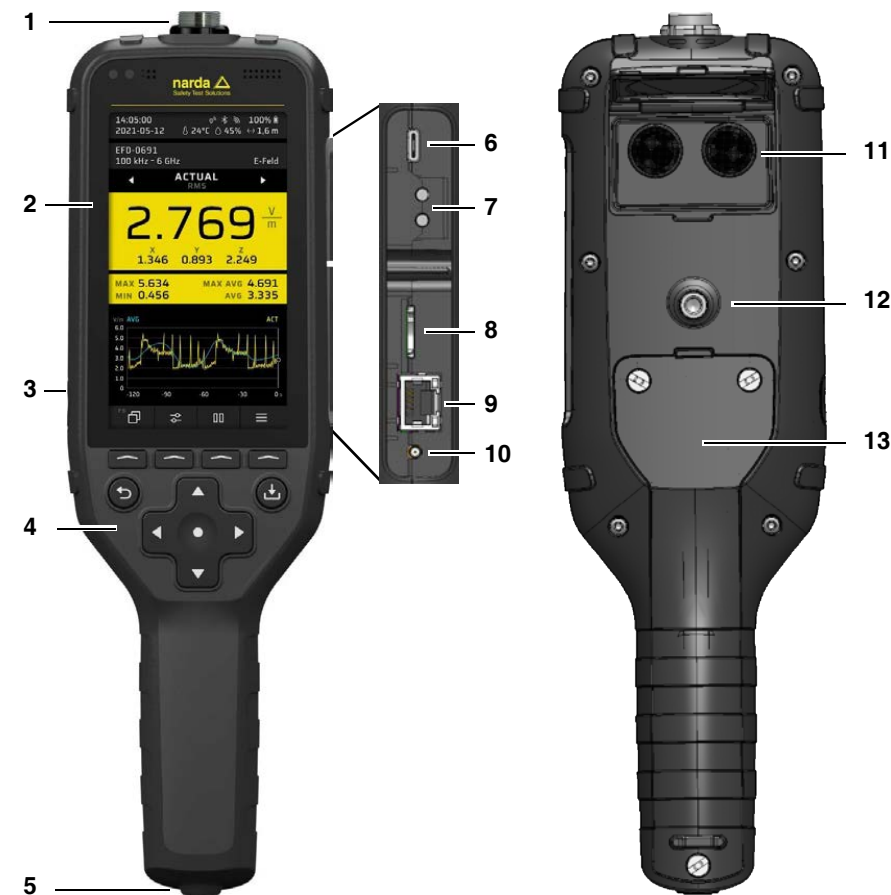
Fig. 2: Device overview FieldMan
