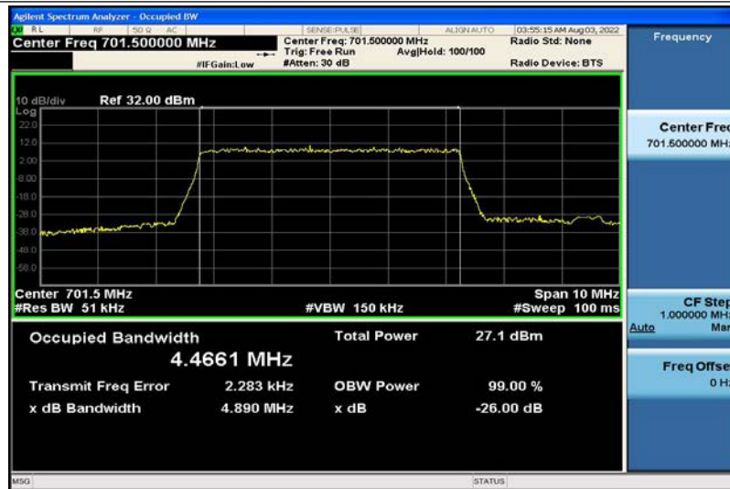
Band12-5MHz-QPSK-23035-25RB#0-4.4661
