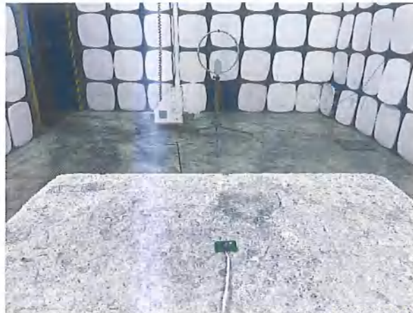
Radiated Emission Test Set-up for Below 30MHz
