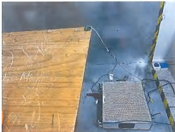
Radiated Emission Test Set-up for 30M-1GHz
