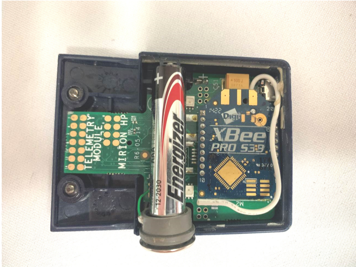
Figure 5. Transmitter Section, Top cover removed
