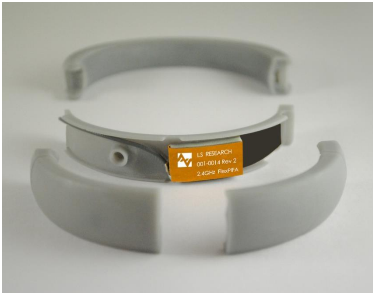
Figure 28: FlexPIFA integrated into bracelet
