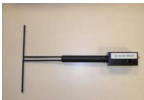
Figure 1 – Satimo COMOSAR Validation Dipole
