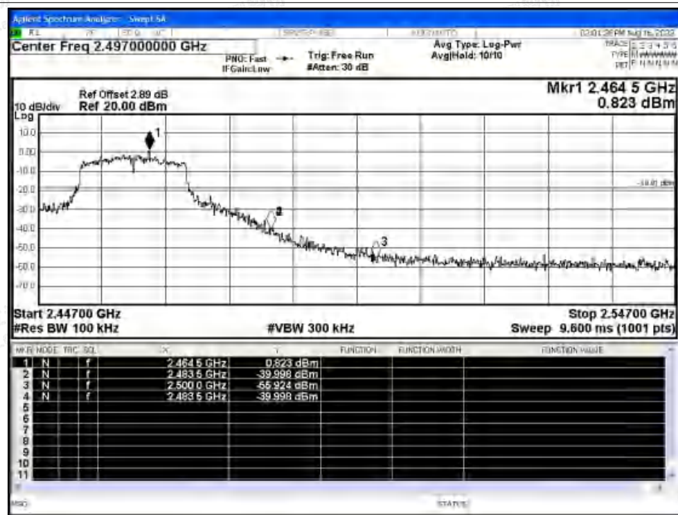
Band Edge NVNT g 2462MHz Ant1 Emission
