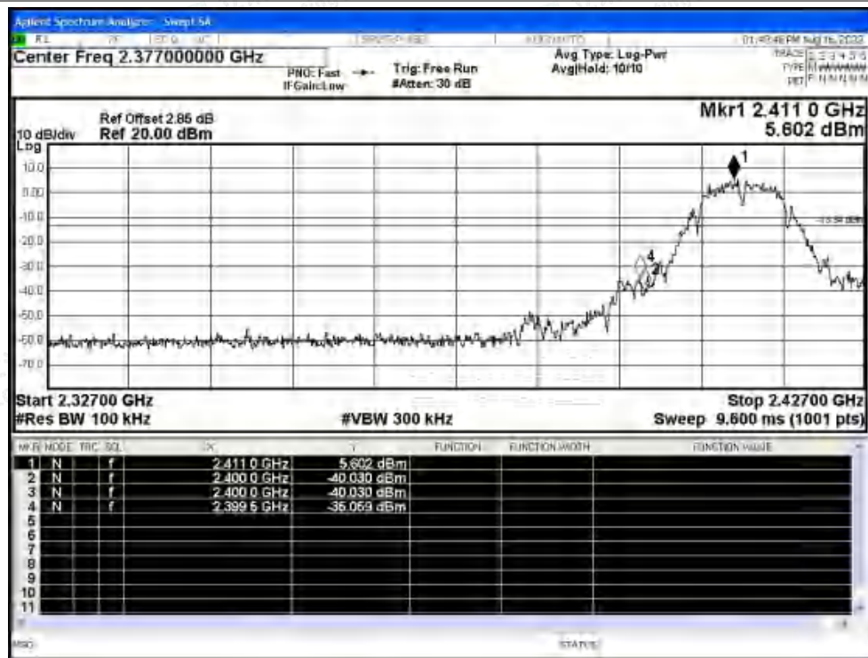
Band Edge NVNT b 2412MHz Ant1 Emission
