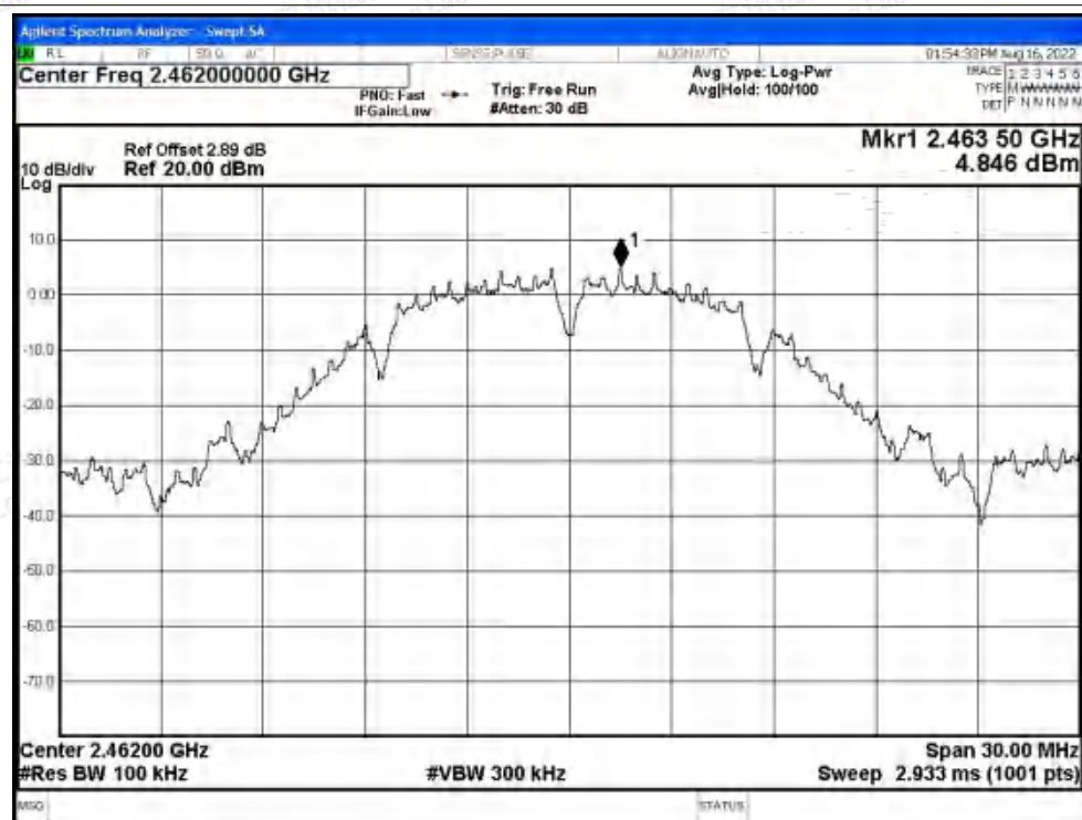
Tx. Spurious NVNT b 2462MHz Ant1 Emission
