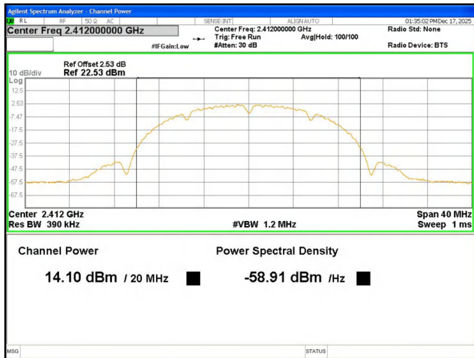
Average Power NVNT b 2412MHz Ant1
