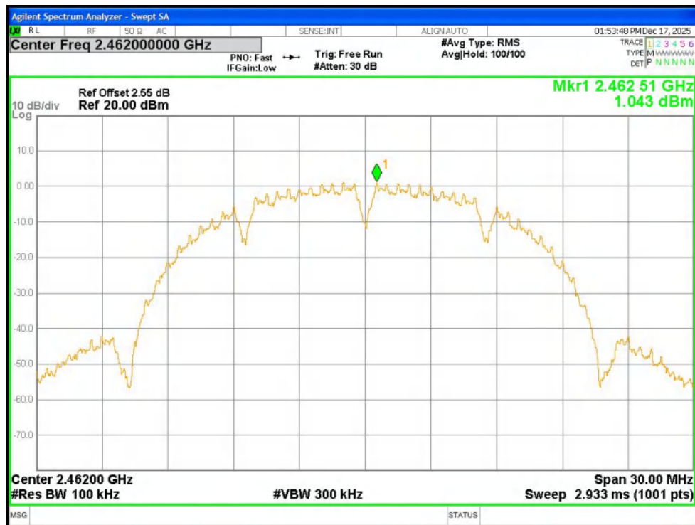
Tx. Spurious NVNT b 2462MHz Ant1 Ref
