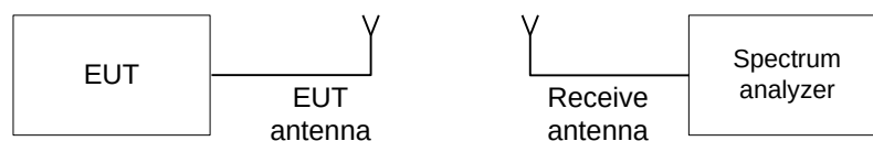
Figure 7.1.1 The 20 dB bandwidth test setup
