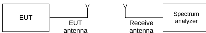
Figure 7.4.1 Average time of occupancy test setup
