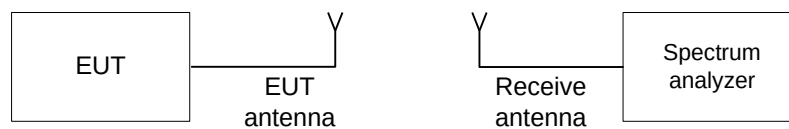
Figure 7.7.1 Band edge emission test setup
