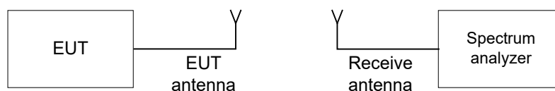
Figure 7.4.1 Average time of occupancy test setup
