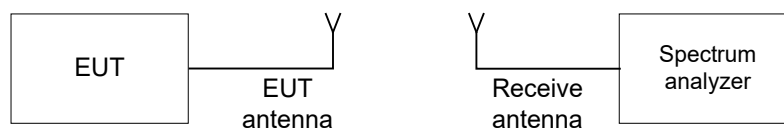
Figure 7.2.1 Carrier frequency separation test setup
