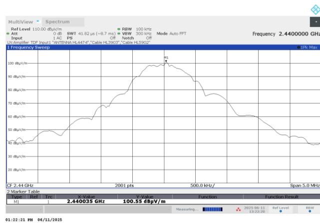
Plot 7.10.2 Peak spectral power density at mid frequency
