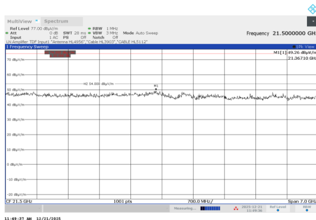
Plot 7.6.14 Radiated emission measurements from 18000 to 25000 MHz at the mid carrier frequency
