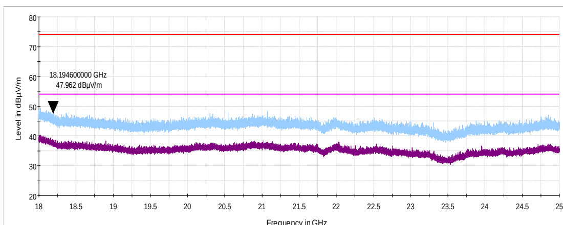
Plot 7.7.14 Radiated emission measurements from 18000 to 25000 MHz at the mid carrier frequency
