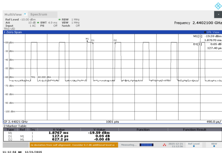
Plot 7.6.49 Transmission pulse duration and period
