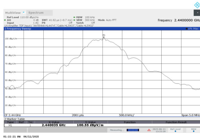
Plot 7.8.2 Peak spectral power density at mid frequency
