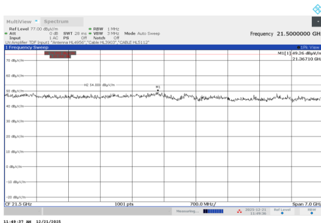
Plot 7.5.14 Radiated emission measurements from 18000 to 25000 MHz at the mid carrier frequency
