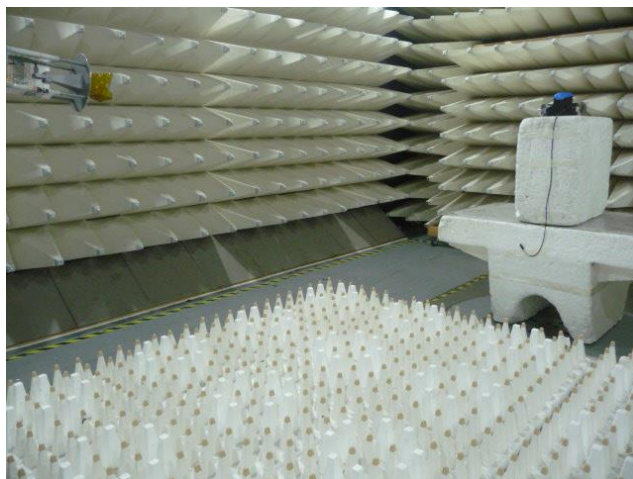
Photograph No.4 Setup for spurious emission field strength measurements in the anechoic chamber in 18-40 GHz range for Digital water meter
