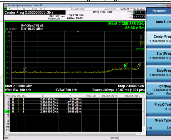
Left Band edge hopping on
