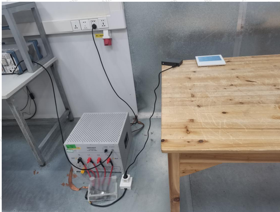
Photo of Power Line Conducted Emission Test
