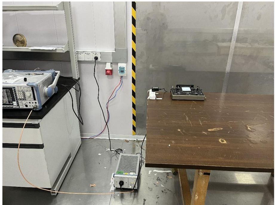
Conducted Emission Test Setup
