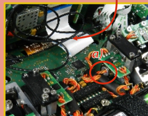
Proper arrangement of the display flat, flexible cable.
