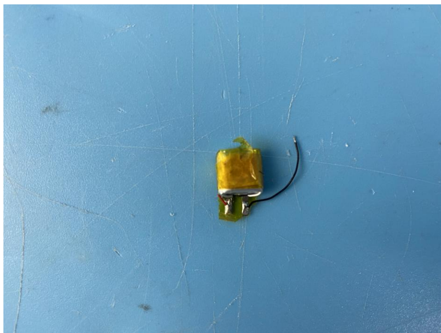
INTERNAL PHOTO OF BATTERY
