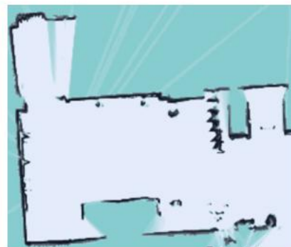
The map scanned by the robot's laser
