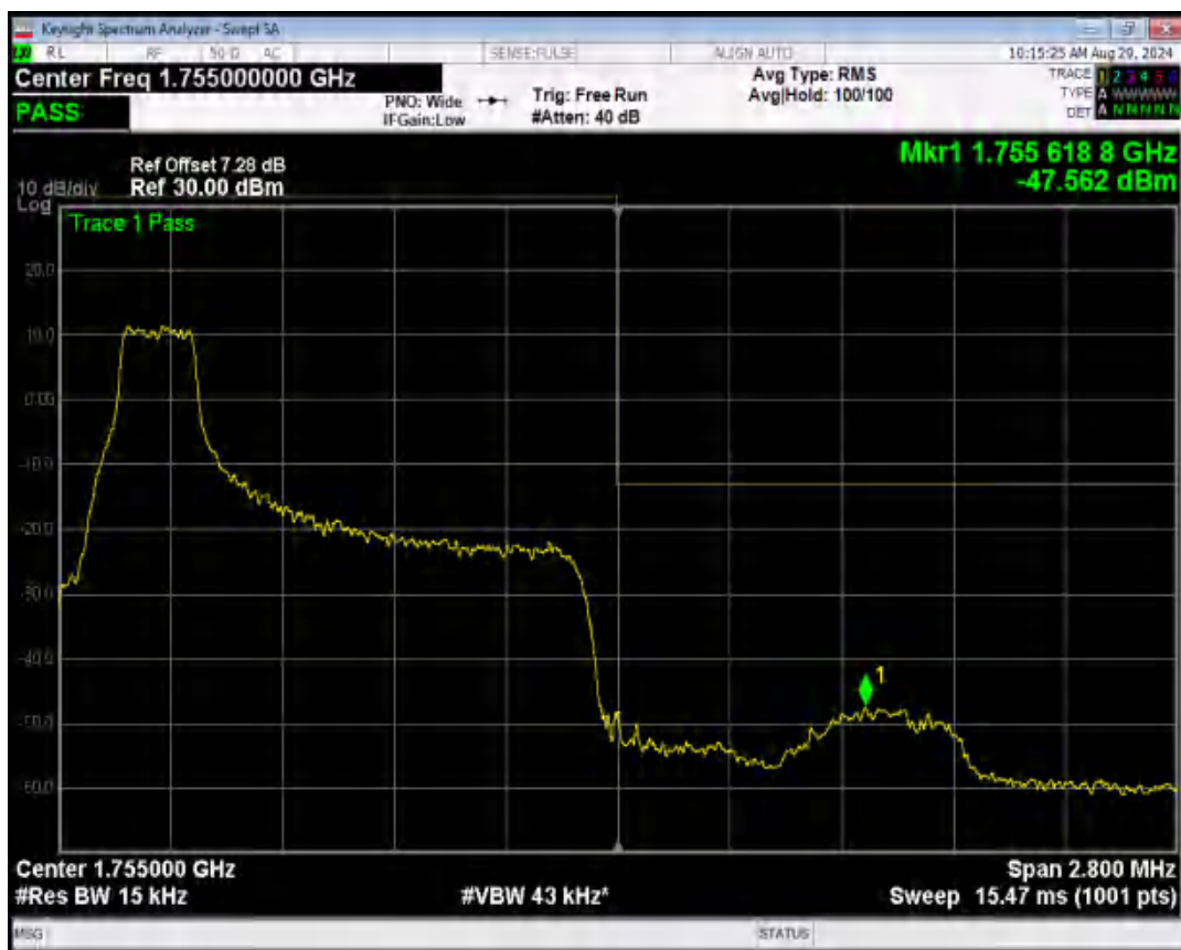
Band4 16QAM BW=1.4MHz Channel=20393 RB Size=1 Position=#Max
