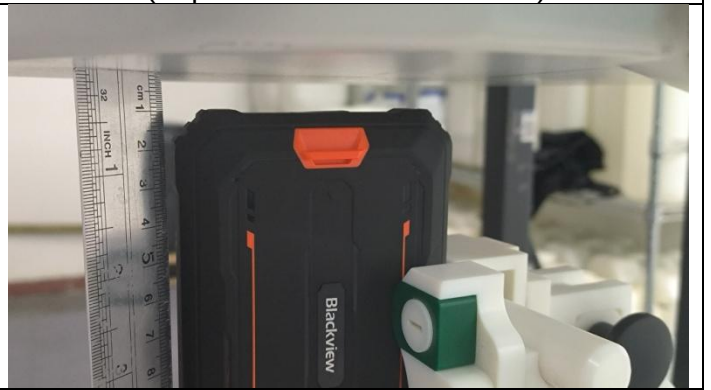
Bottom Side (Separation distance of 10mm)
