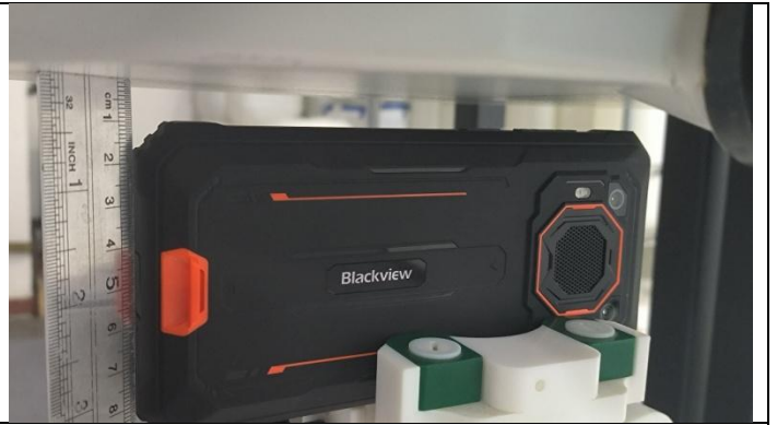
Bottom Side (Separation distance of 10mm)
