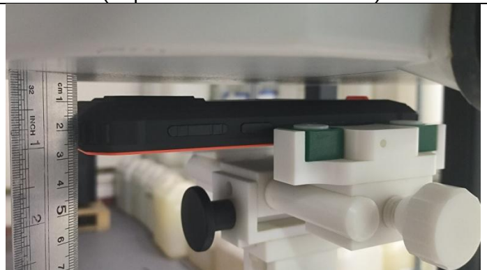
Right Side (Separation distance of 10mm)
