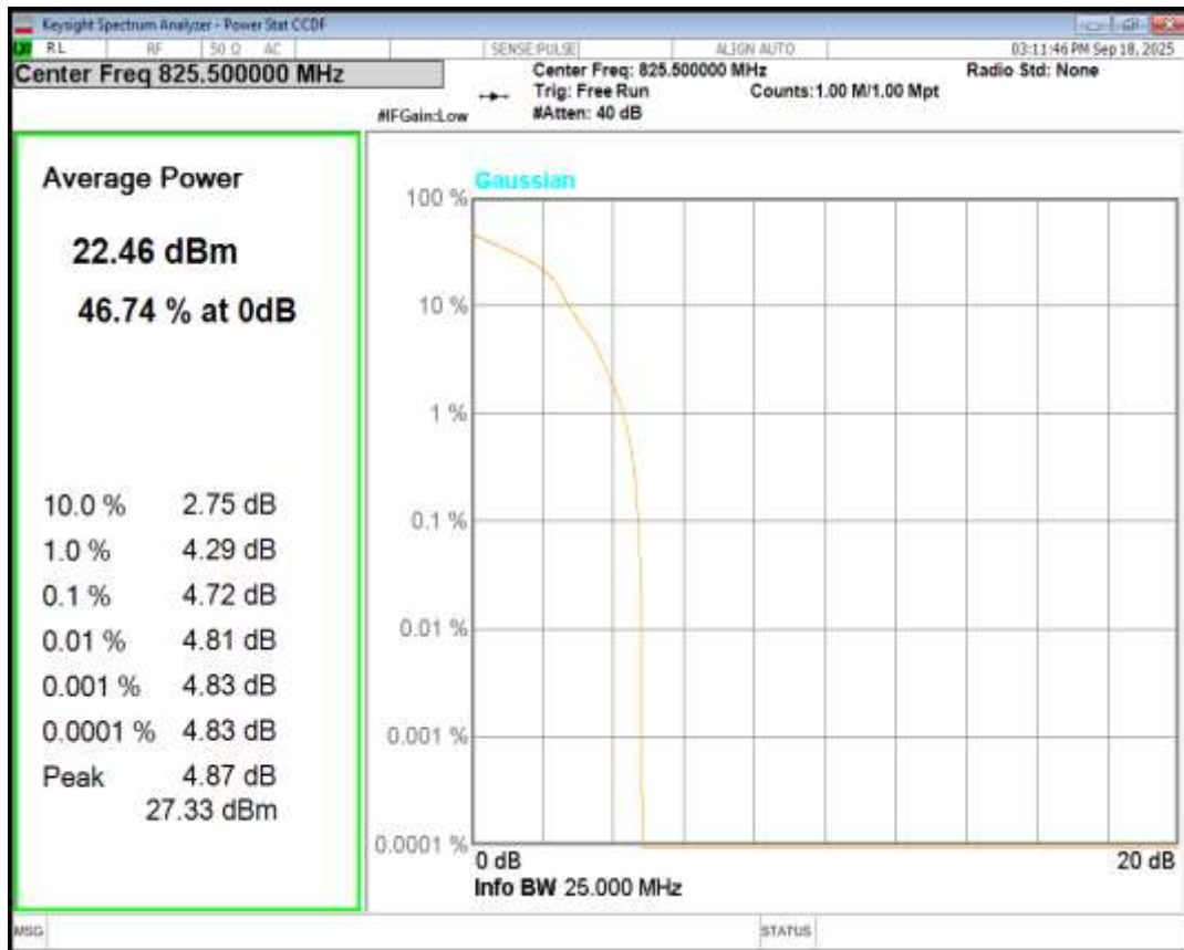
Band5 16QAM BW=3MHz Channel=20525 RB Size=1 Position=#0
