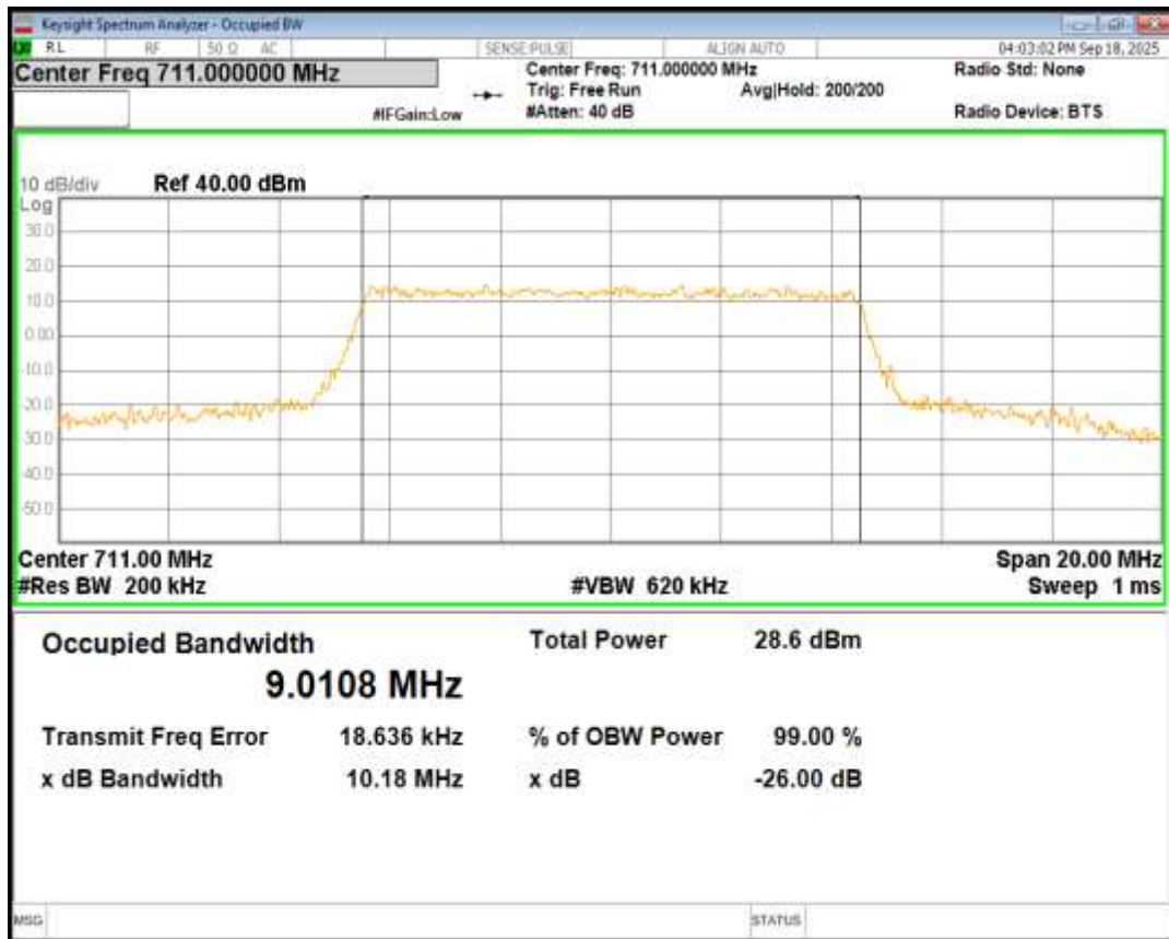
Band17 16QAM BW=5MHz Channel=23755 RB Size=25 Position=#0
