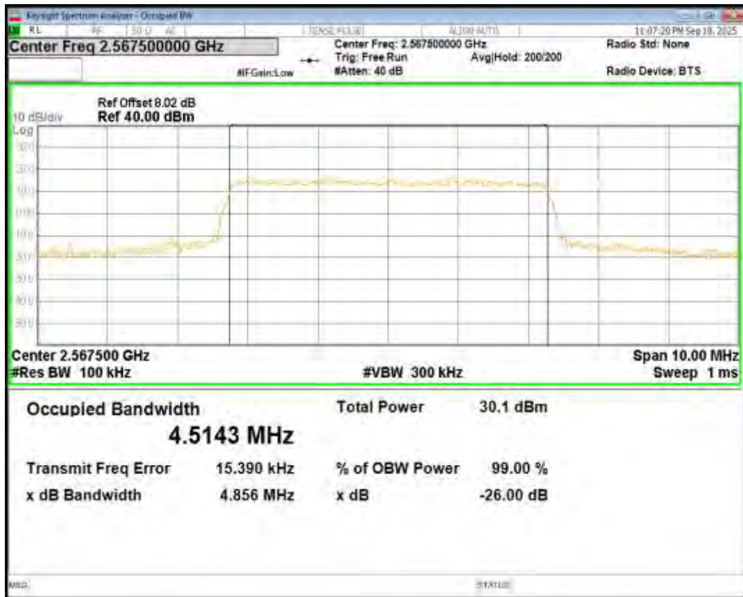
Band7 16QAM BW=5MHz Channel=21100 RB Size=25 Position=#0
