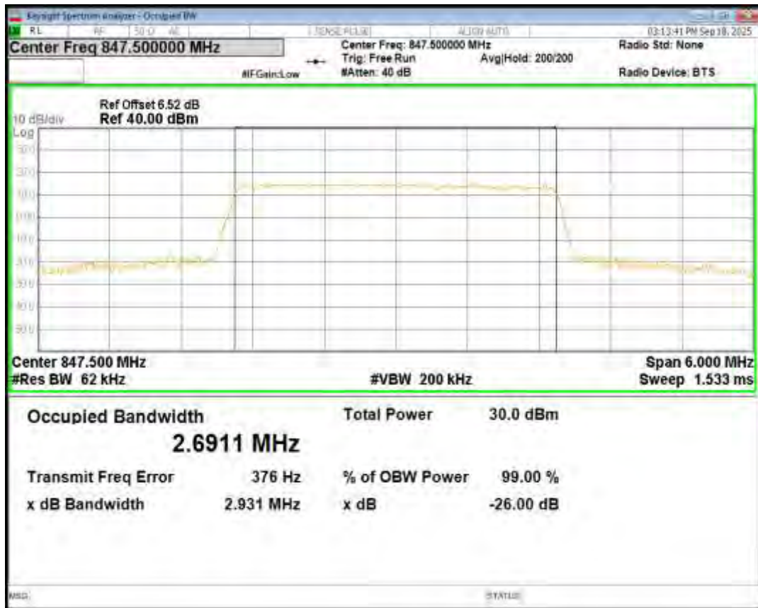
Band5 16QAM BW=5MHz Channel=20425 RB Size=25 Position=#0
