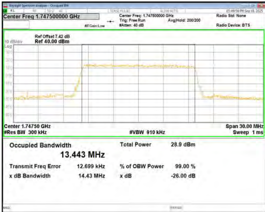
Band4 QPSK BW=20MHz Channel=20050 RB Size=100 Position=#0
