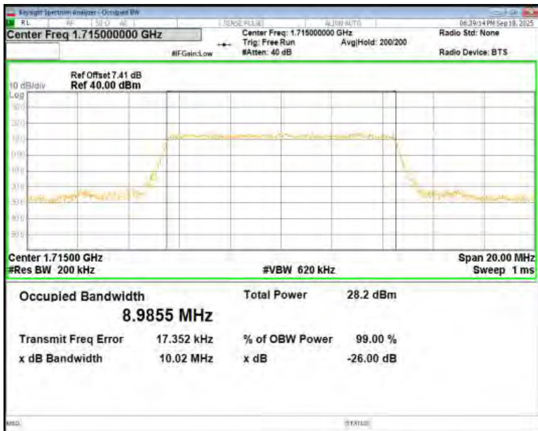
Band66 16QAM BW=10MHz Channel=132322 RB Size=50 Position=#0
