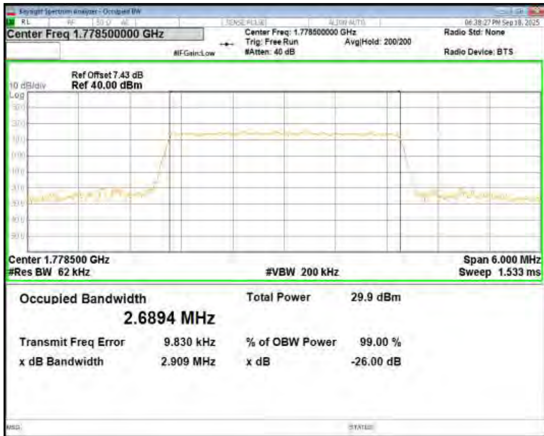
Band66 QPSK BW=5MHz Channel=131997 RB Size=25 Position=#0
