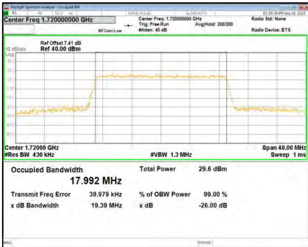
Band4 QPSK BW=20MHz Channel=20175 RB Size=100 Position=#0
