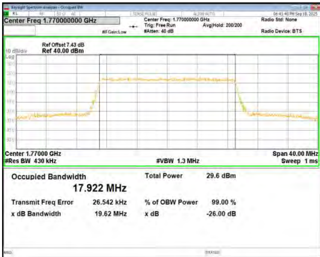
Band66 QPSK BW=3MHz Channel=131987 RB Size=15 Position=#0
