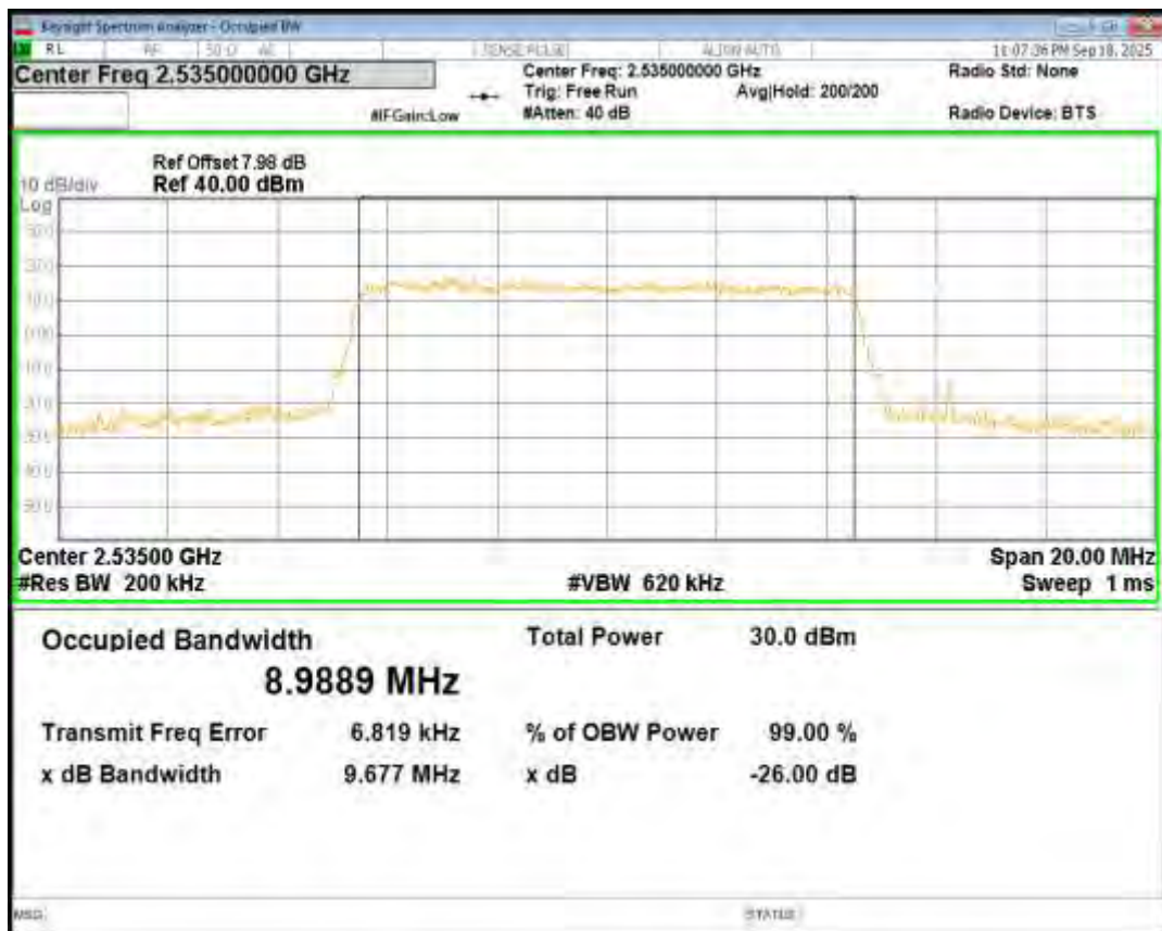
Band7 16QAM BW=5MHz Channel=21425 RB Size=25 Position=#0
