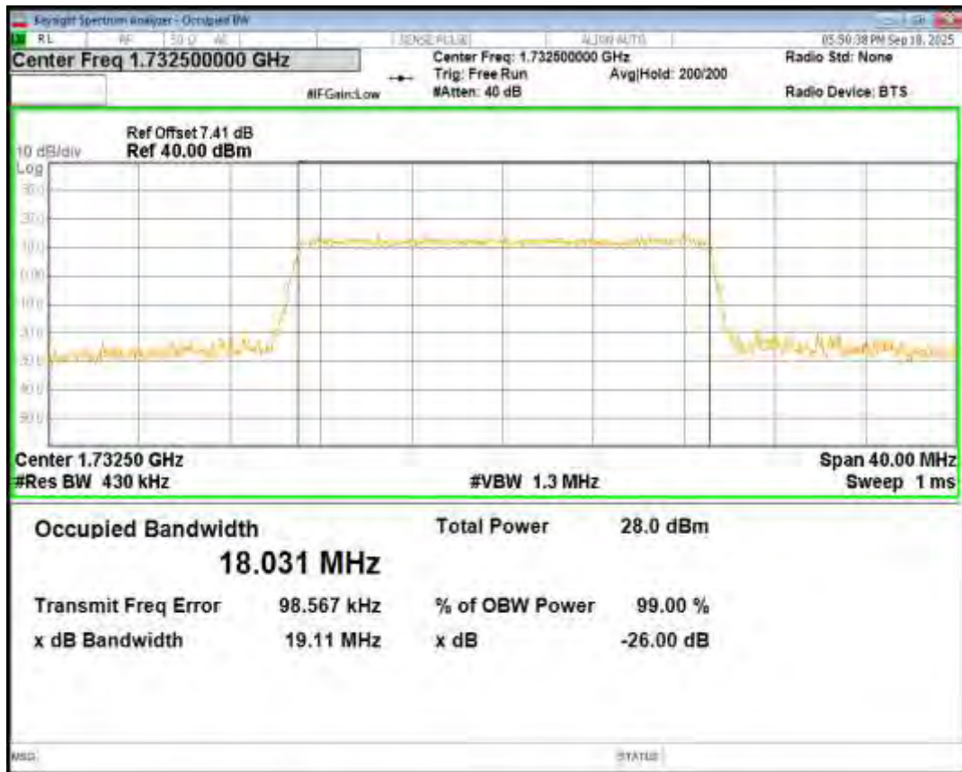
Band4 16QAM BW=15MHz Channel=20325 RB Size=75 Position=#0
