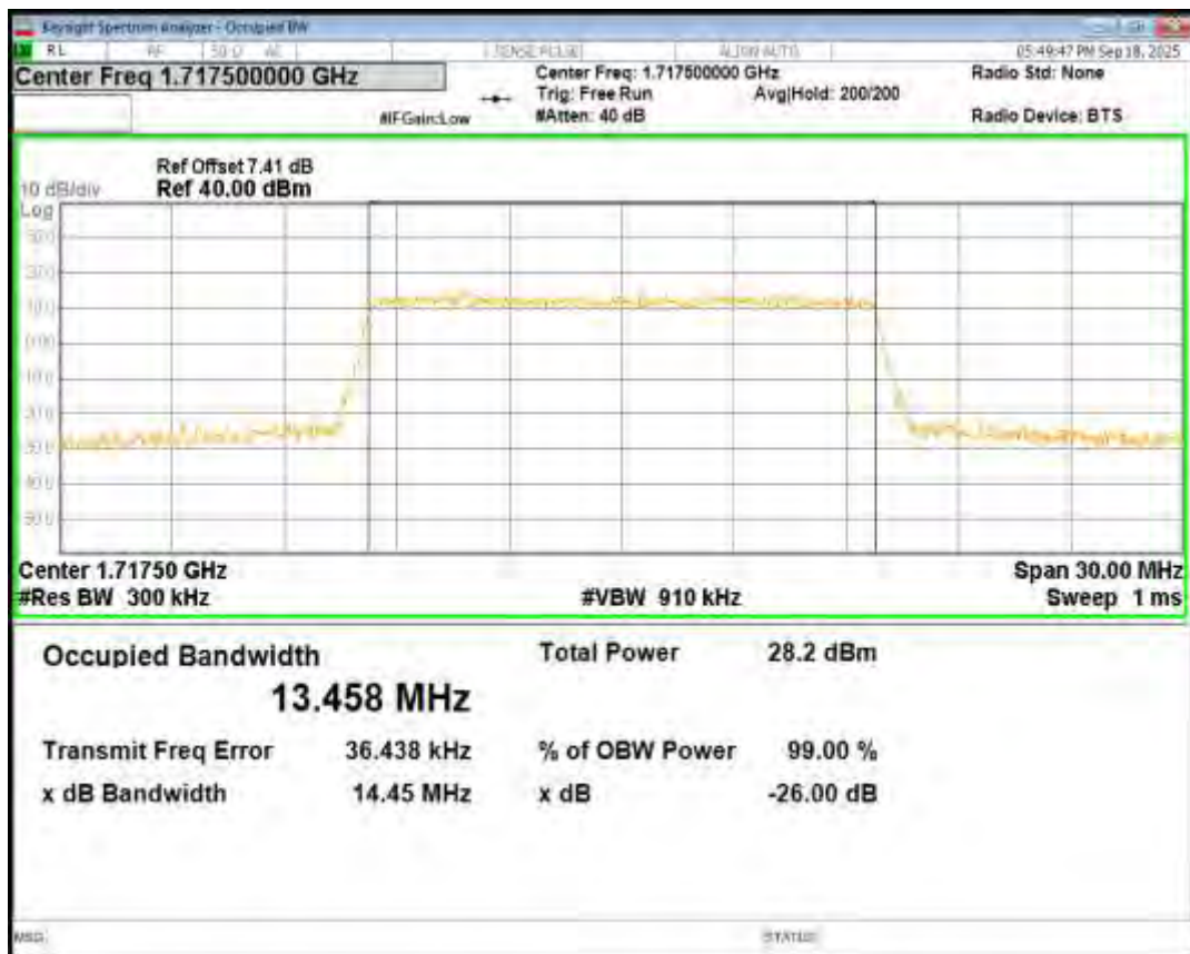
Band4 16QAM BW=15MHz Channel=20175 RB Size=75 Position=#0
