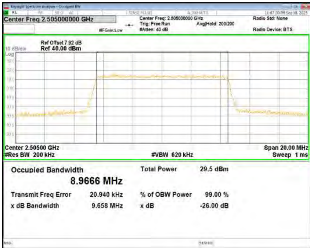
Band7 QPSK BW=15MHz Channel=20825 RB Size=75 Position=#0
