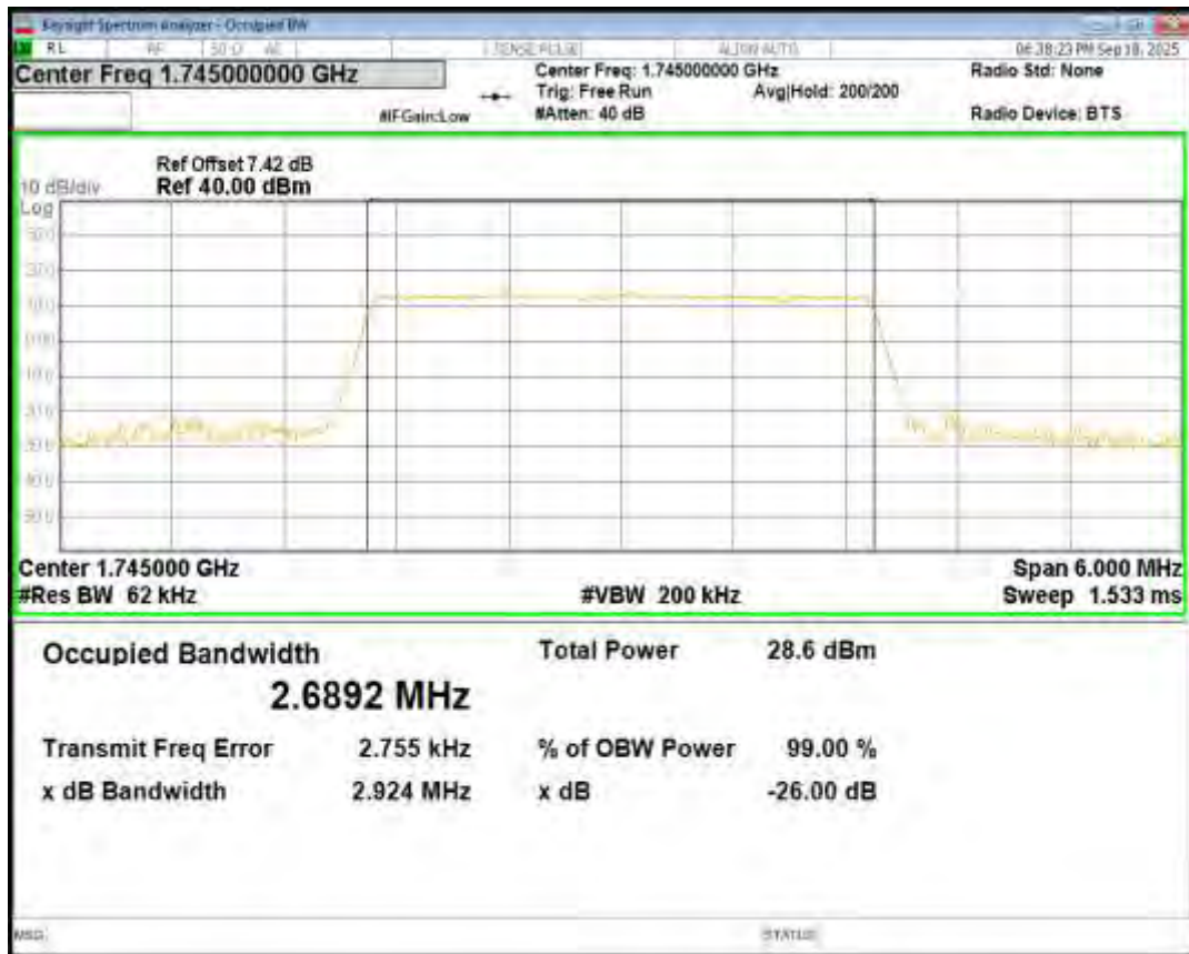
Band66 16QAM BW=3MHz Channel=132657 RB Size=15 Position=#0
