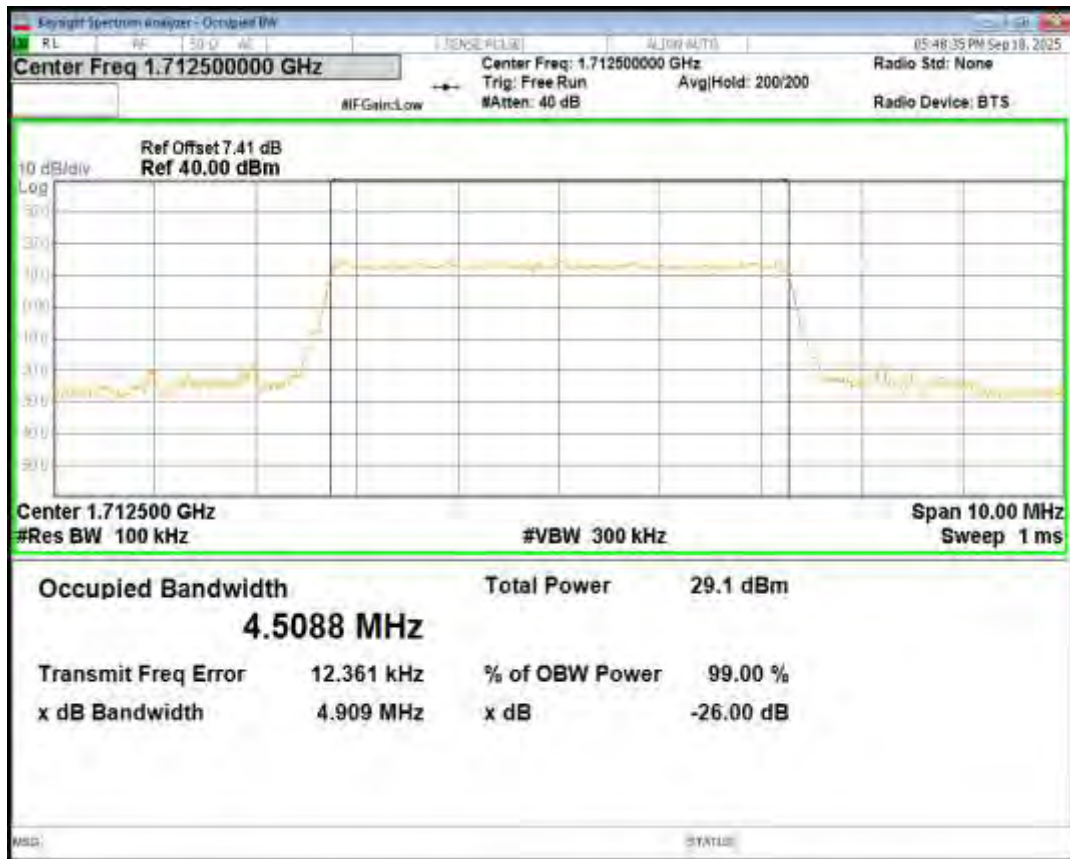
Band4 QPSK BW=5MHz Channel=20375 RB Size=25 Position=#0
