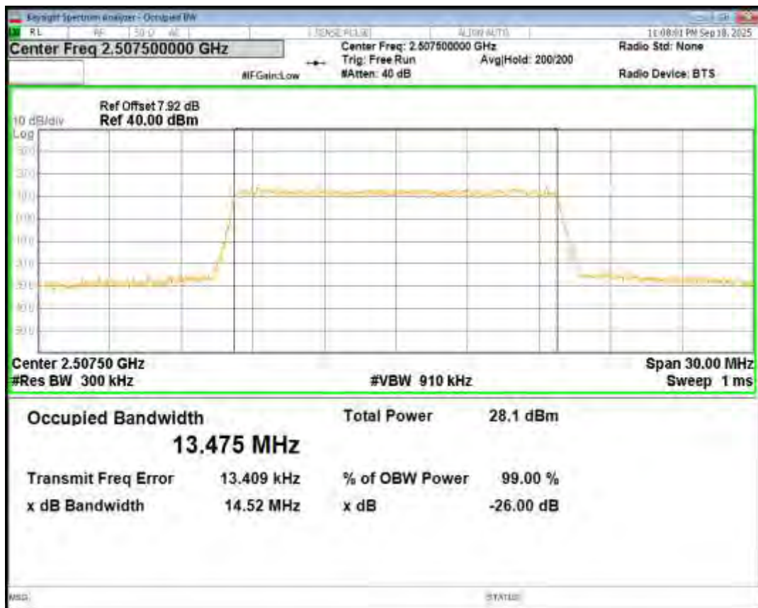
Band7 16QAM BW=15MHz Channel=21100 RB Size=75 Position=#0
