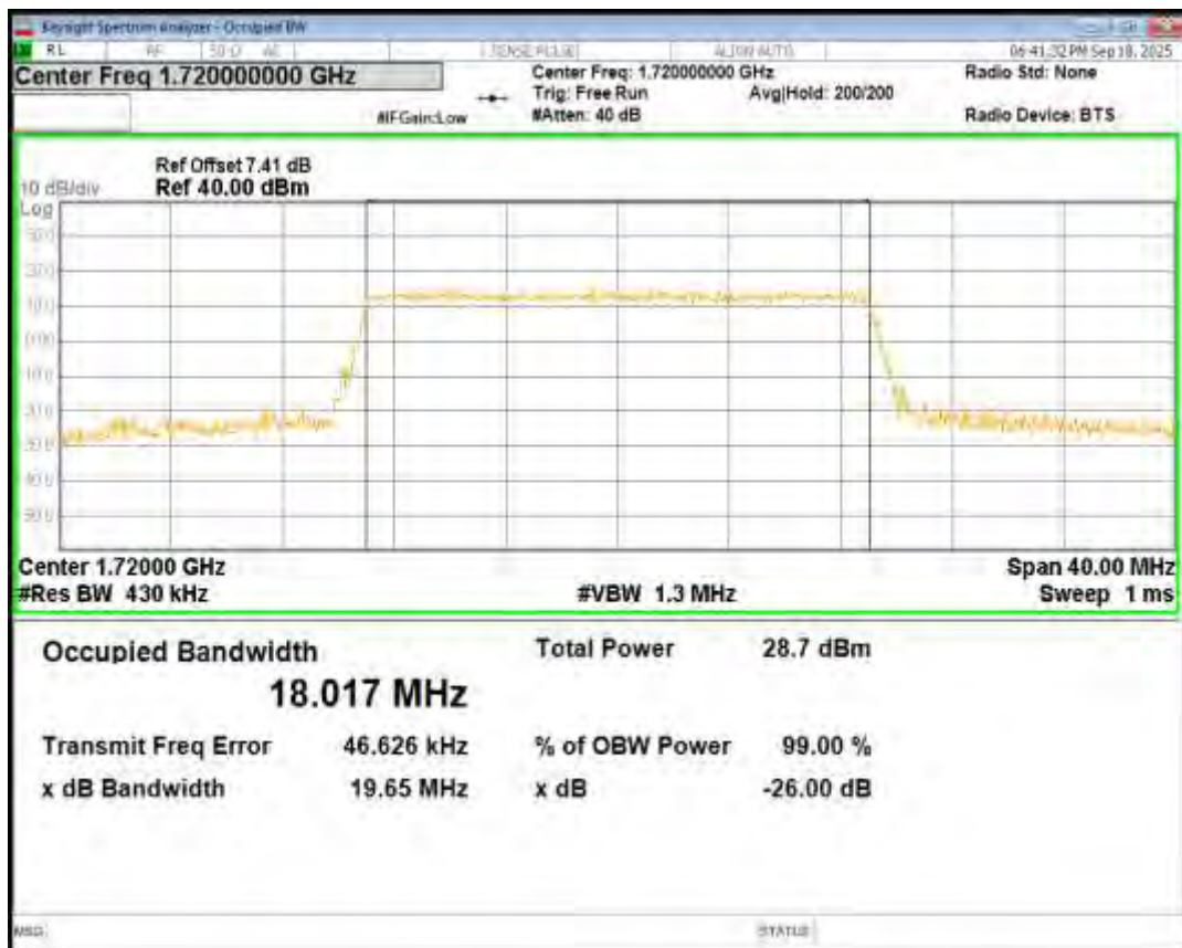
Band66 16QAM BW=5MHz Channel=132647 RB Size=25 Position=#0
