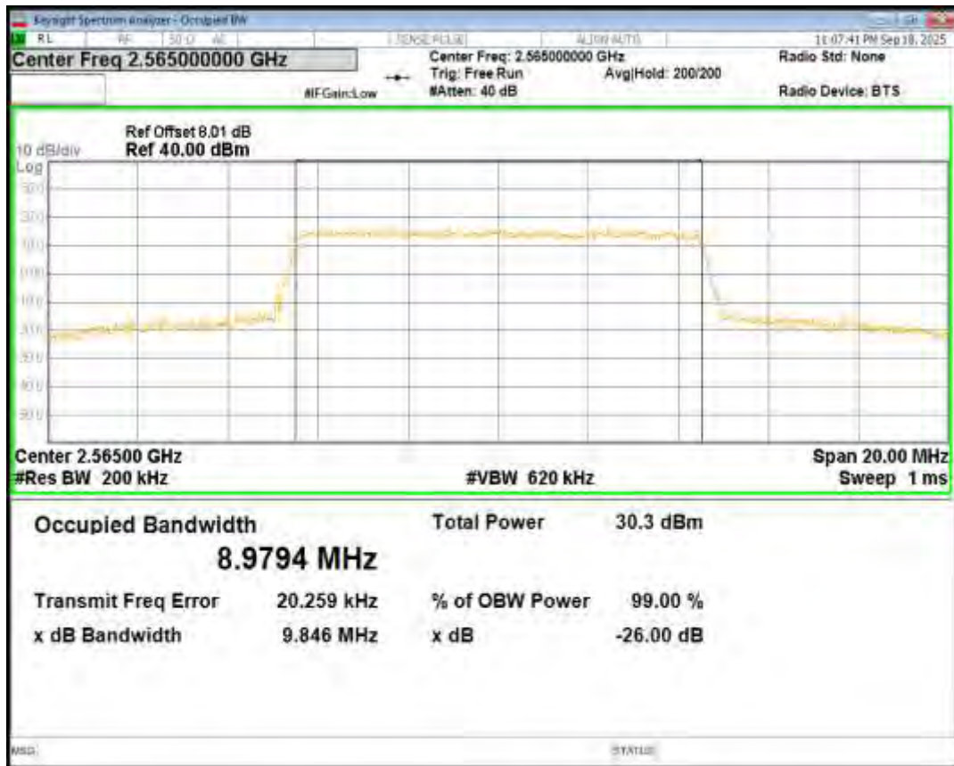
Band7 QPSK BW=10MHz Channel=21100 RB Size=50 Position=#0
