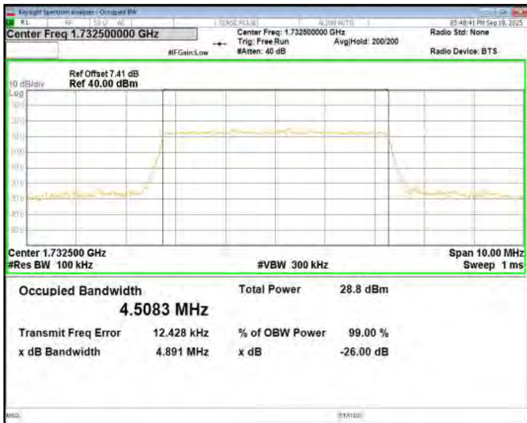
Band4 QPSK BW=20MHz Channel=20300 RB Size=100 Position=#0
