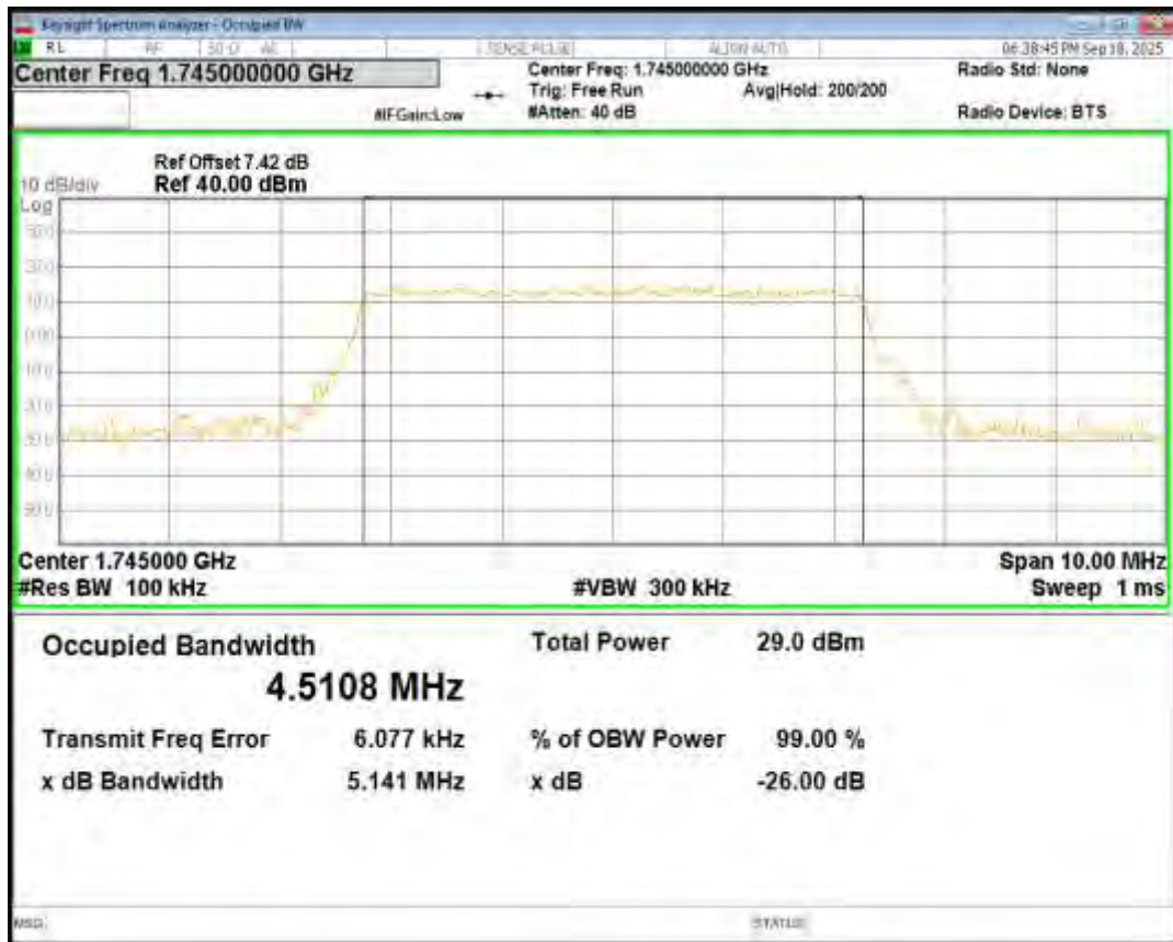
Band66 QPSK BW=5MHz Channel=132647 RB Size=25 Position=#0
