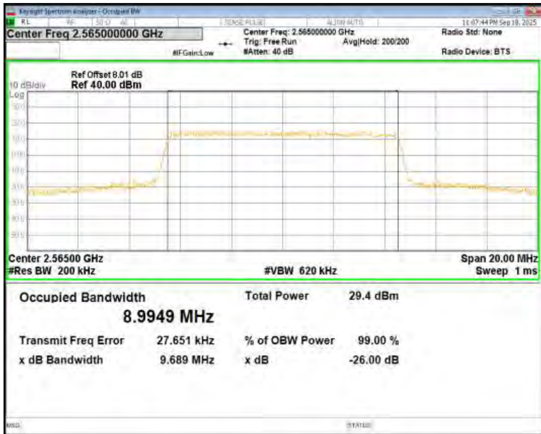
Band7 16QAM BW=15MHz Channel=20825 RB Size=75 Position=#0
