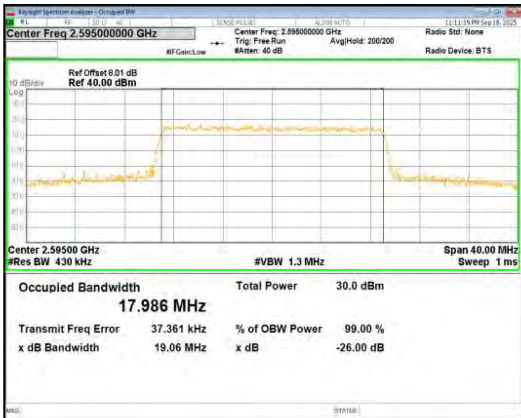
Band41(2535-2655) QPSK BW=20MHz Channel=41140 RB Size=100 Position=#0
