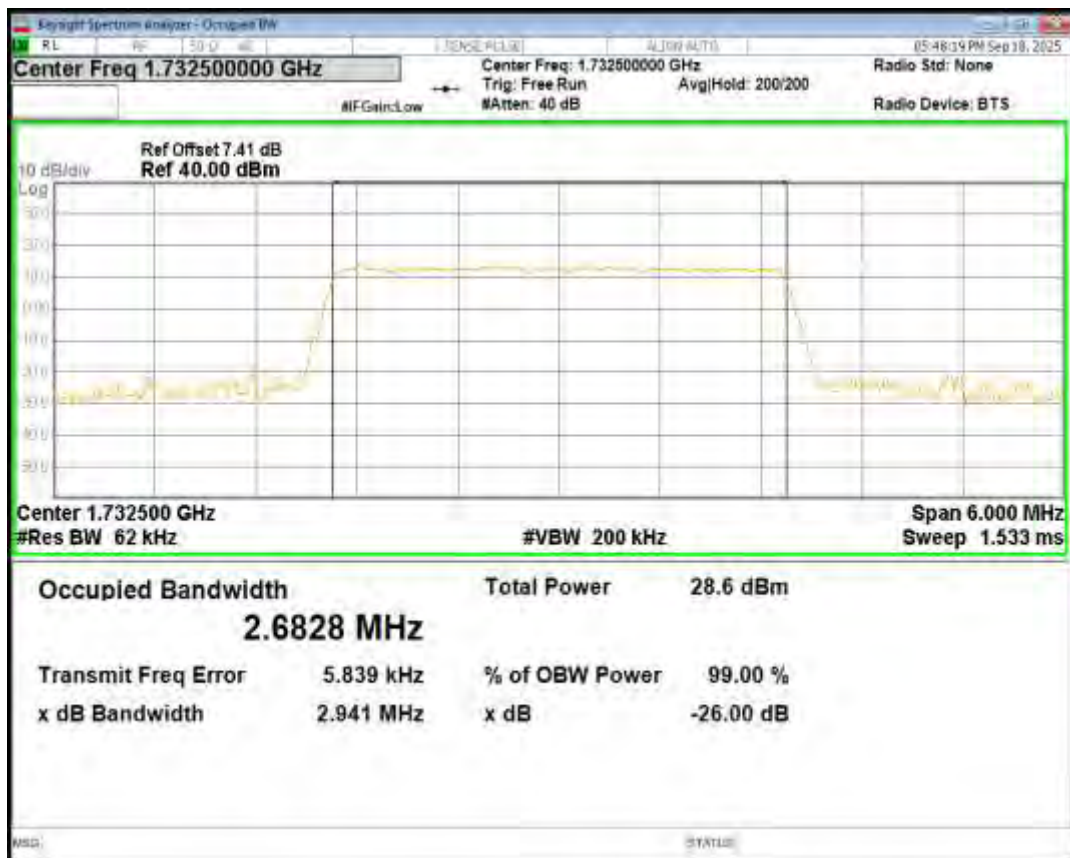
Band4 16QAM BW=3MHz Channel=20385 RB Size=15 Position=#0
