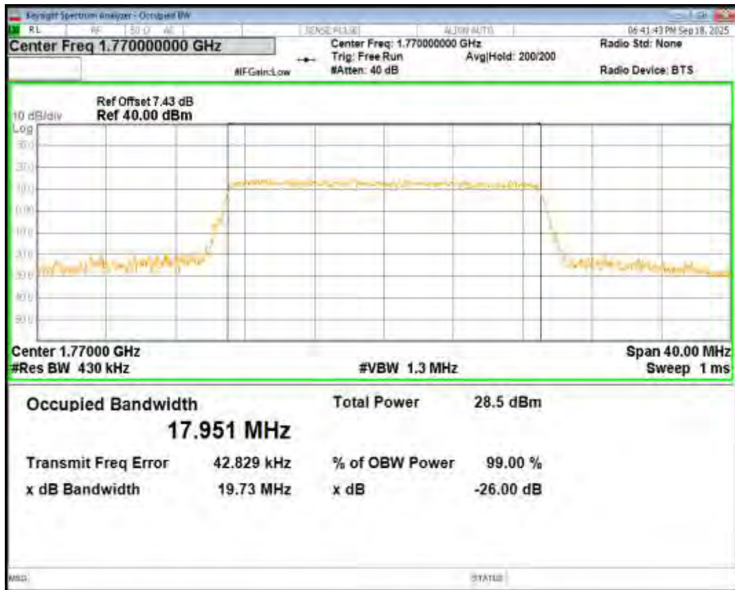
Band66 16QAM BW=20MHz Channel=132322 RB Size=100 Position=#0
