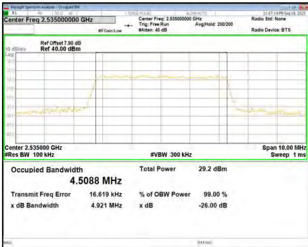
Band7 QPSK BW=10MHz Channel=20800 RB Size=50 Position=#0
