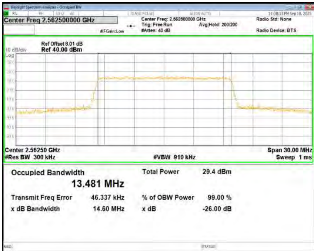
Band7 16QAM BW=20MHz Channel=20850 RB Size=100 Position=#0
