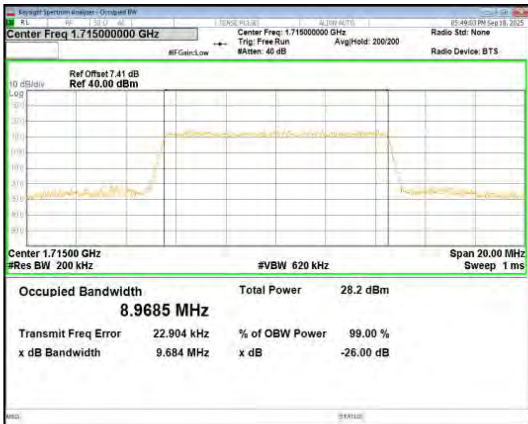
Band4 16QAM BW=10MHz Channel=20175 RB Size=50 Position=#0
