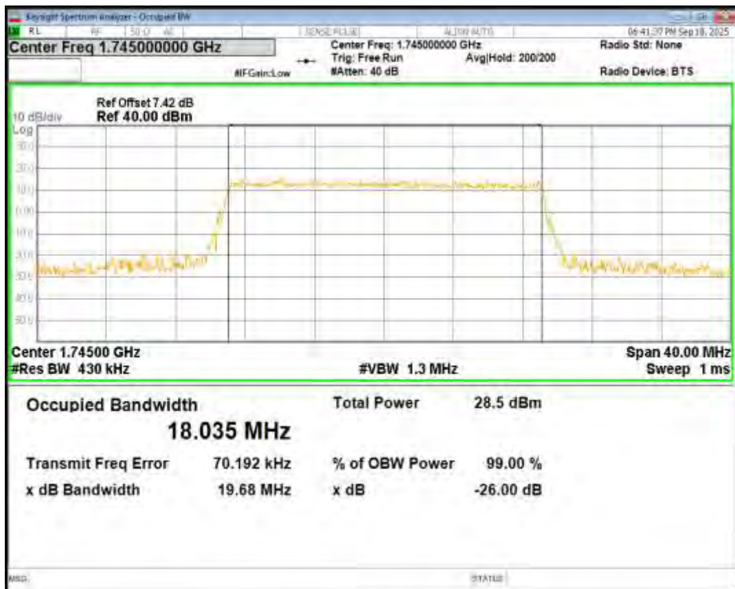
Band66 16QAM BW=15MHz Channel=132597 RB Size=75 Position=#0
