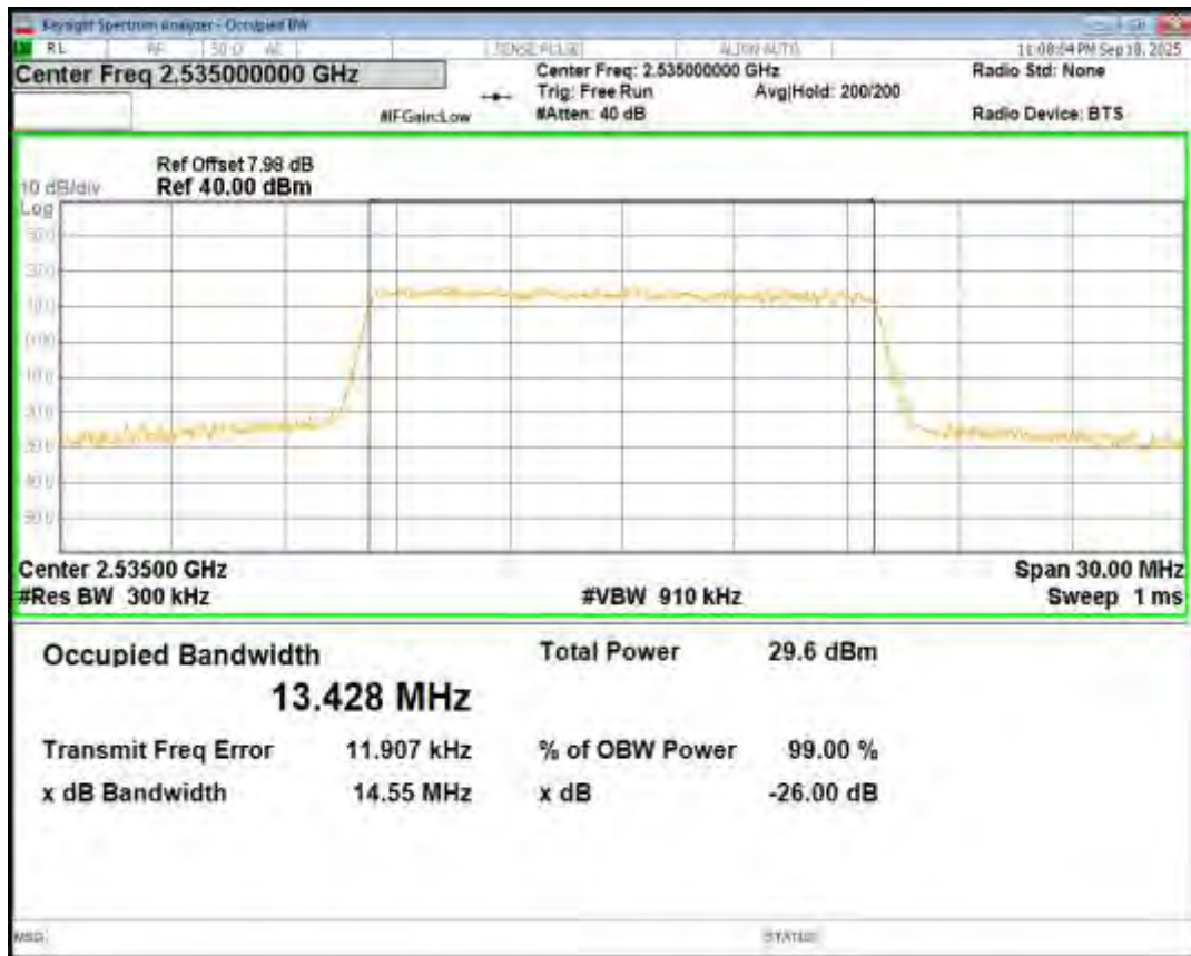
Band7 QPSK BW=15MHz Channel=21375 RB Size=75 Position=#0
