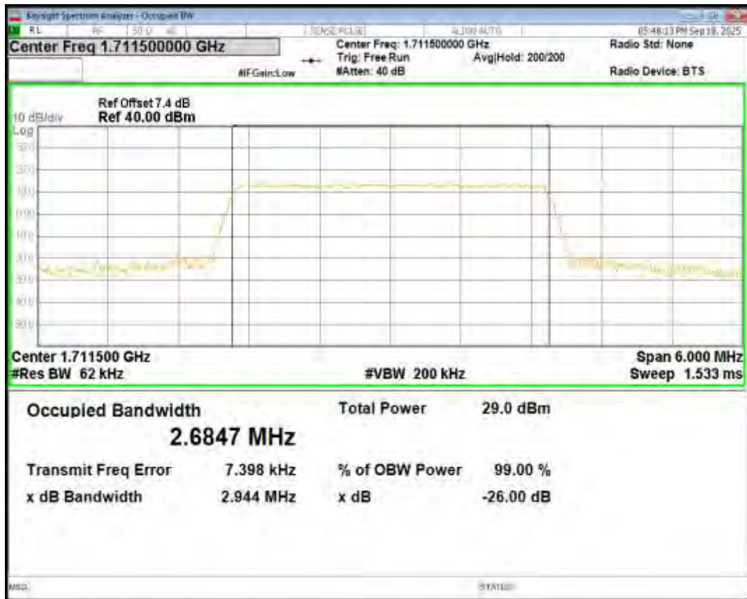
Band4 16QAM BW=3MHz Channel=20175 RB Size=15 Position=#0
