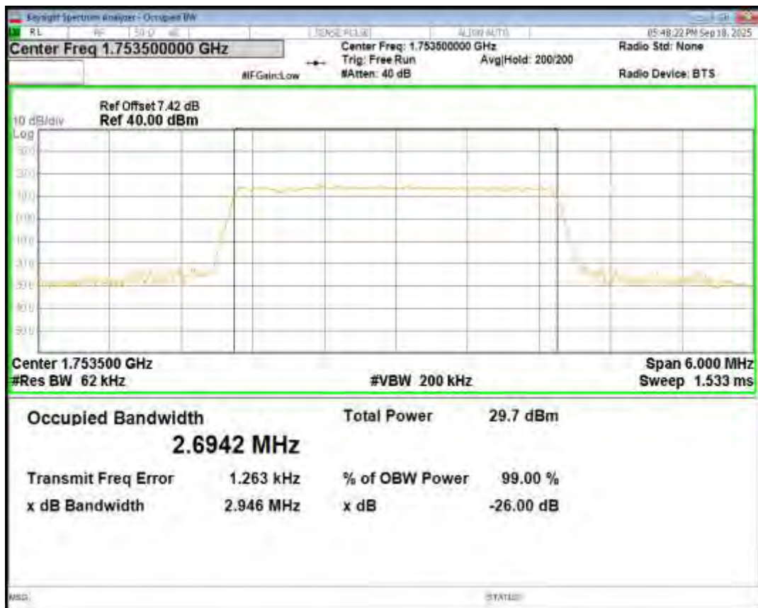
Band4 QPSK BW=5MHz Channel=19975 RB Size=25 Position=#0
