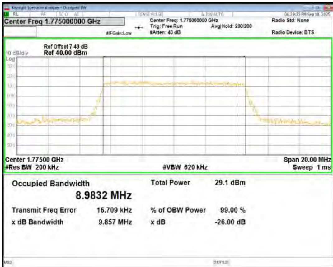
Band66 QPSK BW=15MHz Channel=132047 RB Size=75 Position=#0
