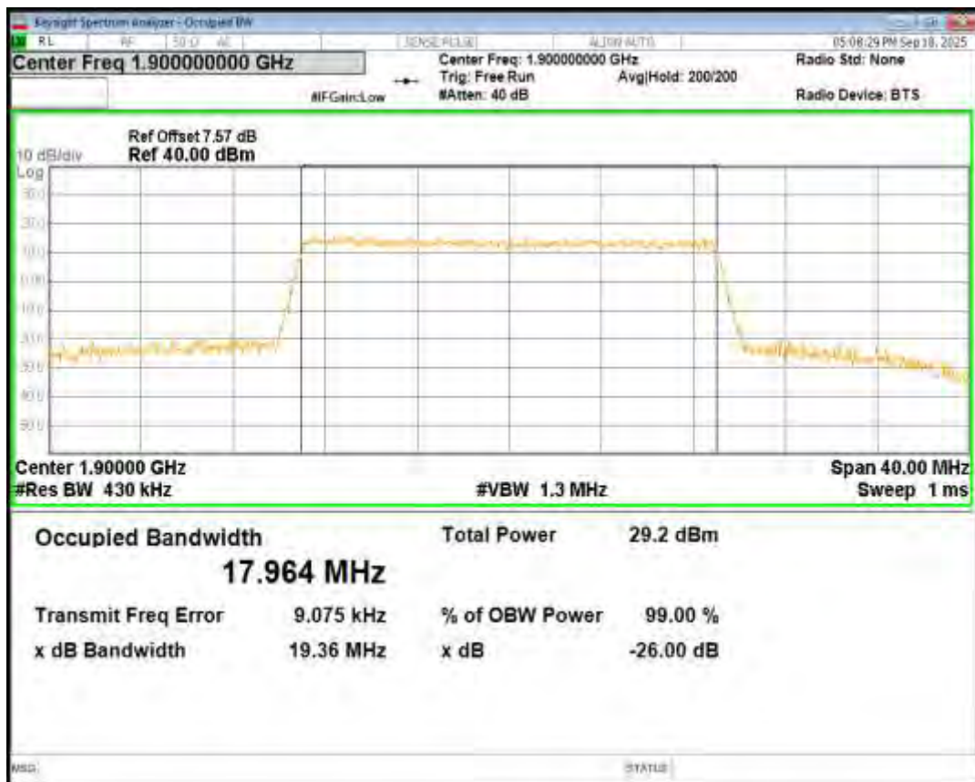
Band2 QPSK BW=3MHz Channel=18615 RB Size=15 Position=#0
