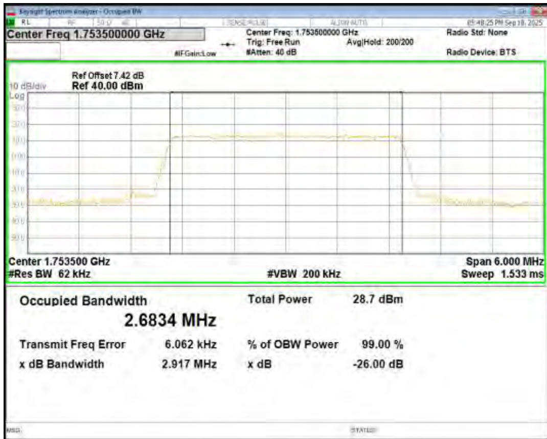
Band4 16QAM BW=5MHz Channel=19975 RB Size=25 Position=#0
