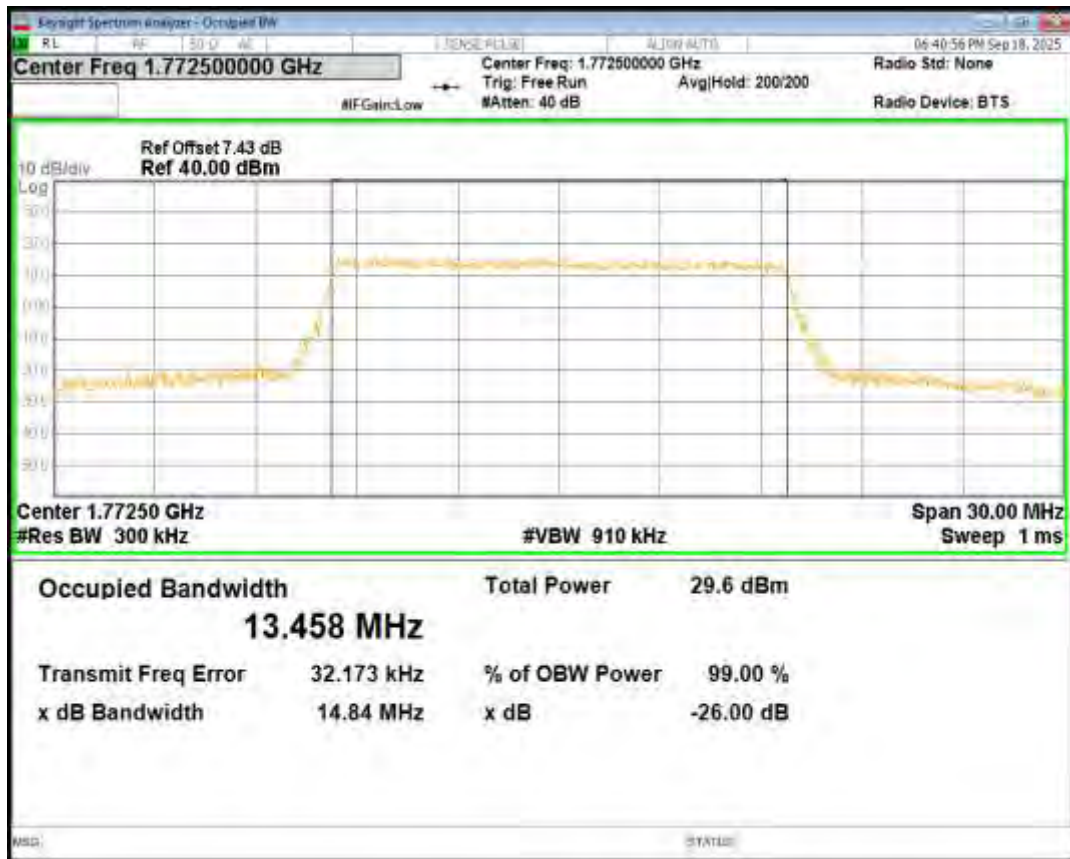
Band66 QPSK BW=20MHz Channel=132072 RB Size=100 Position=#0
