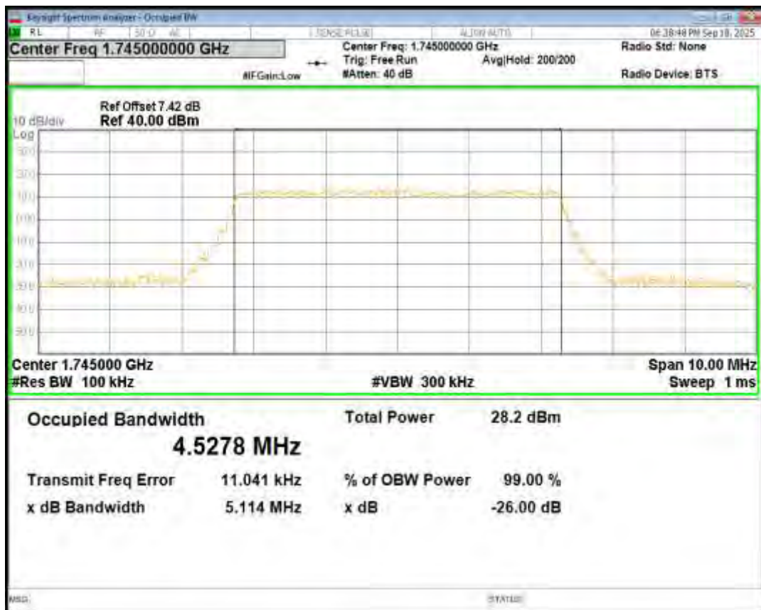
Band66 QPSK BW=1.4MHz Channel=132322 RB Size=6 Position=#0
