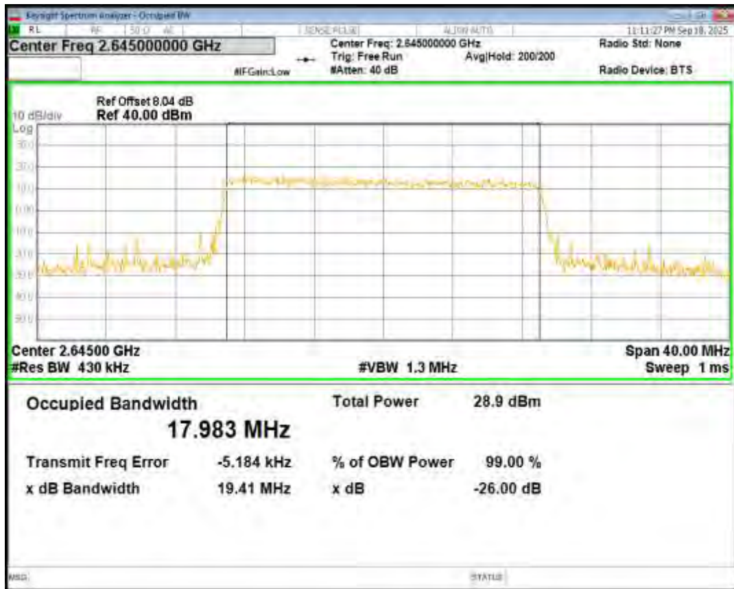
Band41(2535-2655) 16QAM BW=5MHz Channel=40065 RB Size=25 Position=#0
