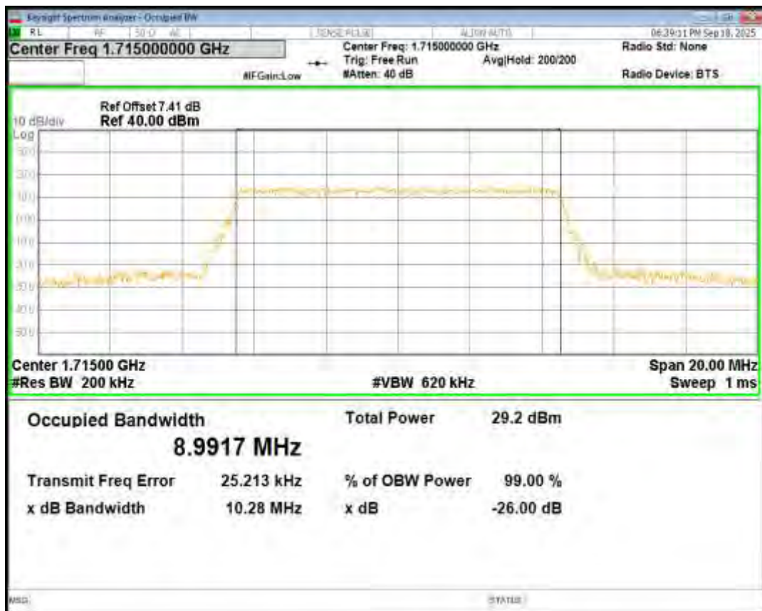
Band66 QPSK BW=10MHz Channel=132322 RB Size=50 Position=#0
