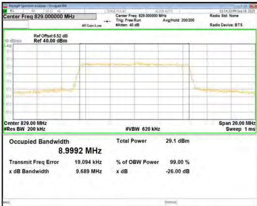
Band5 16QAM BW=10MHz Channel=20525 RB Size=50 Position=#0
