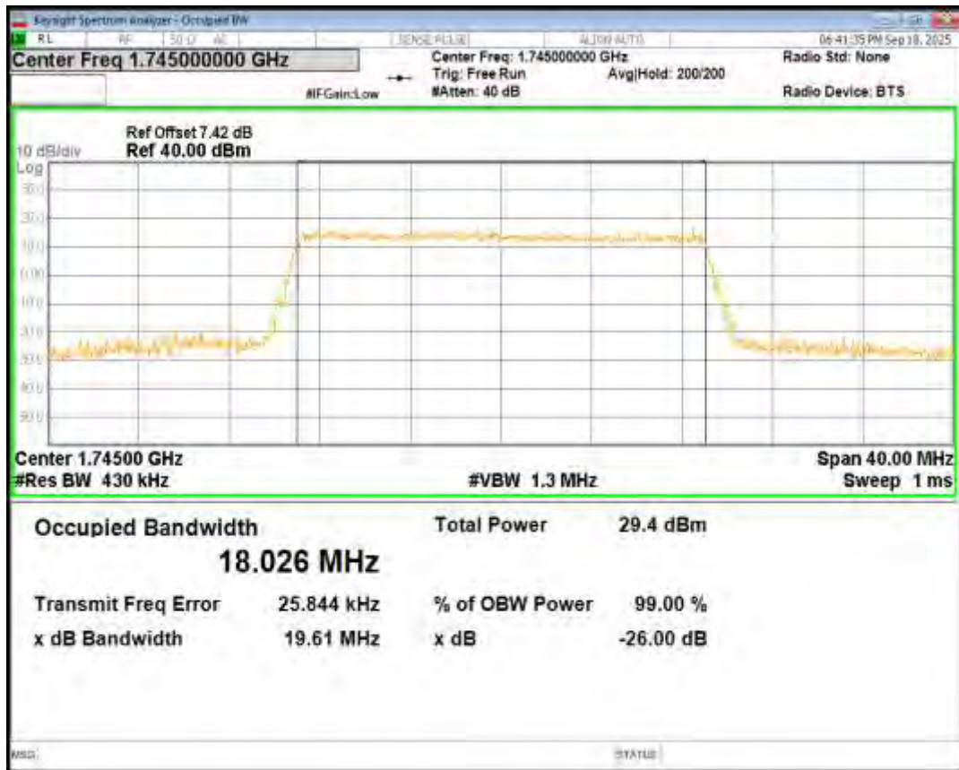
Band66 QPSK BW=20MHz Channel=132572 RB Size=100 Position=#0
