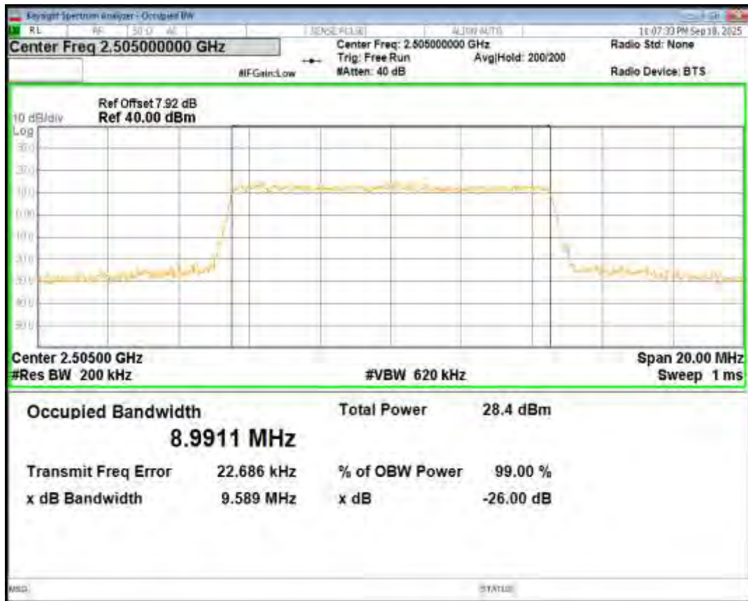
Band7 16QAM BW=10MHz Channel=21100 RB Size=50 Position=#0
