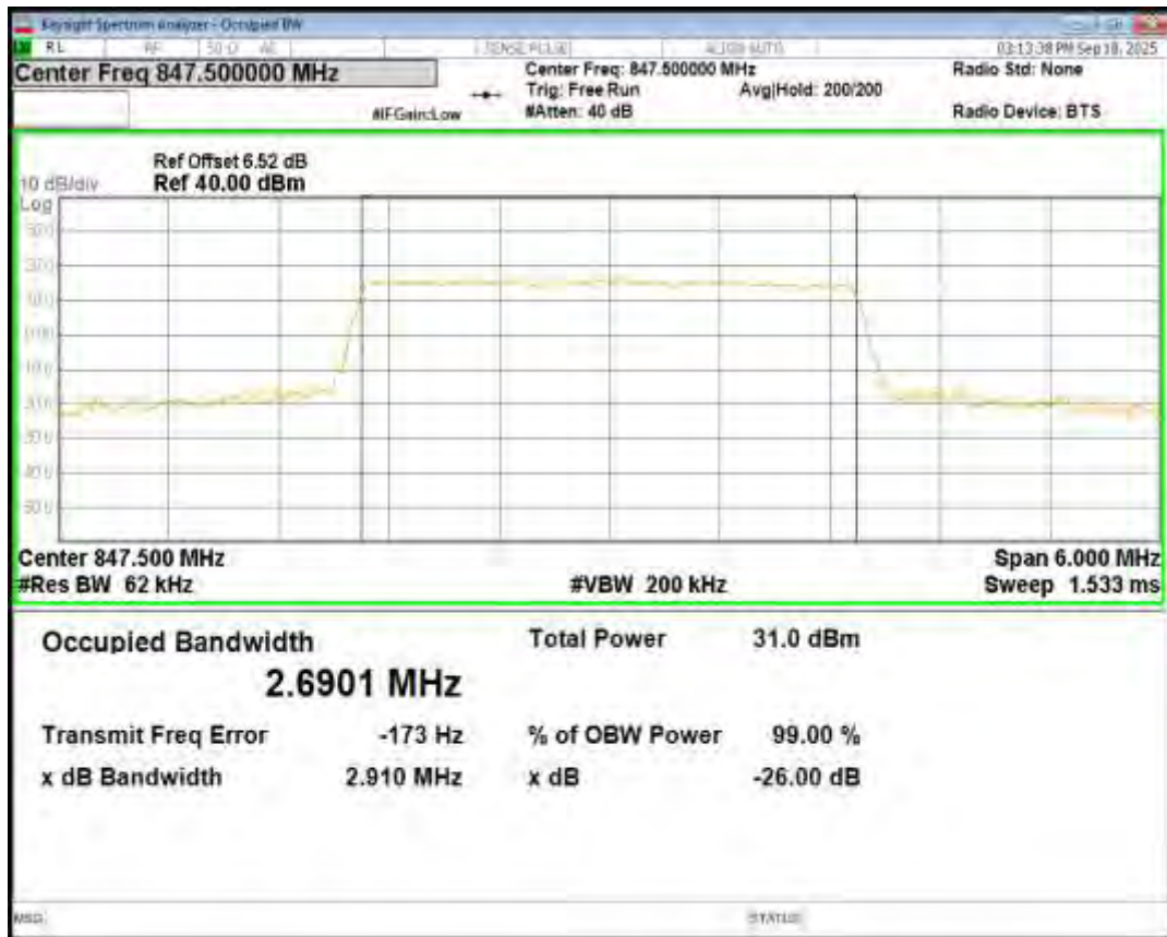
Band5 QPSK BW=5MHz Channel=20425 RB Size=25 Position=#0
