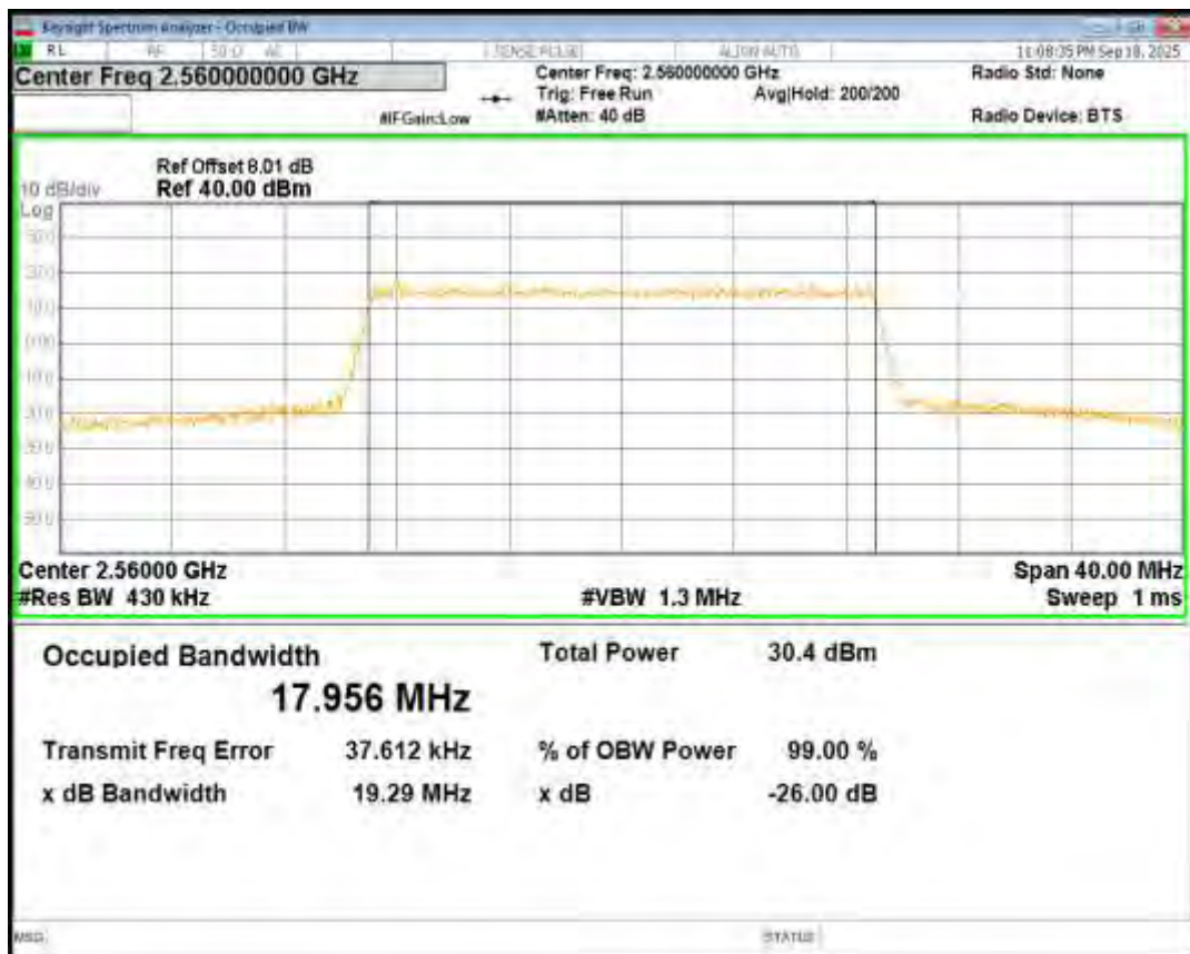
Band7 QPSK BW=5MHz Channel=20775 RB Size=25 Position=#0
