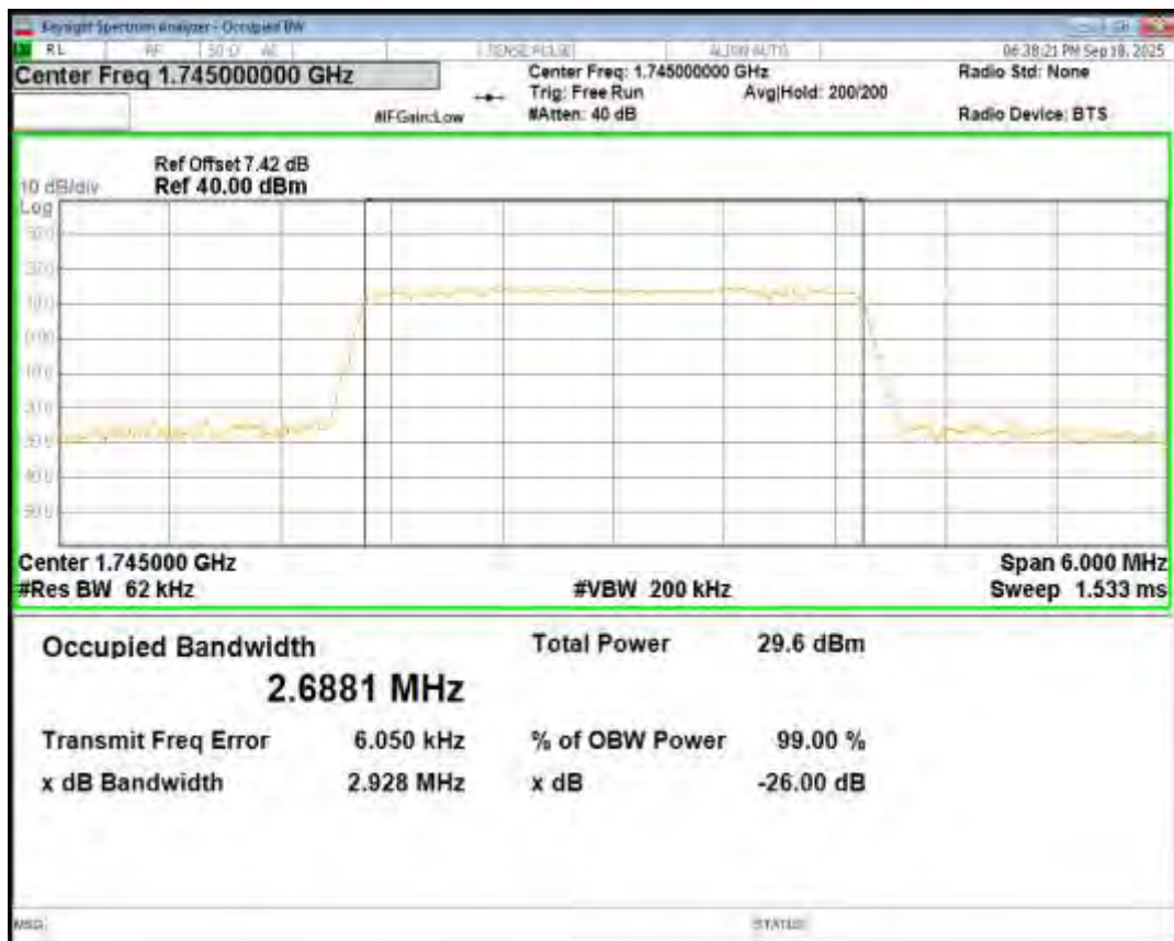
Band66 QPSK BW=3MHz Channel=132657 RB Size=15 Position=#0
