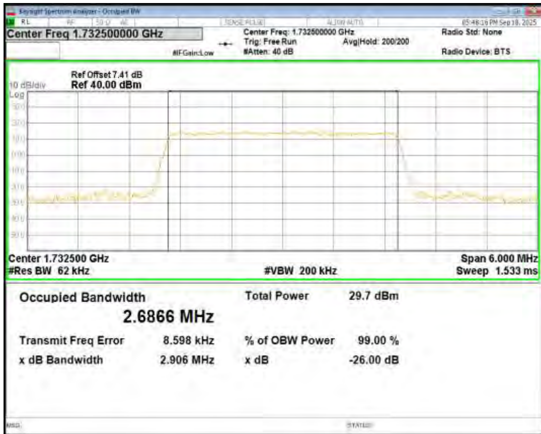
Band4 QPSK BW=3MHz Channel=20385 RB Size=15 Position=#0
