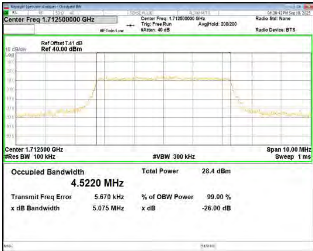
Band66 16QAM BW=5MHz Channel=132322 RB Size=25 Position=#0
