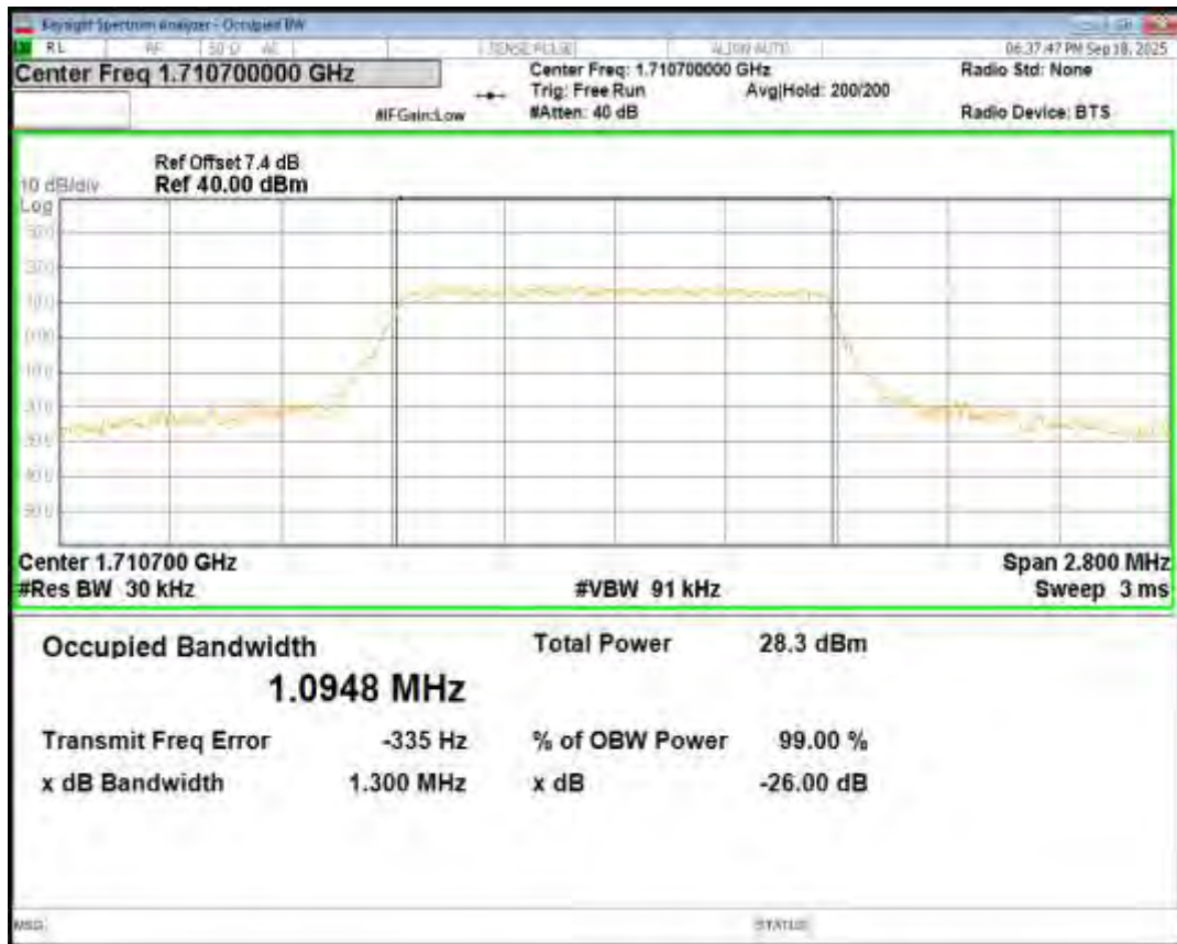
Band66 16QAM BW=1.4MHz Channel=132322 RB Size=6 Position=#0
