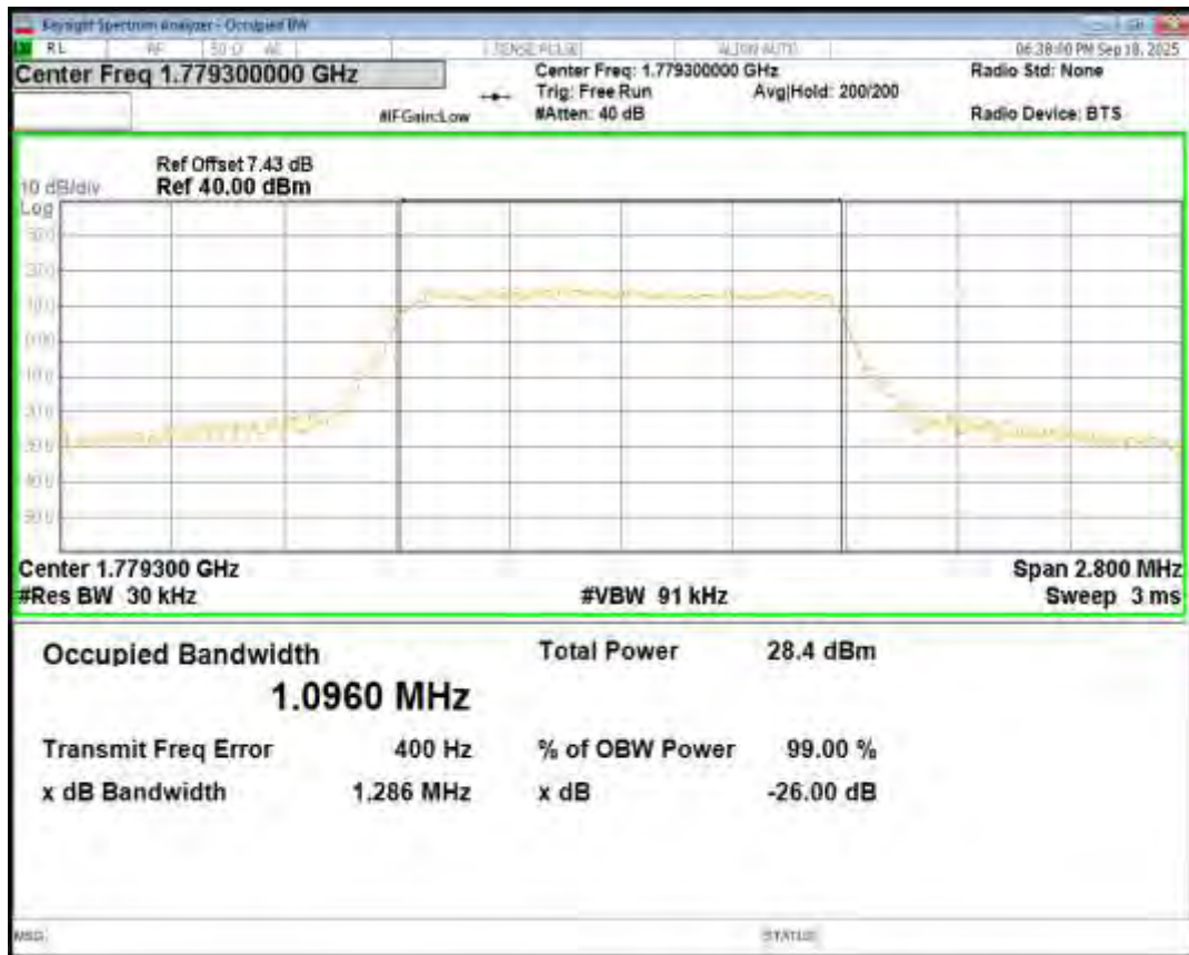
Band66 16QAM BW=10MHz Channel=132022 RB Size=50 Position=#0
