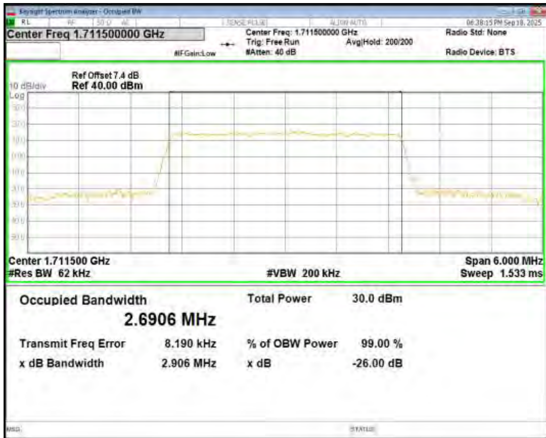
Band66 QPSK BW=3MHz Channel=132322 RB Size=15 Position=#0
