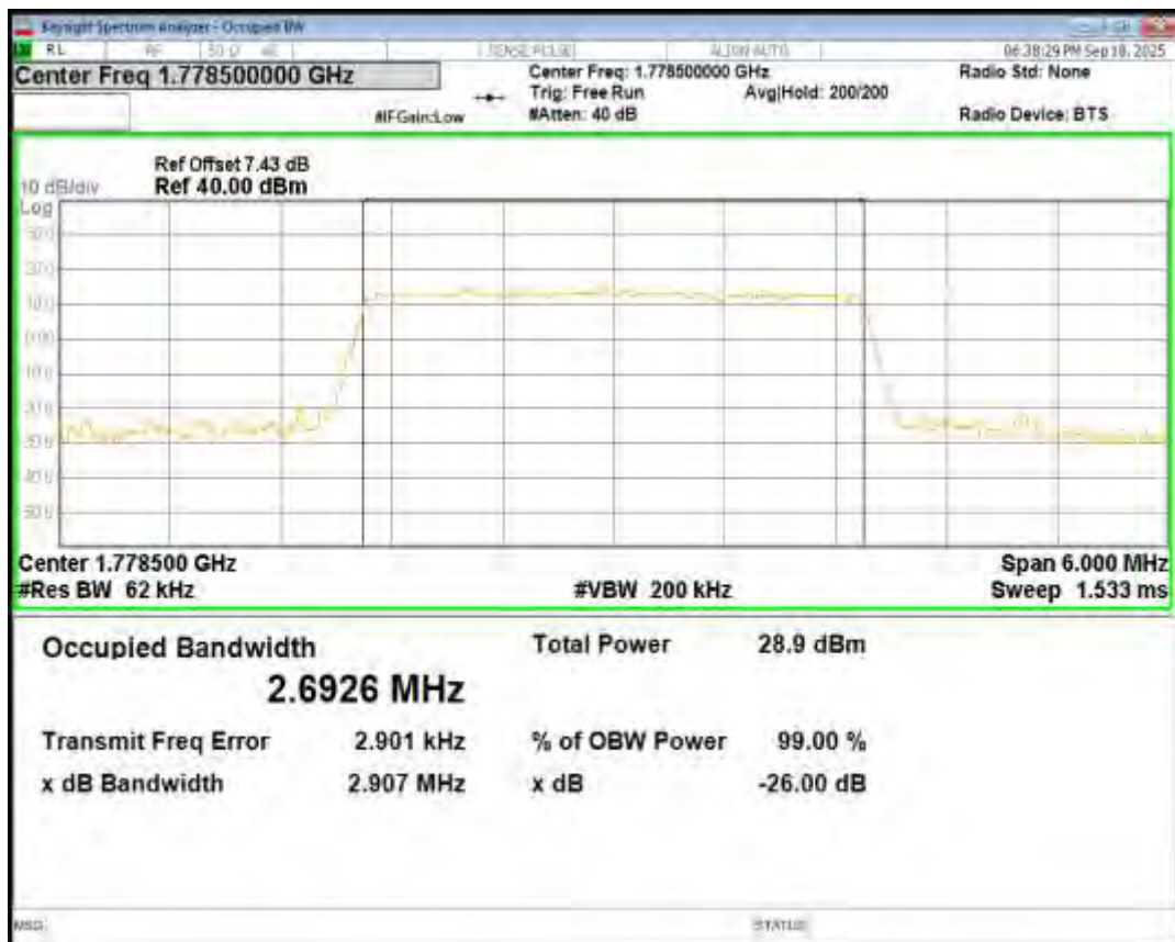
Band66 16QAM BW=5MHz Channel=131997 RB Size=25 Position=#0
