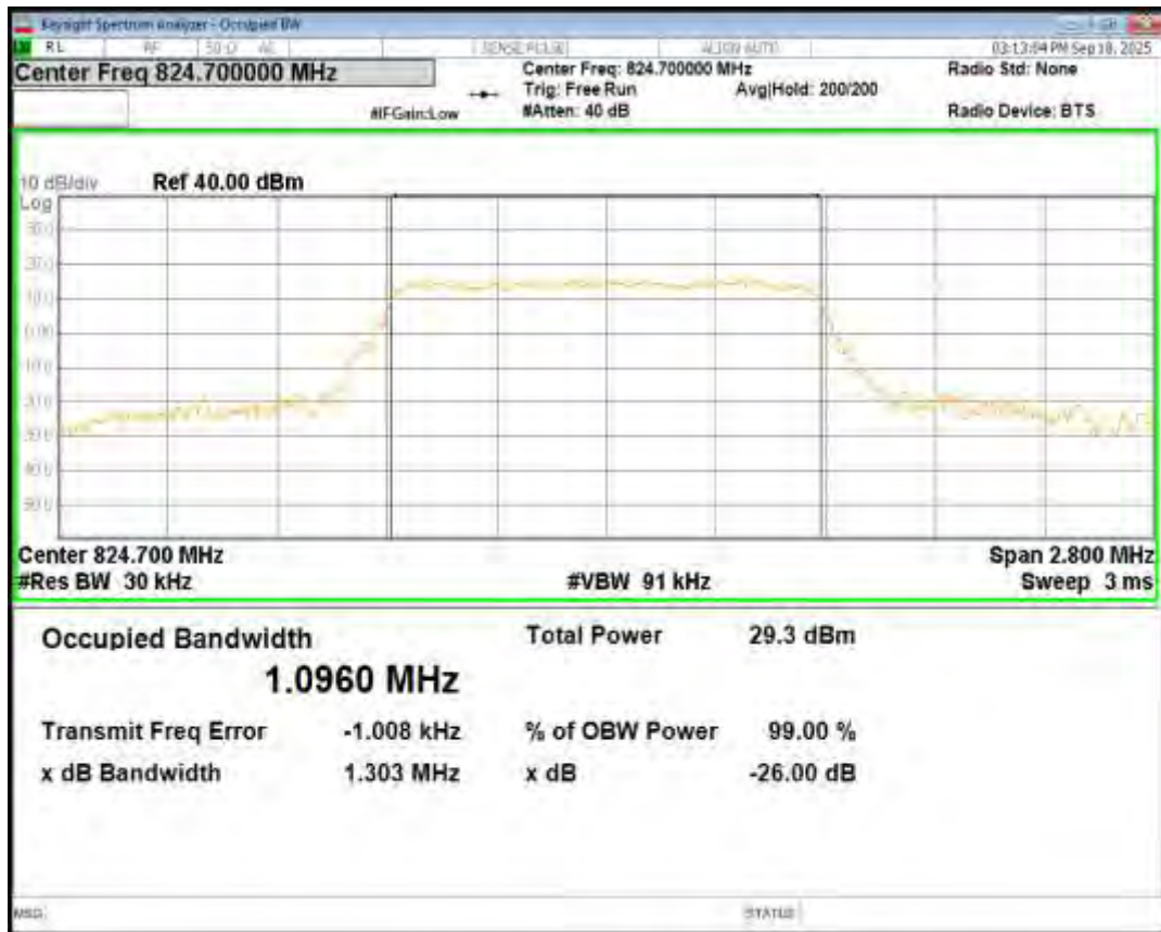
Band5 16QAM BW=1.4MHz Channel=20525 RB Size=6 Position=#0
