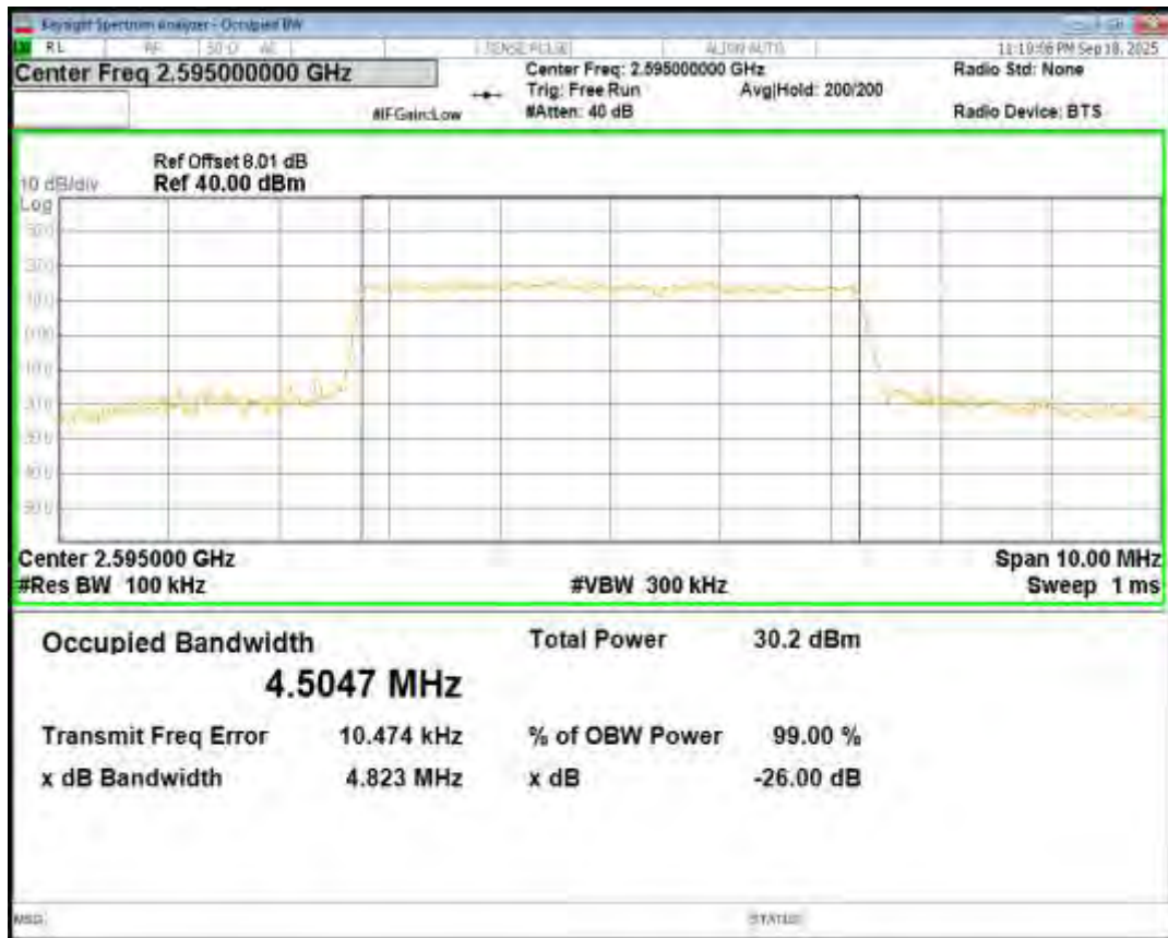
Band41(2535-2655) QPSK BW=5MHz Channel=41215 RB Size=25 Position=#0
