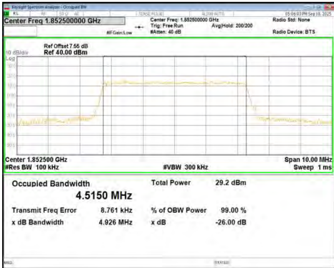
Band2 QPSK BW=5MHz Channel=19175 RB Size=25 Position=#0
