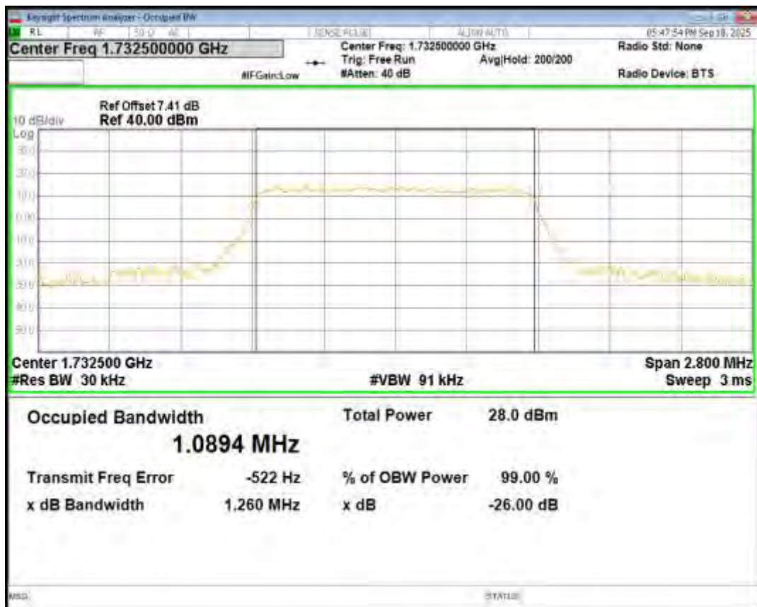
Band4 16QAM BW=1.4MHz Channel=20393 RB Size=6 Position=#0
