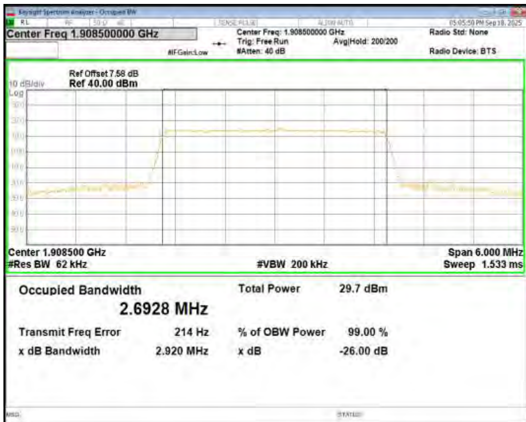
Band2 QPSK BW=5MHz Channel=18625 RB Size=25 Position=#0
