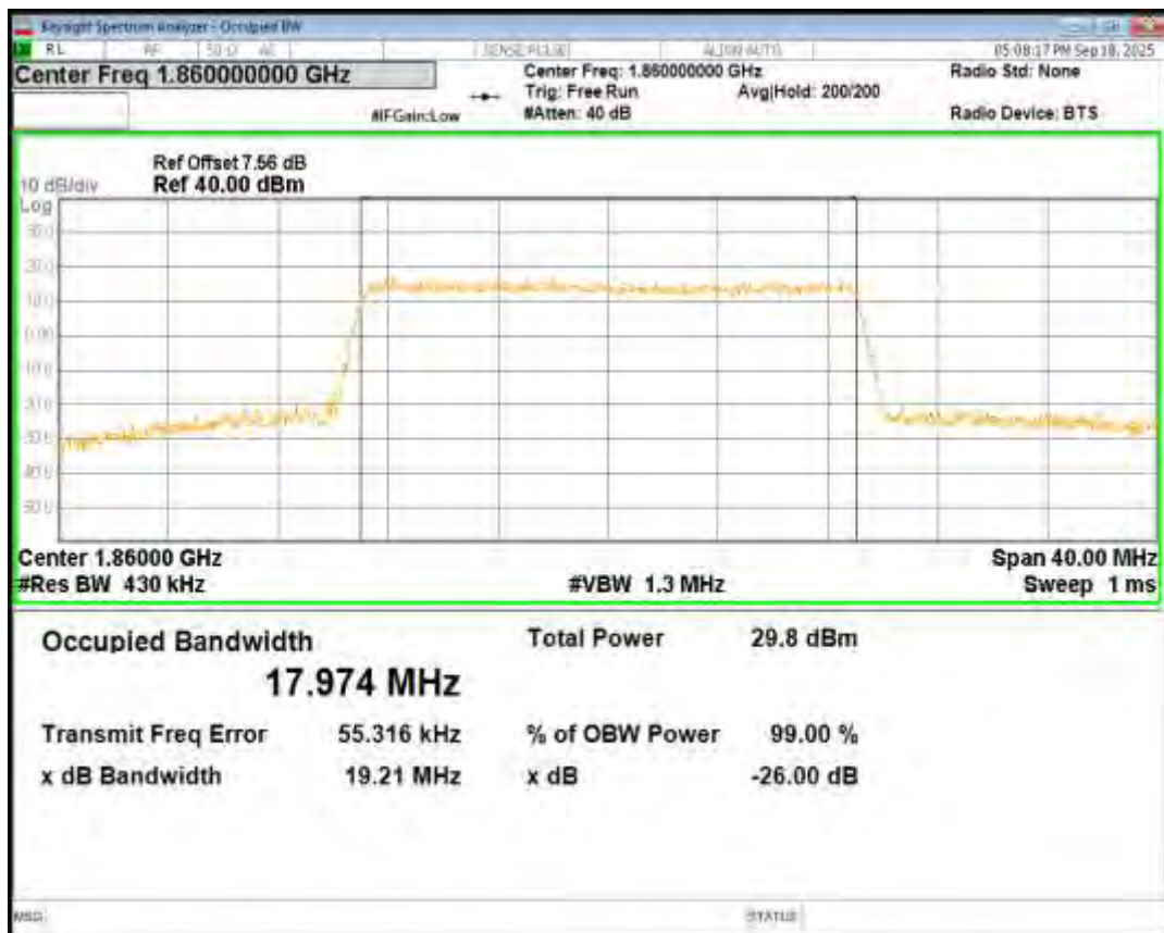
Band2 QPSK BW=20MHz Channel=18900 RB Size=100 Position=#0
