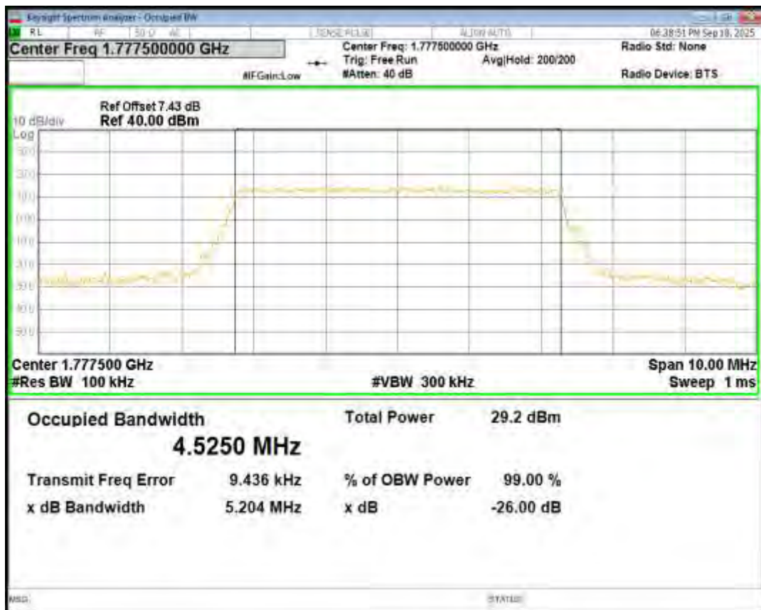
Band7 16QAM BW=10MHz Channel=20800 RB Size=50 Position=#0
