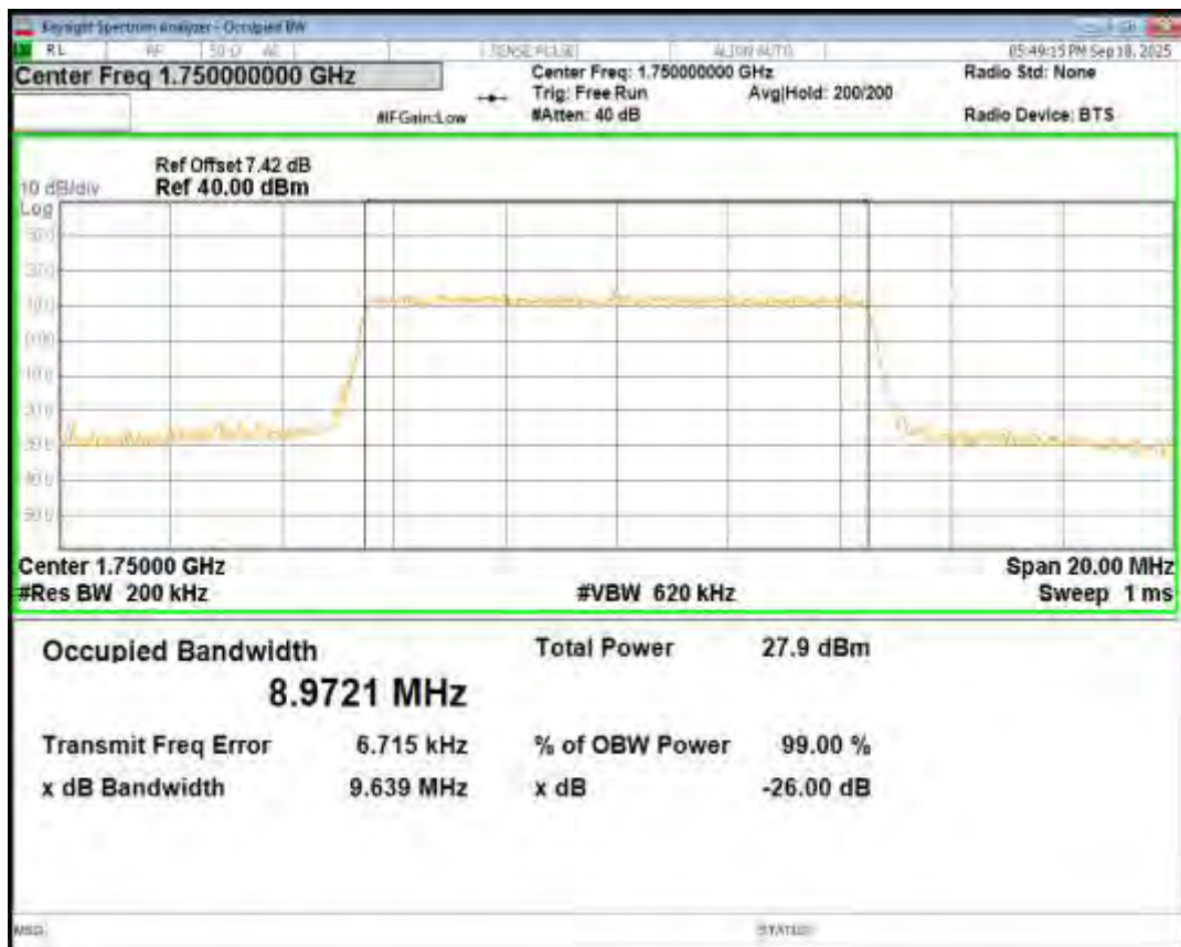
Band4 16QAM BW=20MHz Channel=20175 RB Size=100 Position=#0
