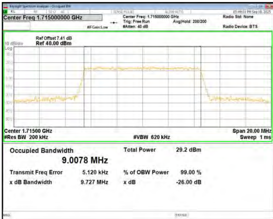
Band4 16QAM BW=5MHz Channel=20375 RB Size=25 Position=#0
