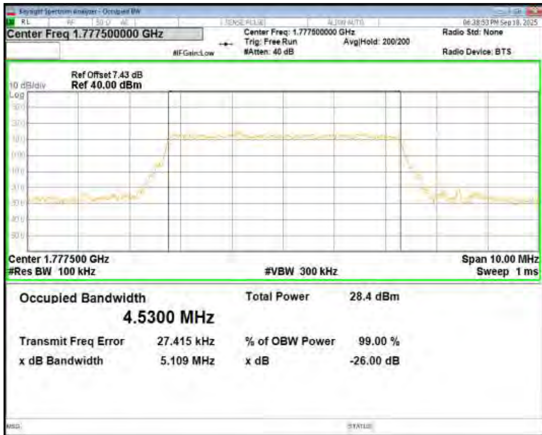
Band66 16QAM BW=3MHz Channel=131987 RB Size=15 Position=#0
