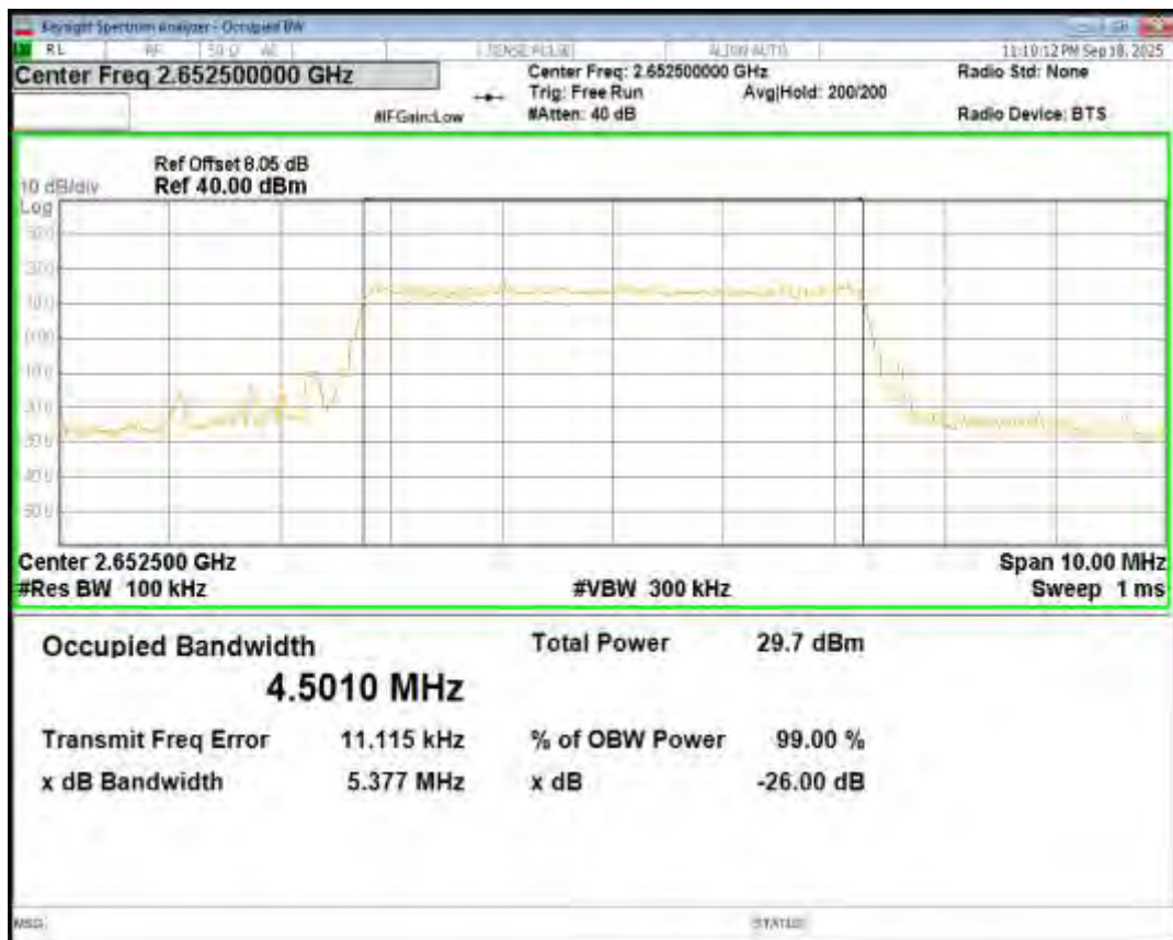
Band5 16QAM BW=1.4MHz Channel=20407 RB Size=6 Position=#0
