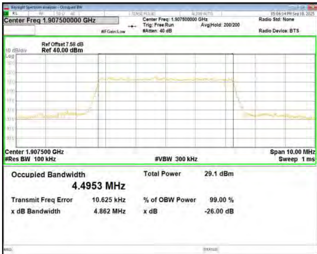
Band4 16QAM BW=1.4MHz Channel=19957 RB Size=6 Position=#0
