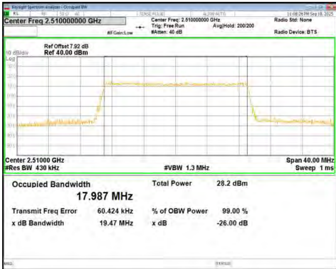
Band7 16QAM BW=20MHz Channel=21100 RB Size=100 Position=#0
