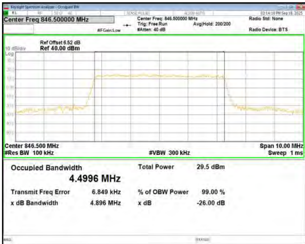
Band5 QPSK BW=1.4MHz Channel=20407 RB Size=6 Position=#0
