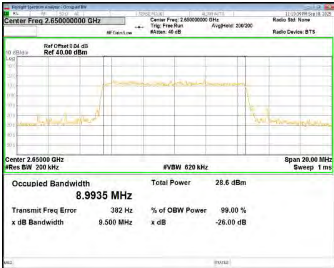
Band41(2535-2655) 16QAM BW=15MHz Channel=40115 RB Size=75 Position=#0
