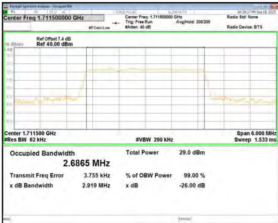
Band66 16QAM BW=3MHz Channel=132322 RB Size=15 Position=#0
