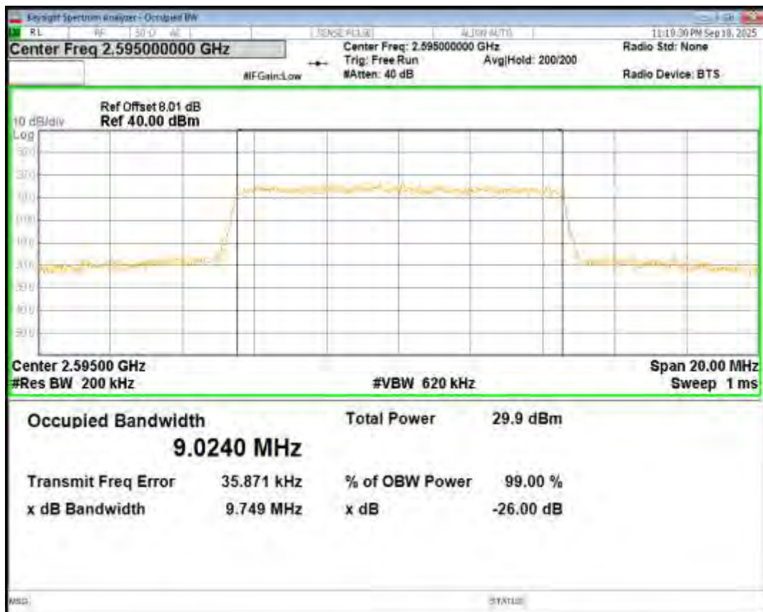
Band41(2535-2655) 16QAM BW=5MHz Channel=41215 RB Size=25 Position=#0
