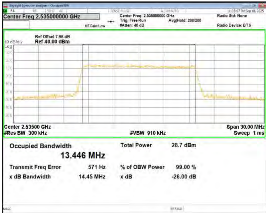
Band7 16QAM BW=15MHz Channel=21375 RB Size=75 Position=#0
