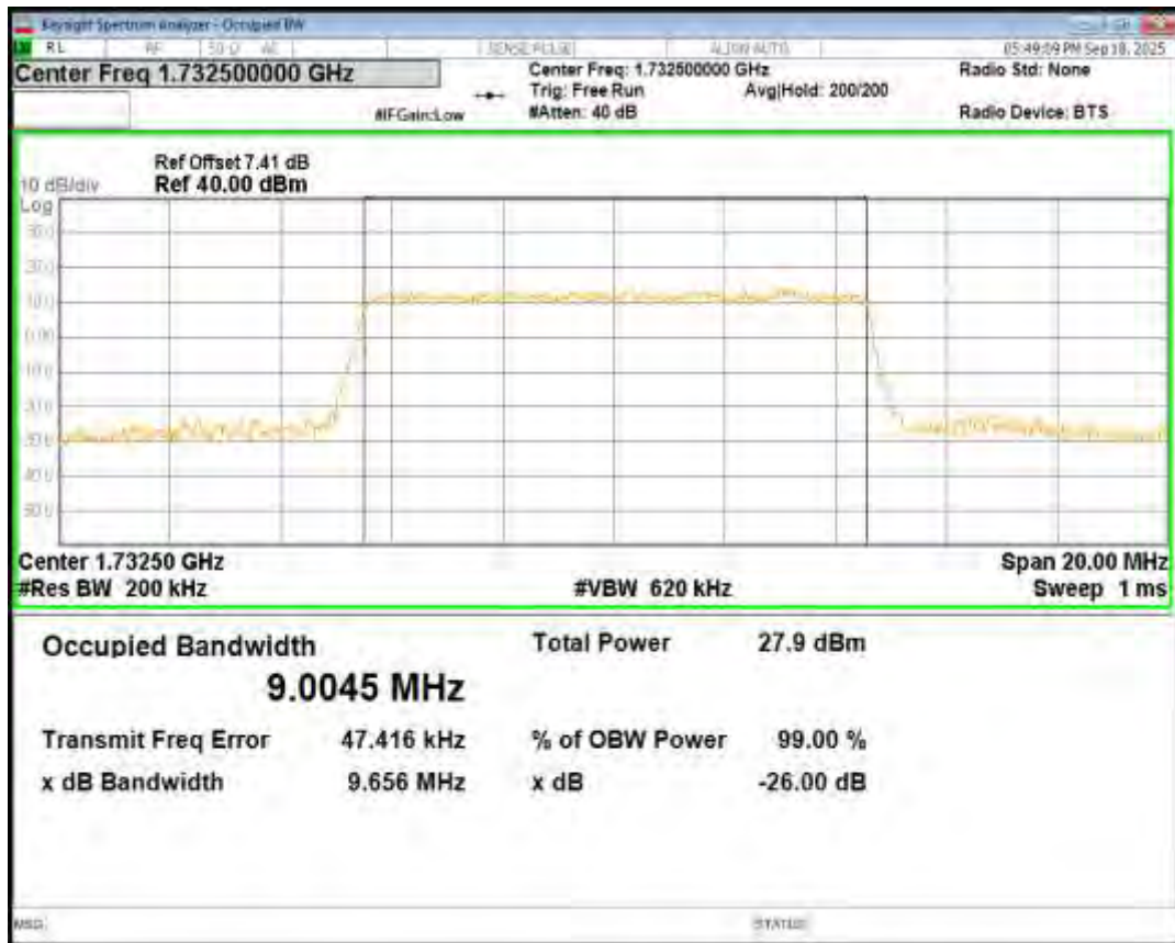
Band4 16QAM BW=10MHz Channel=20350 RB Size=50 Position=#0
