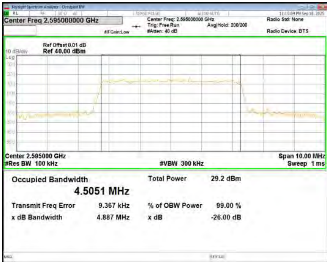
Band41(2535-2655) QPSK BW=10MHz Channel=40640 RB Size=50 Position=#0
