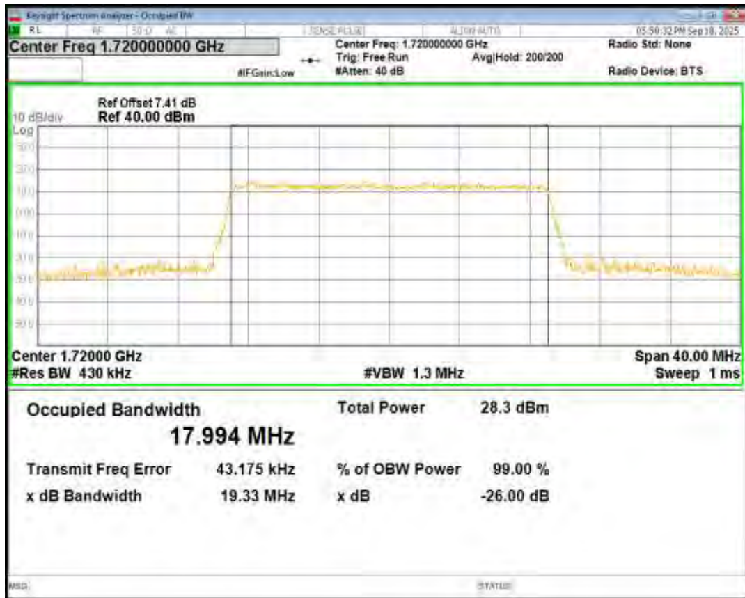
Band4 16QAM BW=15MHz Channel=20025 RB Size=75 Position=#0
