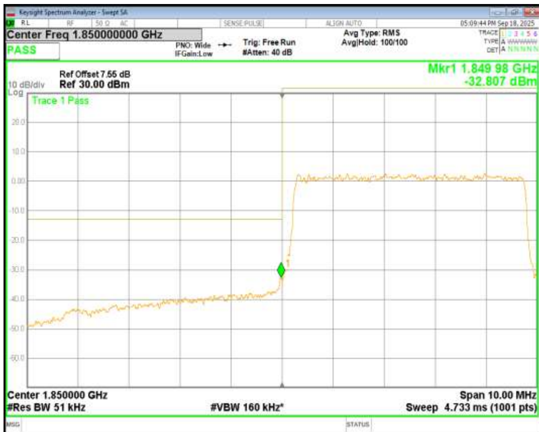
Band2 16QAM BW=5MHz Channel=19175 RB Size=25 Position=#0
