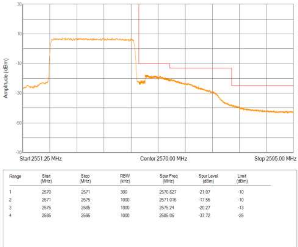
Band7 QPSK BW=20MHz Channel=20850 RB Size=100 Position=#0
