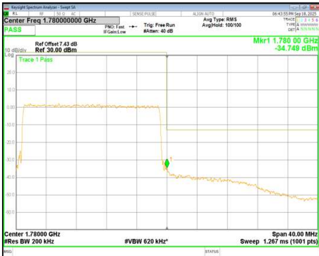
Band66 16QAM BW=3MHz Channel=131987 RB Size=15 Position=#0
