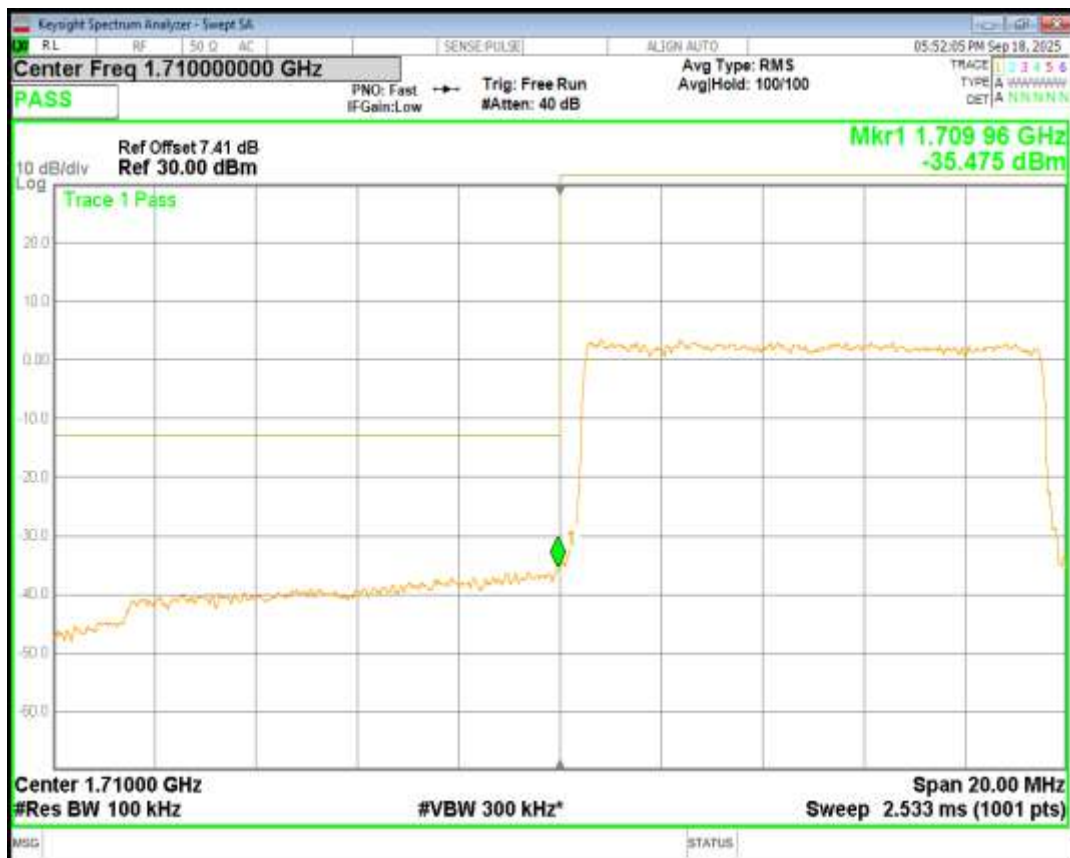
Band4 QPSK BW=10MHz Channel=20350 RB Size=50 Position=#0
