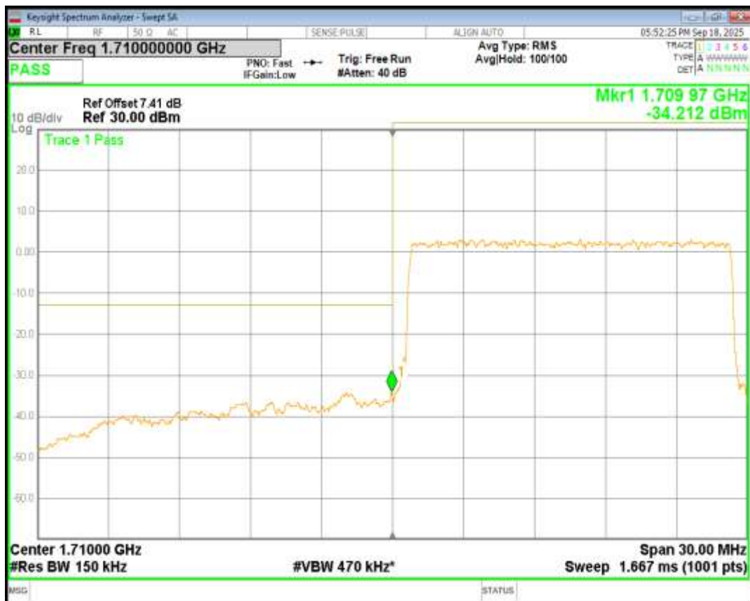
Band4 QPSK BW=15MHz Channel=20325 RB Size=75 Position=#0
