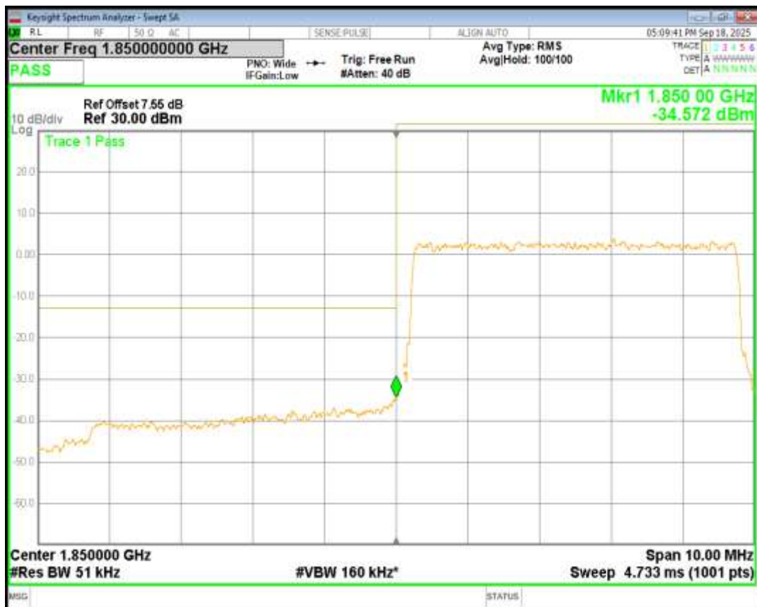
Band2 QPSK BW=5MHz Channel=19175 RB Size=25 Position=#0
