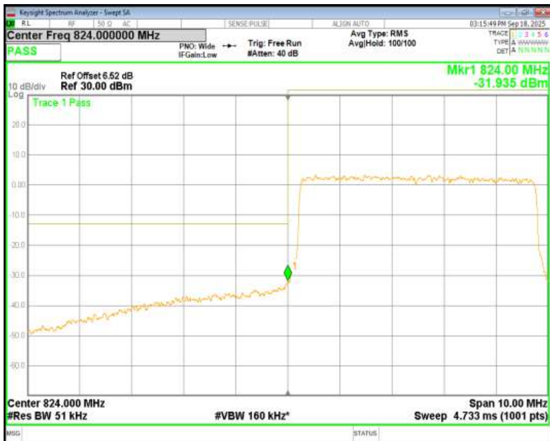
Band5 16QAM BW=5MHz Channel=20625 RB Size=25 Position=#0
