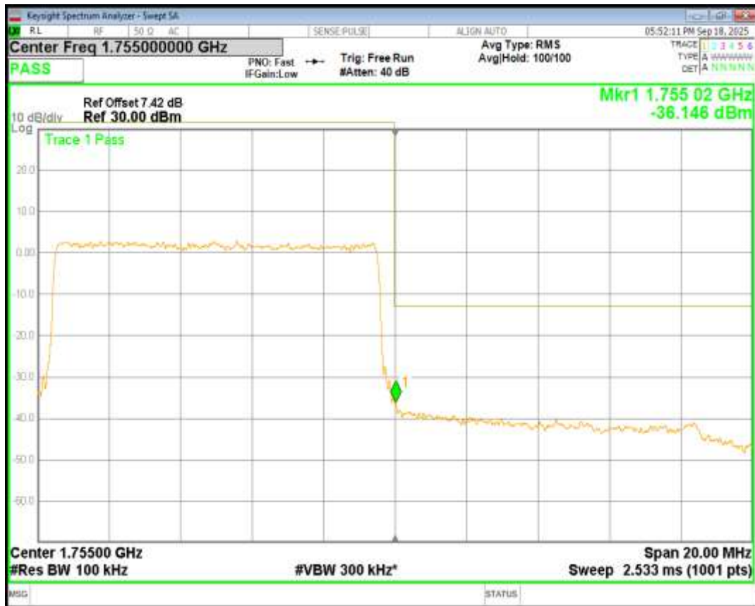
Band4 QPSK BW=15MHz Channel=20025 RB Size=75 Position=#0
