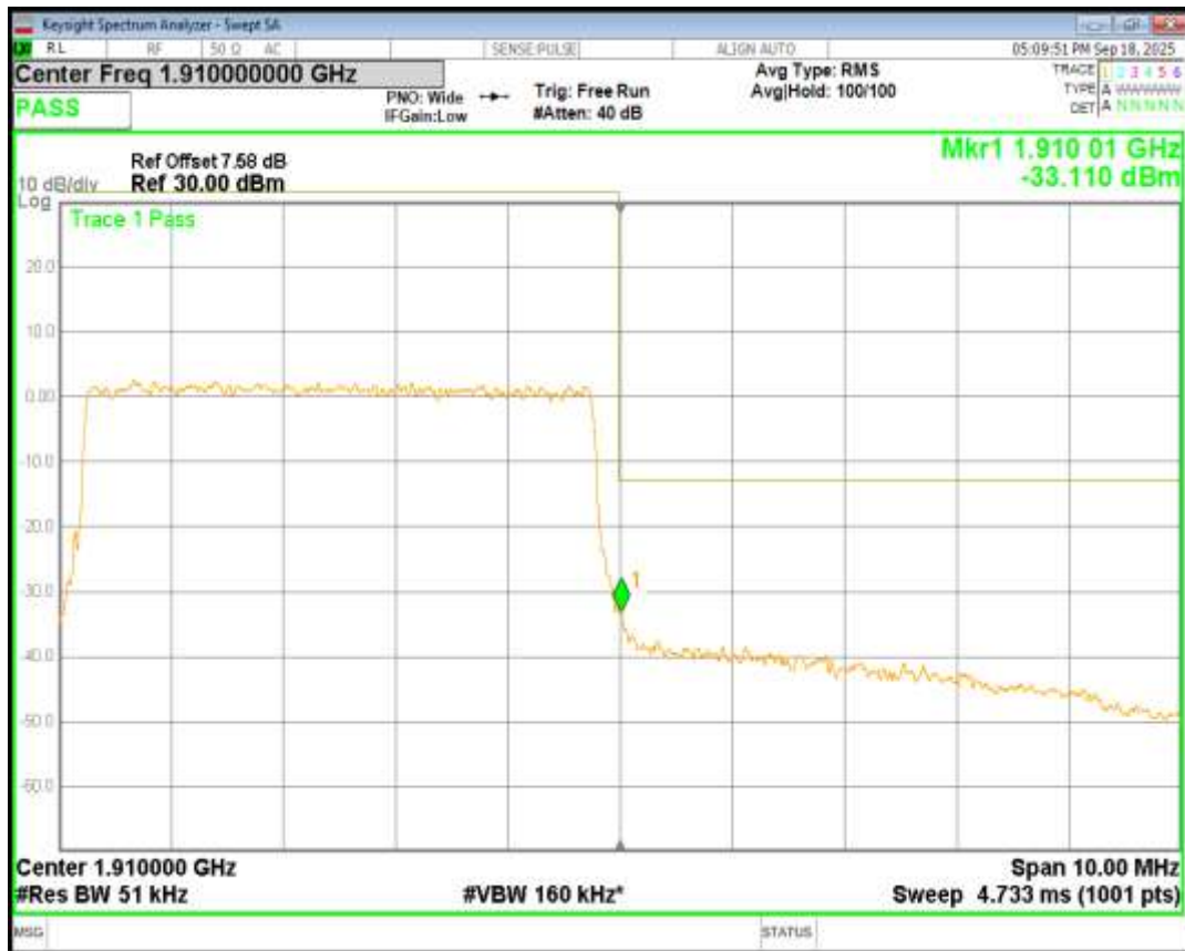
Band2 16QAM BW=3MHz Channel=18615 RB Size=15 Position=#0
