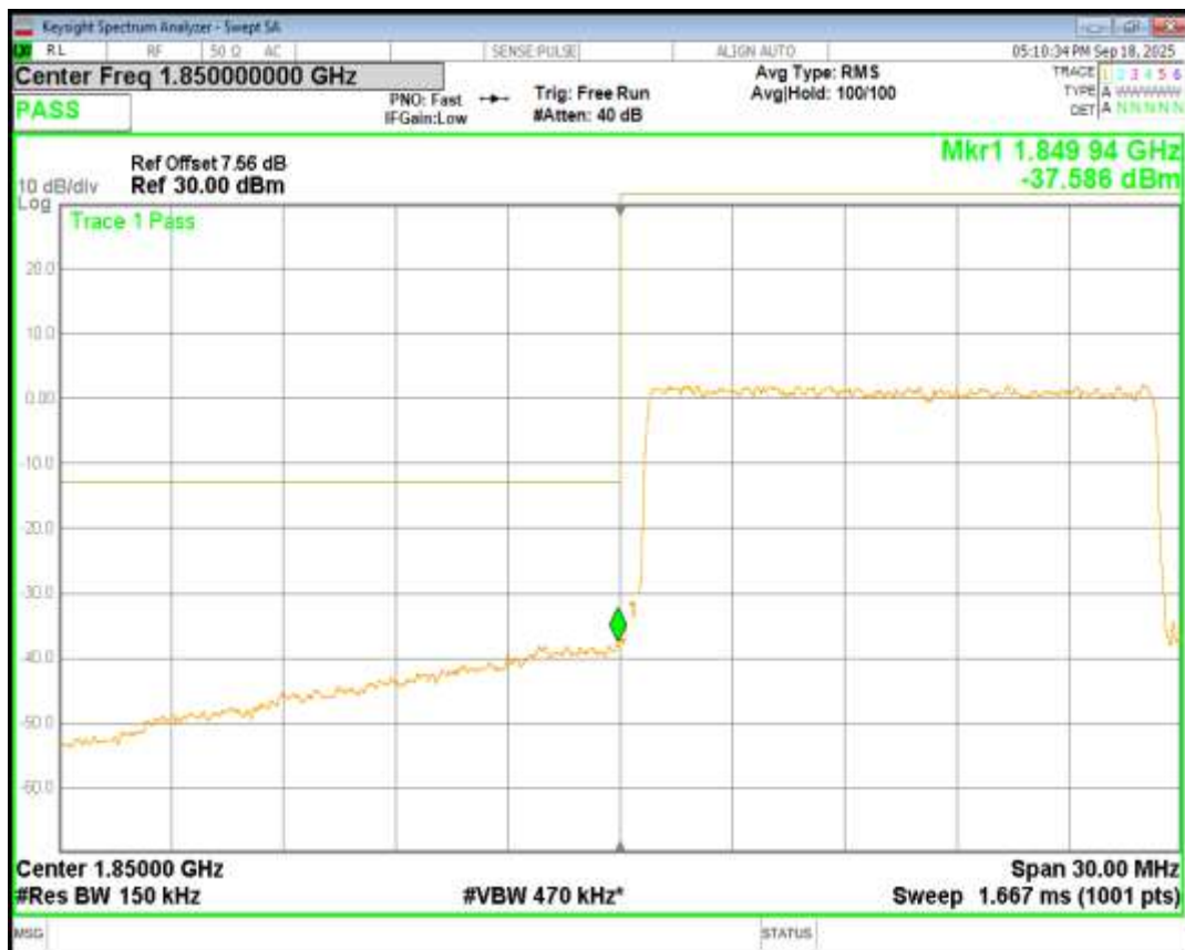
Band2 16QAM BW=15MHz Channel=19125 RB Size=75 Position=#0
