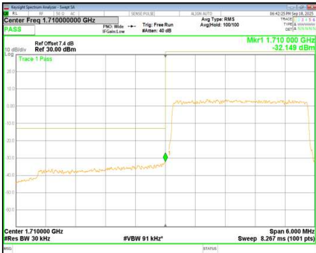
Band66 QPSK BW=3MHz Channel=132657 RB Size=15 Position=#0
