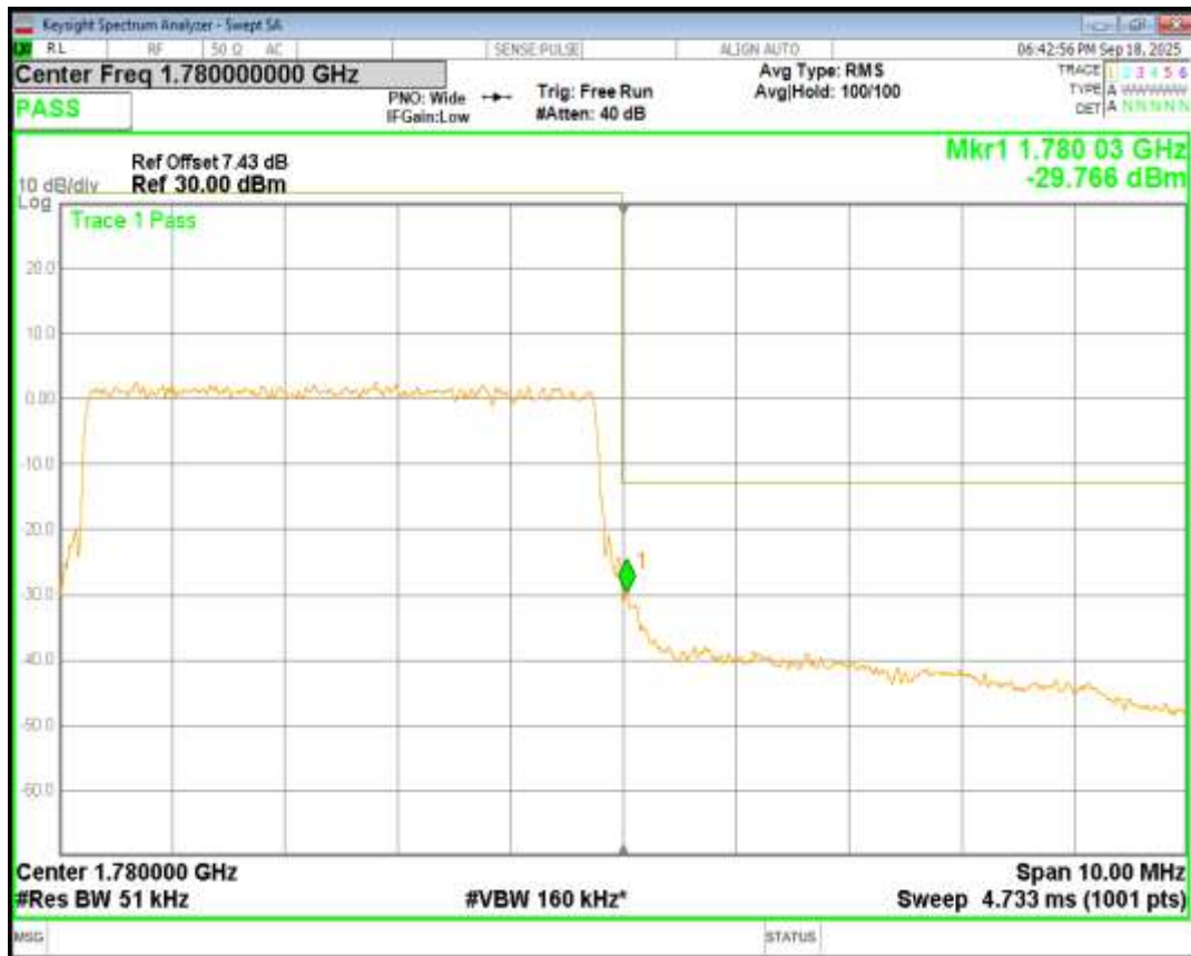
Band66 16QAM BW=20MHz Channel=132572 RB Size=100 Position=#0
