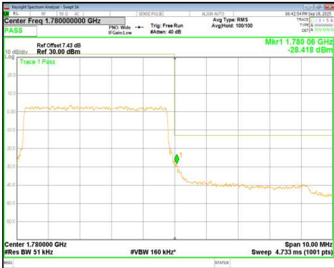
Band7 16QAM BW=10MHz Channel=20800 RB Size=50 Position=#0
