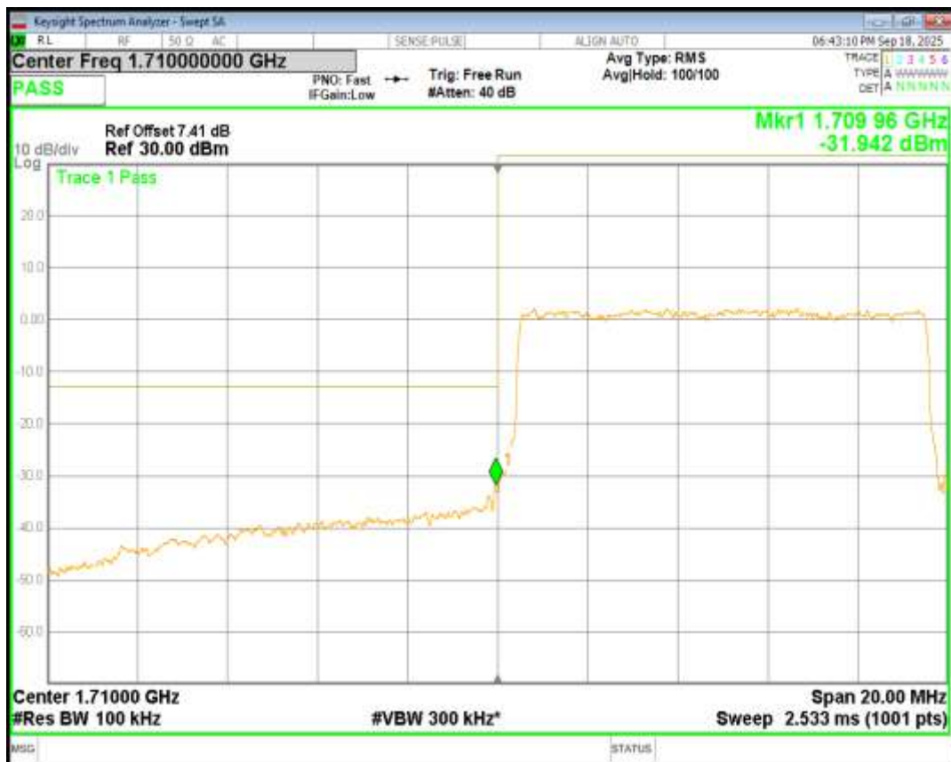
Band66 16QAM BW=10MHz Channel=132622 RB Size=50 Position=#0
