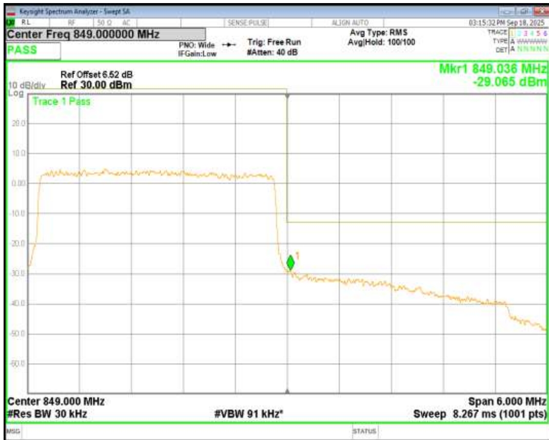
Band5 QPSK BW=5MHz Channel=20425 RB Size=25 Position=#0
