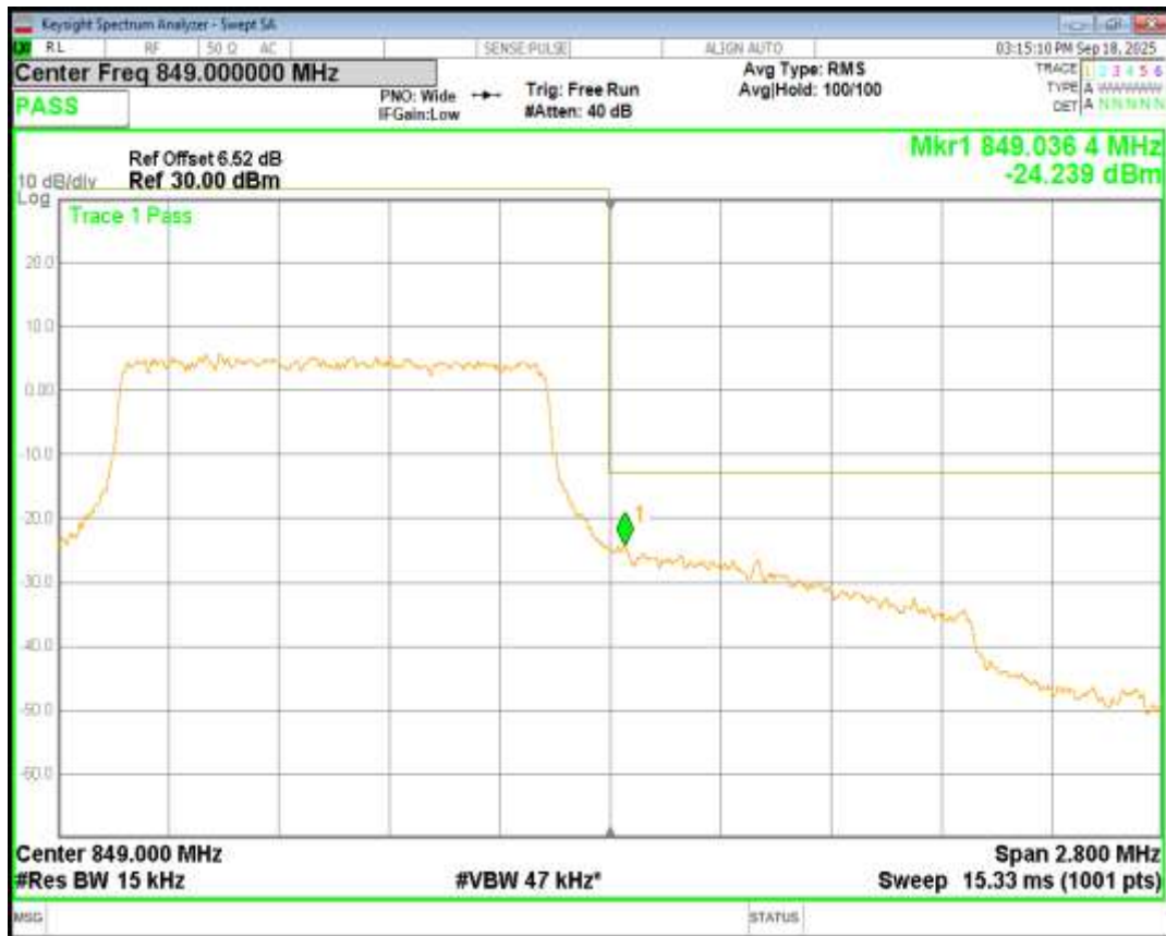
Band5 QPSK BW=10MHz Channel=20450 RB Size=50 Position=#0
