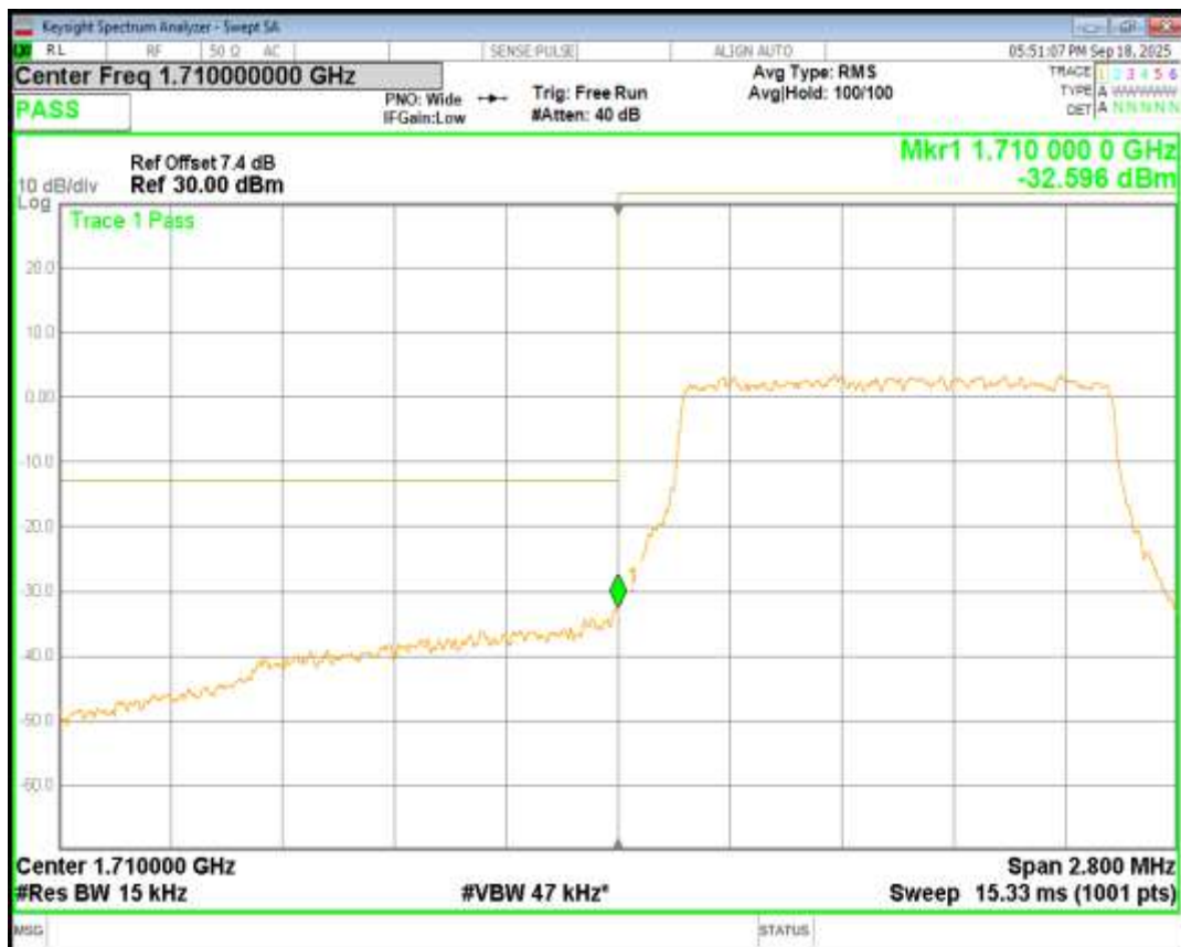
Band4 16QAM BW=1.4MHz Channel=20393 RB Size=6 Position=#0
