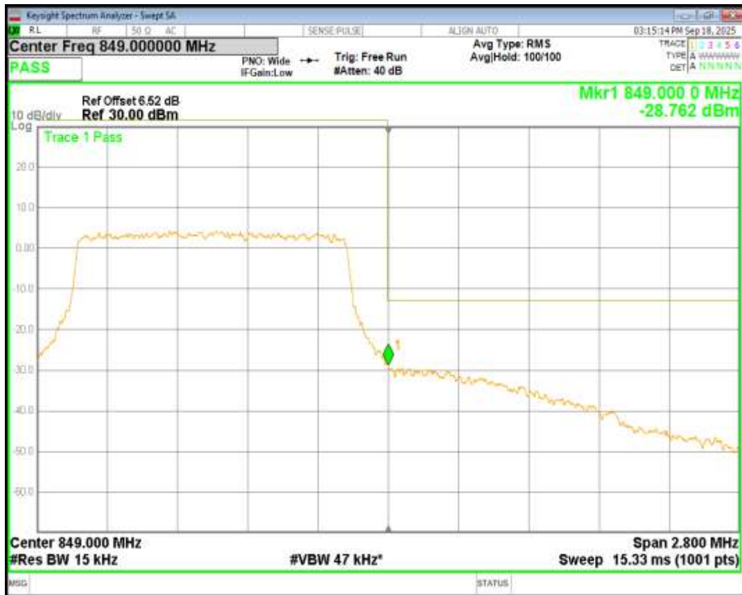
Band5 16QAM BW=10MHz Channel=20450 RB Size=50 Position=#0
