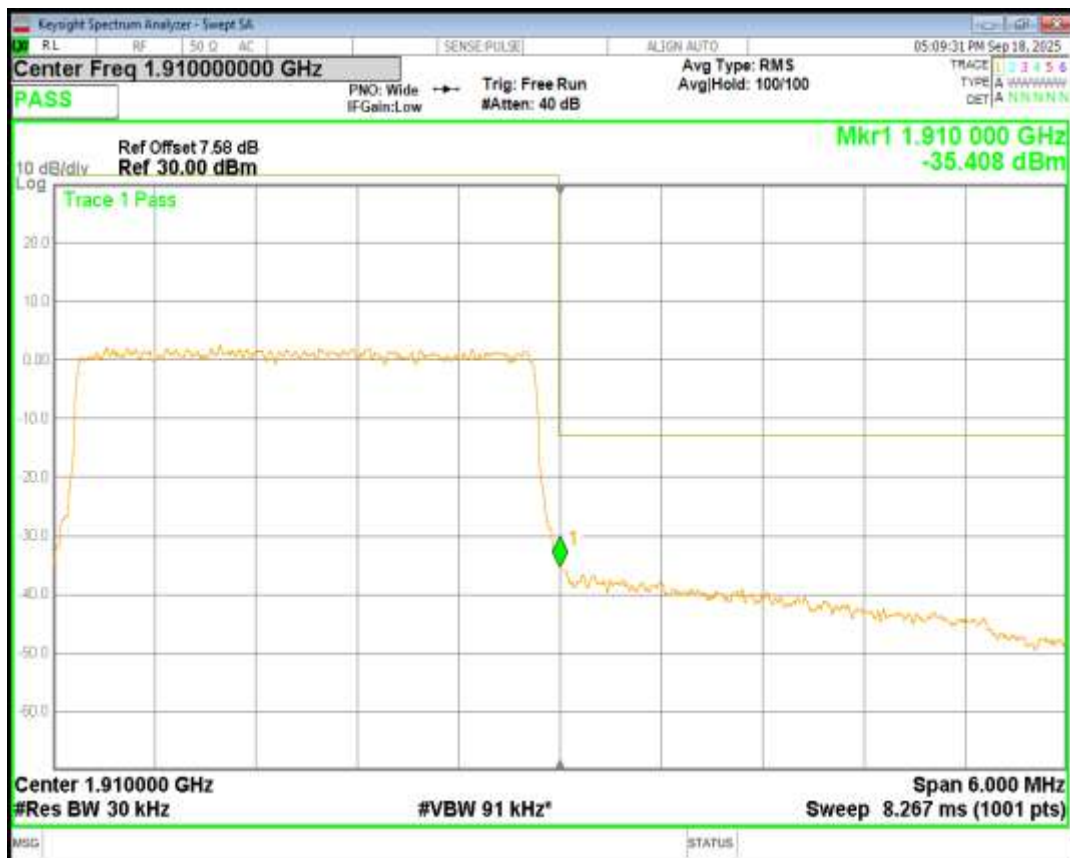
Band2 QPSK BW=1.4MHz Channel=19193 RB Size=6 Position=#0
