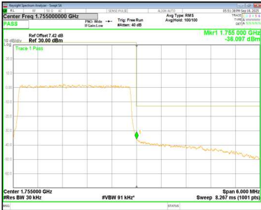
Band4 16QAM BW=5MHz Channel=20375 RB Size=25 Position=#0
