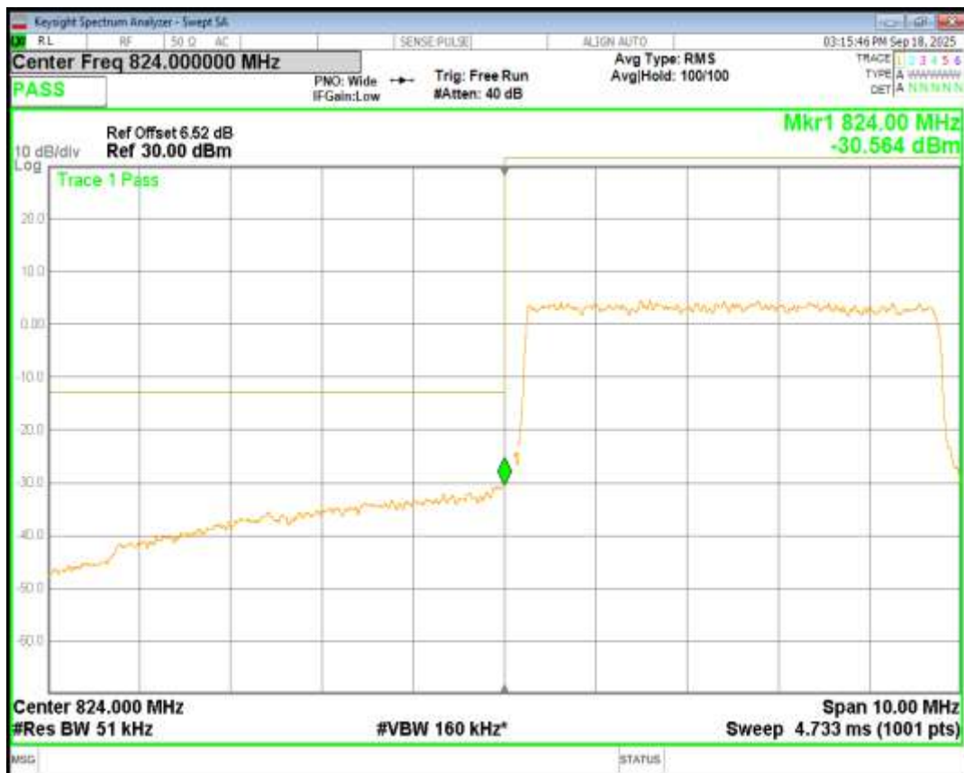
Band5 QPSK BW=5MHz Channel=20625 RB Size=25 Position=#0
