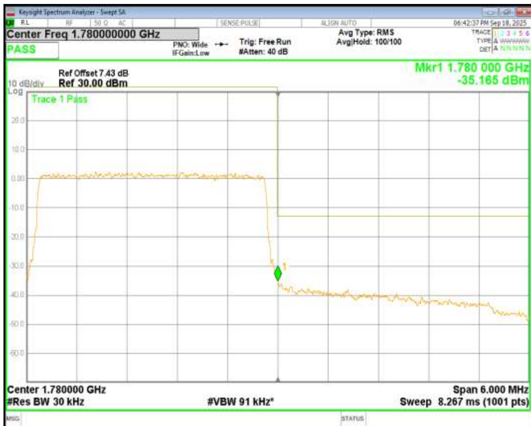
Band66 16QAM BW=5MHz Channel=132647 RB Size=25 Position=#0
