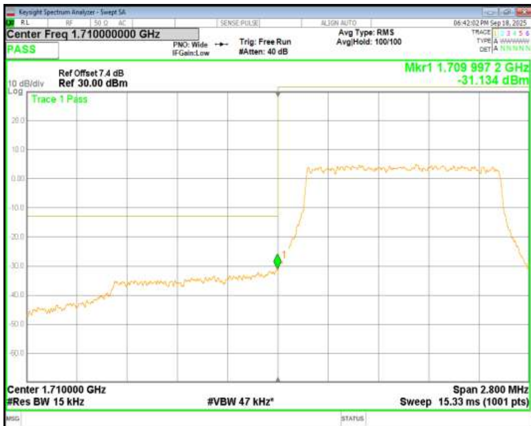
Band66 QPSK BW=1.4MHz Channel=132665 RB Size=6 Position=#0
