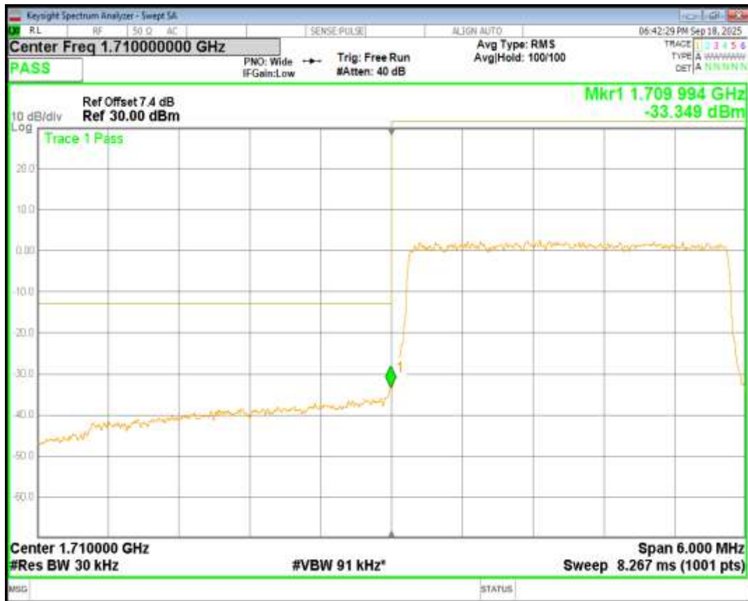
Band66 QPSK BW=1.4MHz Channel=131979 RB Size=6 Position=#0
