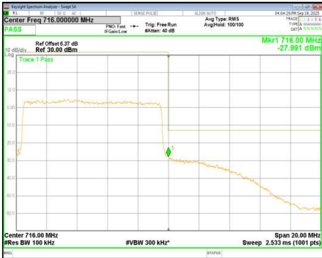
Band17 QPSK BW=5MHz Channel=23755 RB Size=25 Position=#0
