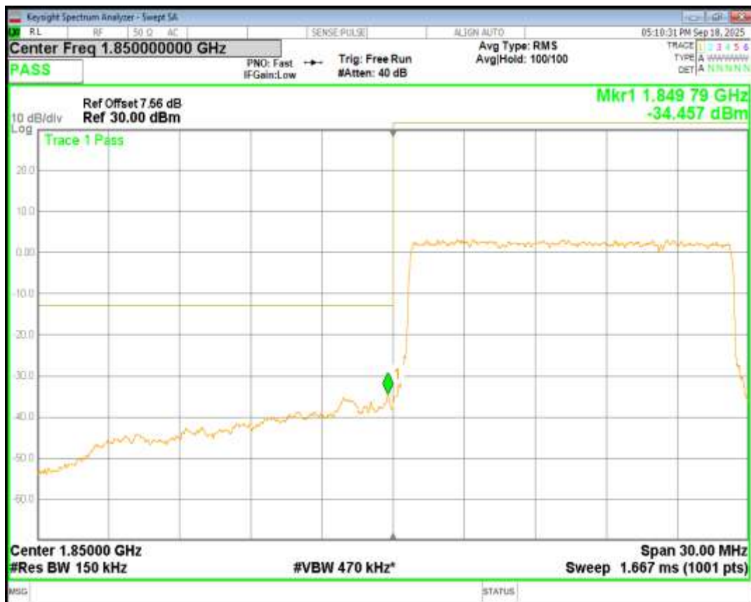
Band2 QPSK BW=15MHz Channel=19125 RB Size=75 Position=#0
