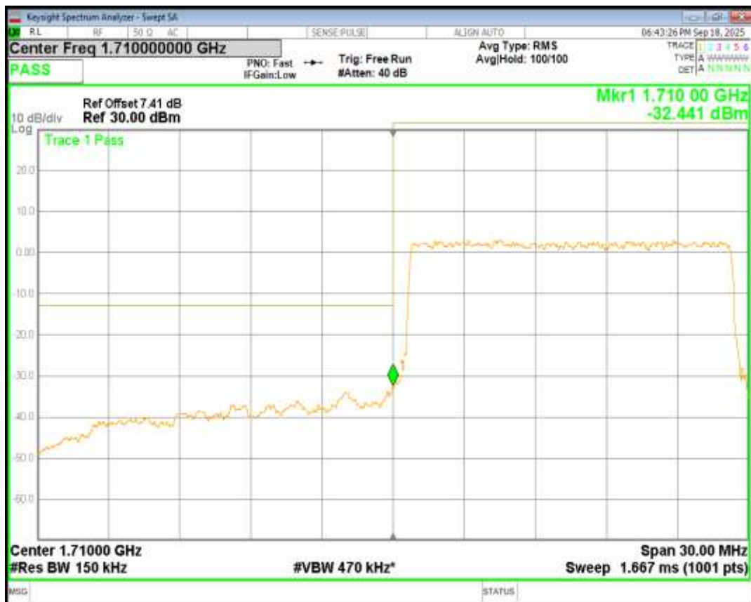
Band66 QPSK BW=15MHz Channel=132597 RB Size=75 Position=#0
