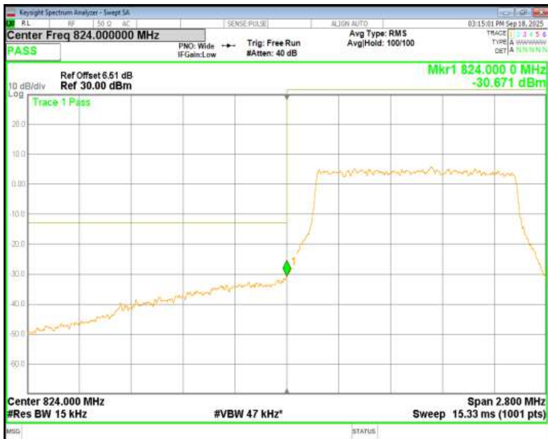
Band5 QPSK BW=1.4MHz Channel=20643 RB Size=6 Position=#0
