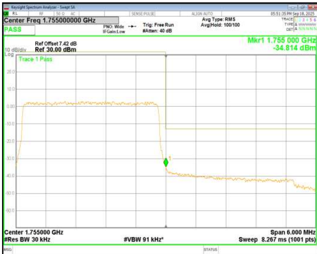
Band4 QPSK BW=5MHz Channel=20375 RB Size=25 Position=#0
