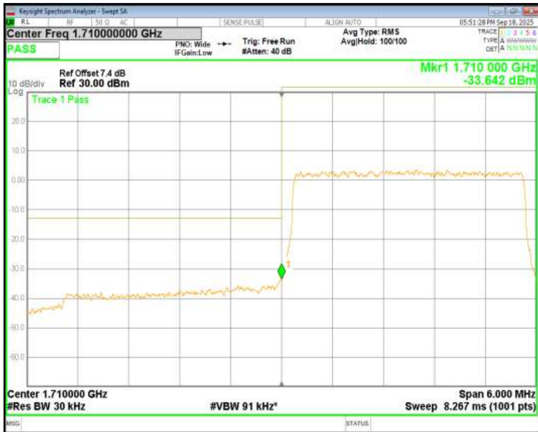
Band4 QPSK BW=3MHz Channel=20385 RB Size=15 Position=#0
