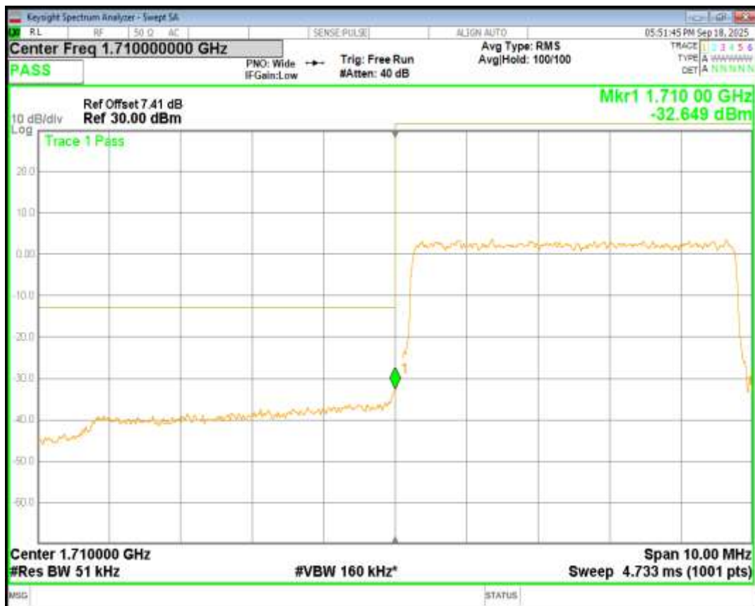
Band4 QPSK BW=20MHz Channel=20050 RB Size=100 Position=#0
