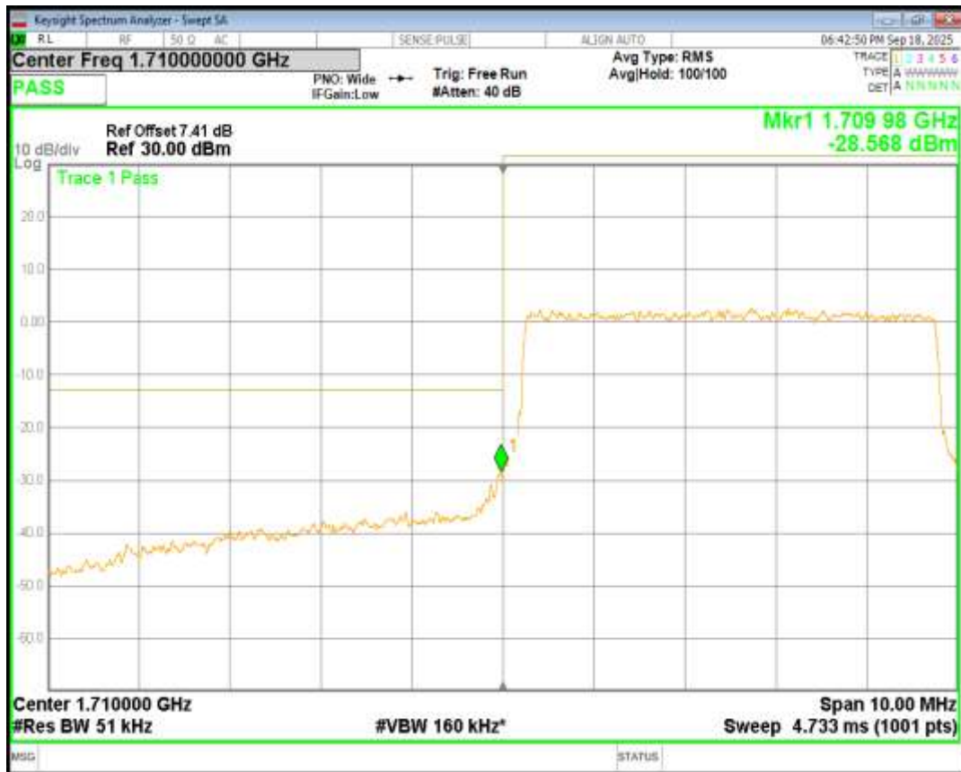
Band66 16QAM BW=3MHz Channel=132657 RB Size=15 Position=#0
