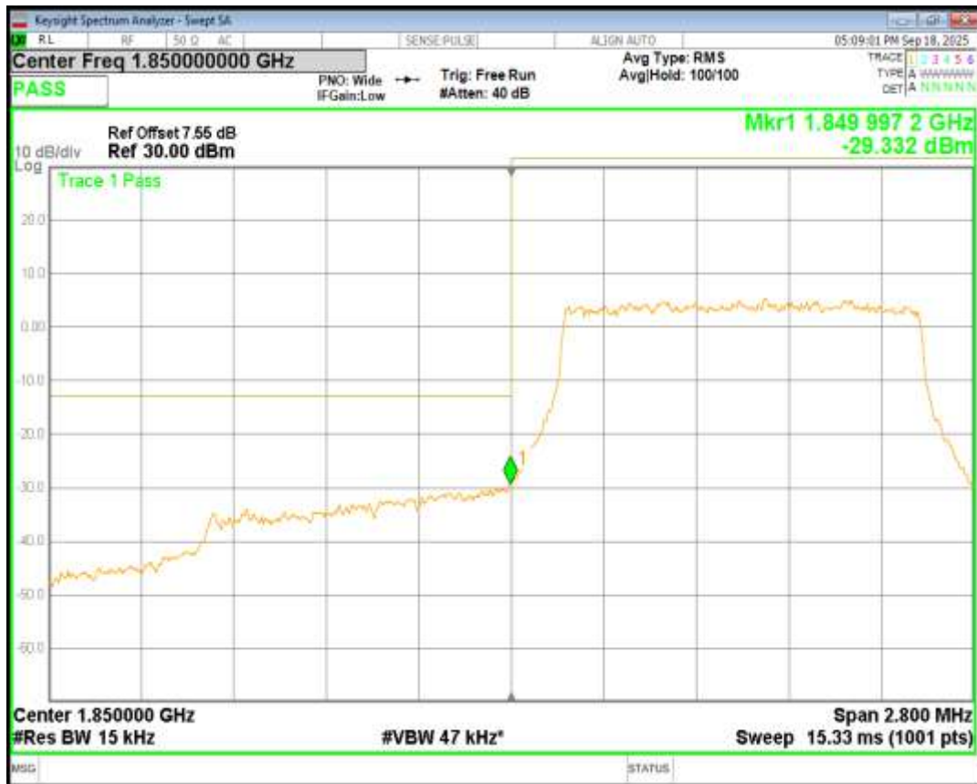
Band2 16QAM BW=5MHz Channel=18625 RB Size=25 Position=#0
