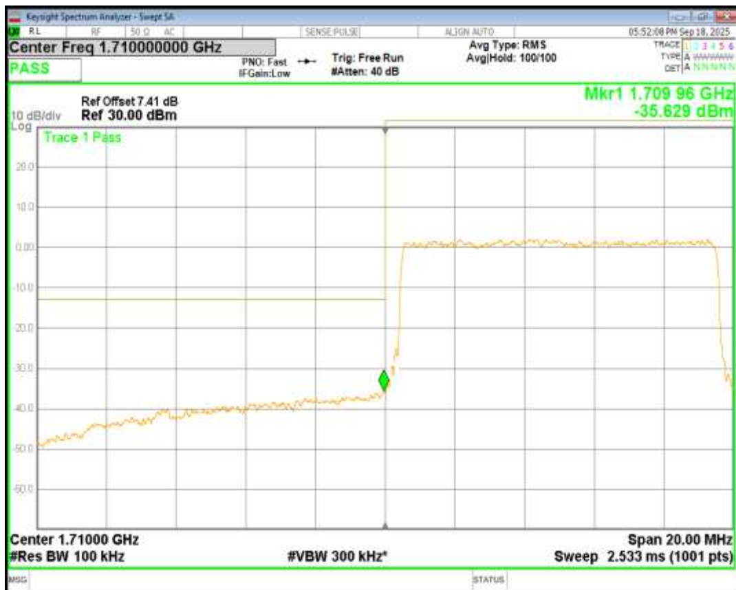
Band4 16QAM BW=10MHz Channel=20350 RB Size=50 Position=#0
