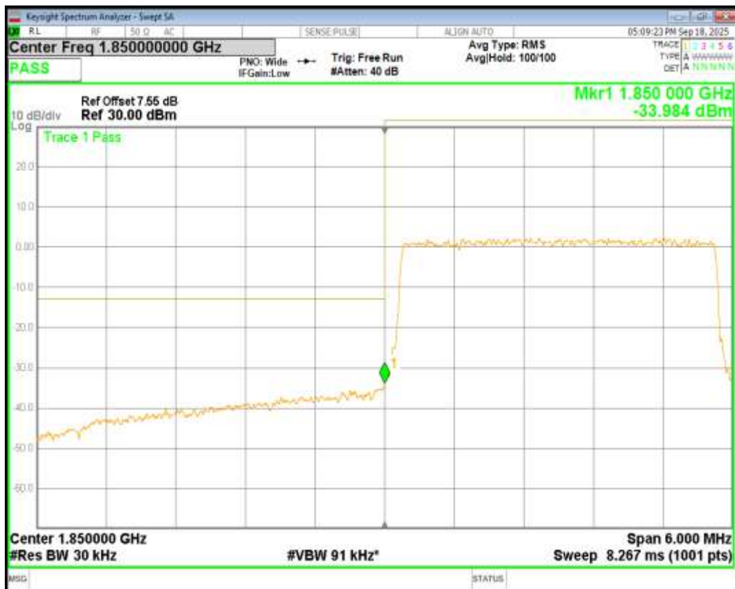
Band2 16QAM BW=20MHz Channel=19100 RB Size=100 Position=#0
