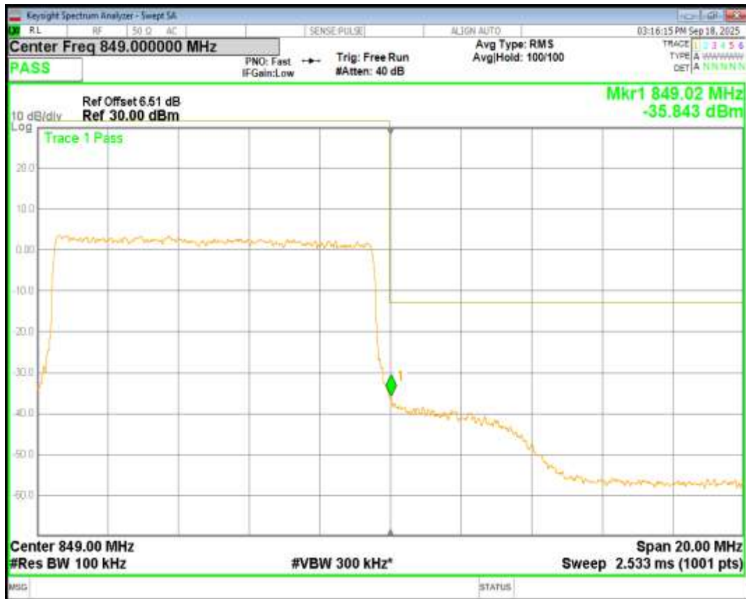
Band5 16QAM BW=3MHz Channel=20415 RB Size=15 Position=#0
