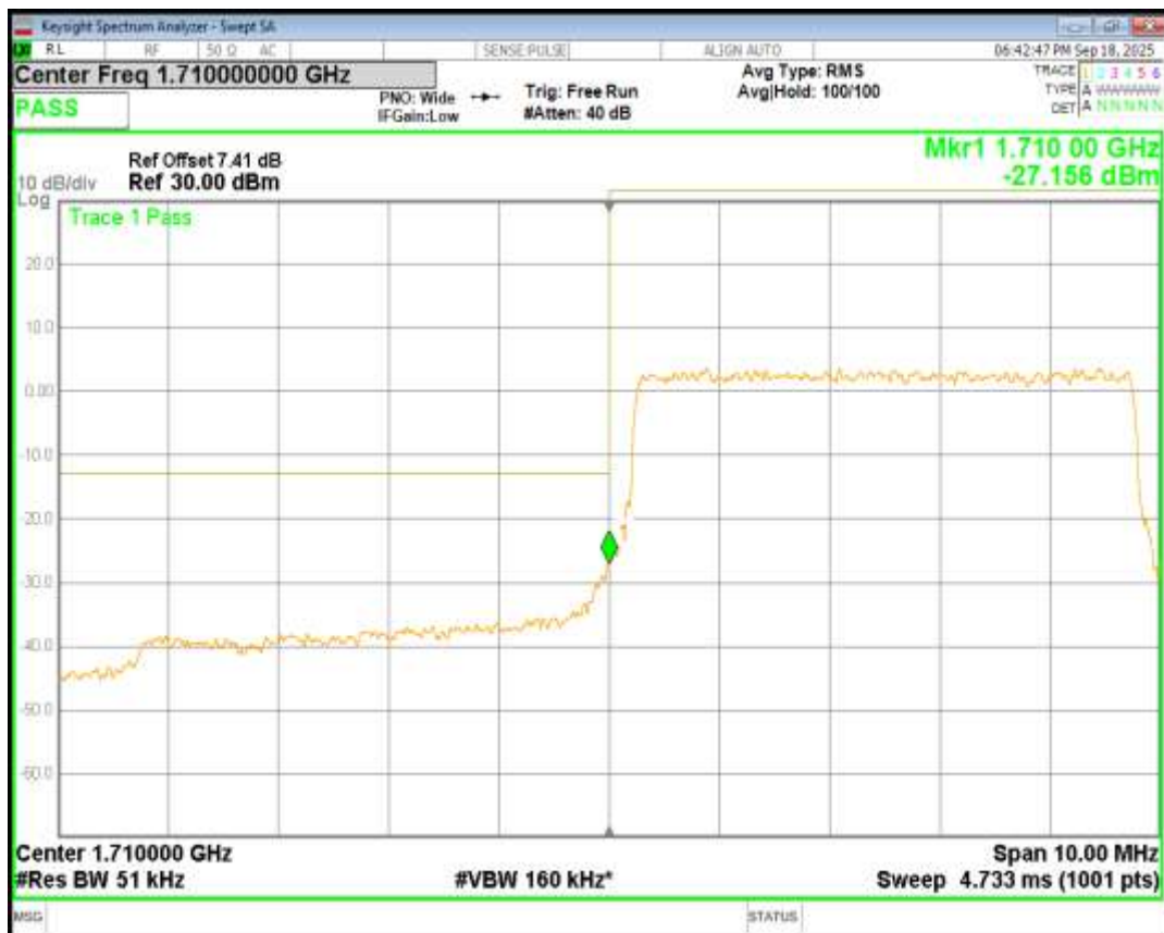
Band66 QPSK BW=5MHz Channel=132647 RB Size=25 Position=#0
