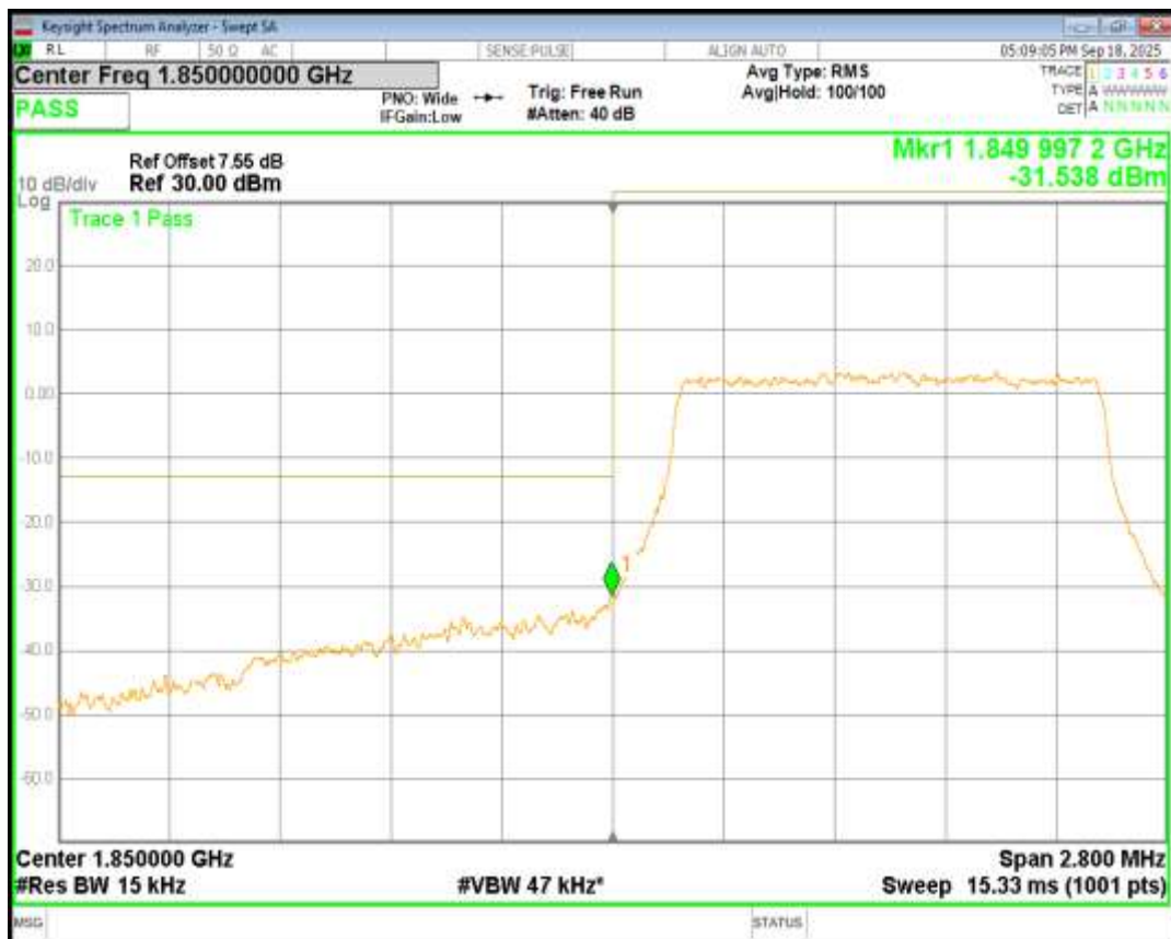
Band2 16QAM BW=1.4MHz Channel=19193 RB Size=6 Position=#0
