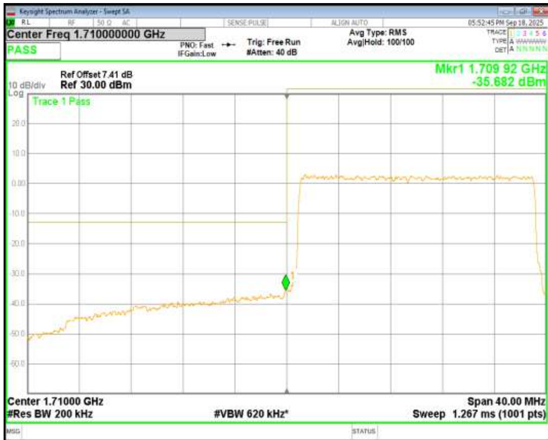
Band4 QPSK BW=20MHz Channel=20300 RB Size=100 Position=#0
