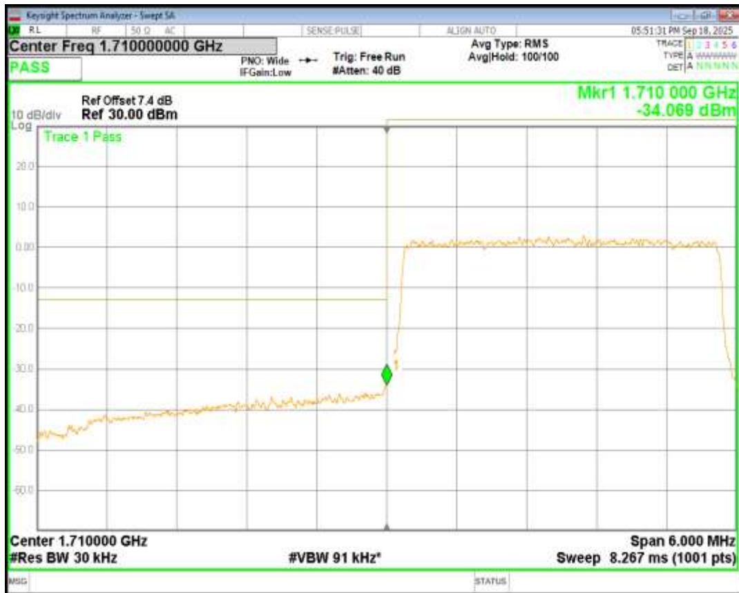
Band4 QPSK BW=1.4MHz Channel=19957 RB Size=6 Position=#0
