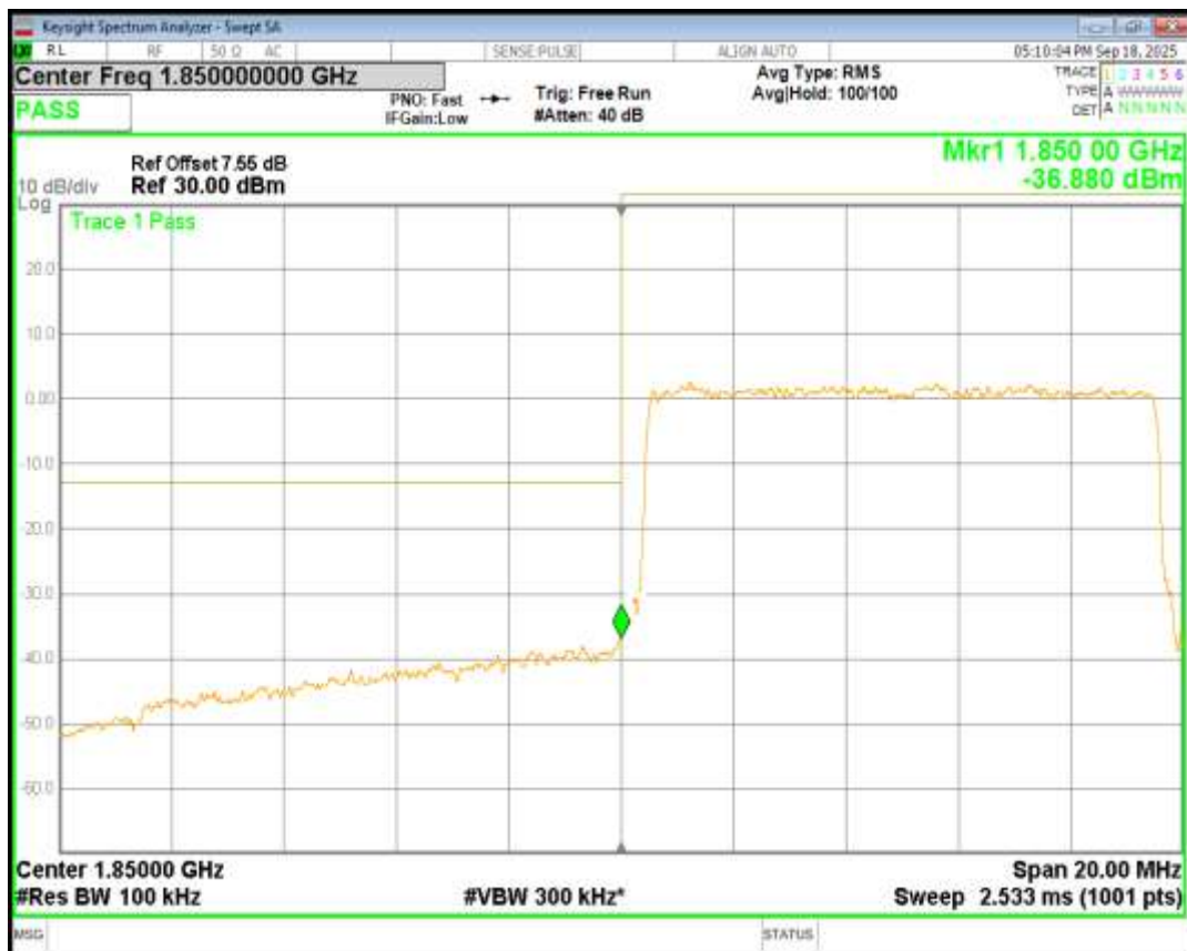
Band2 16QAM BW=10MHz Channel=19150 RB Size=50 Position=#0
