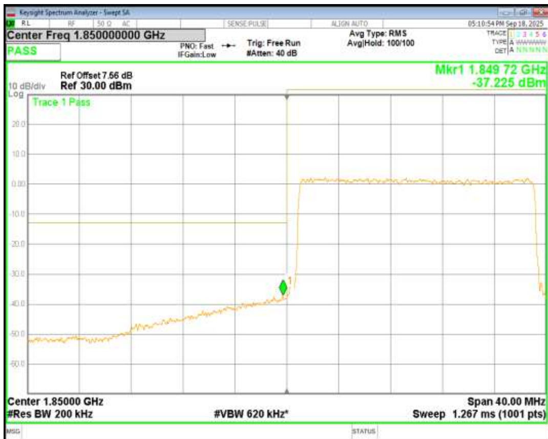
Band2 QPSK BW=1.4MHz Channel=18607 RB Size=6 Position=#0
