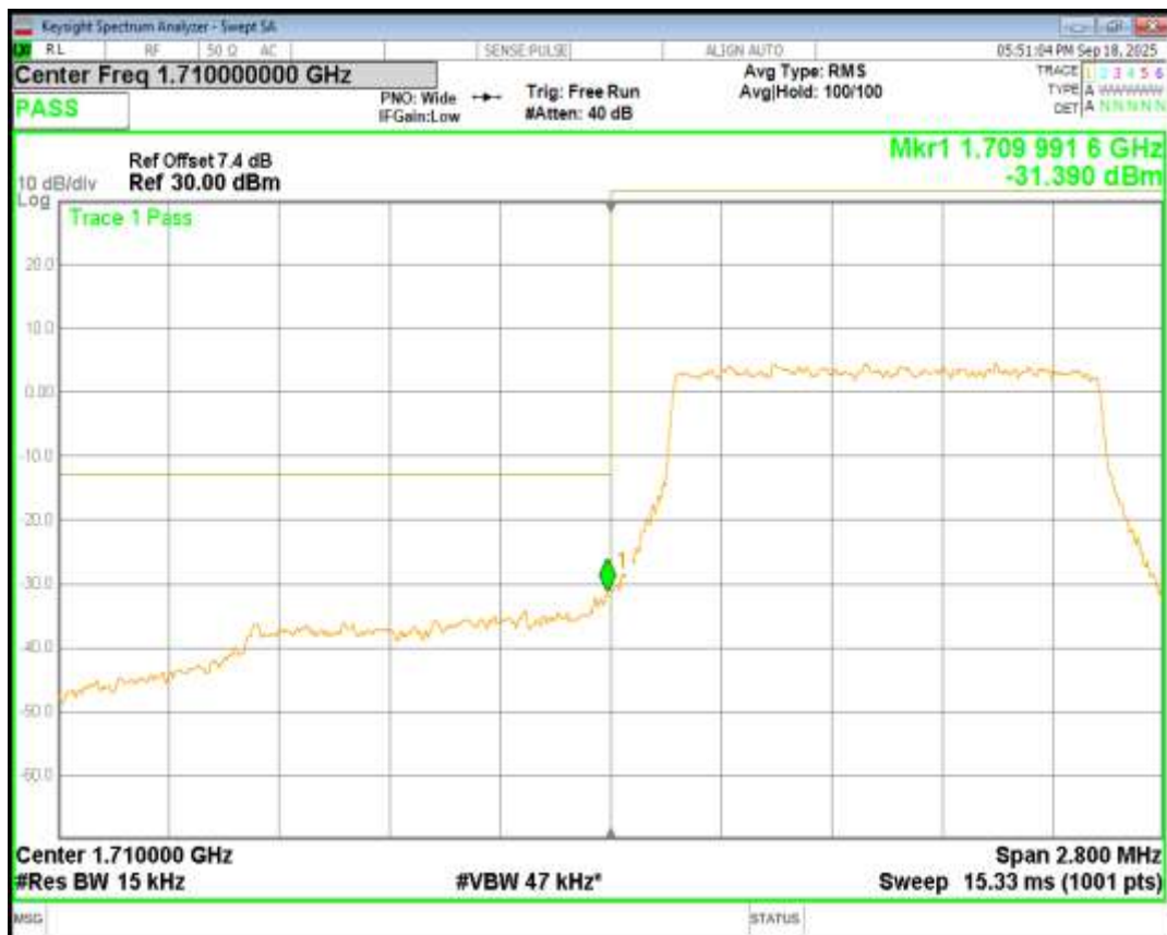
Band4 QPSK BW=1.4MHz Channel=20393 RB Size=6 Position=#0
