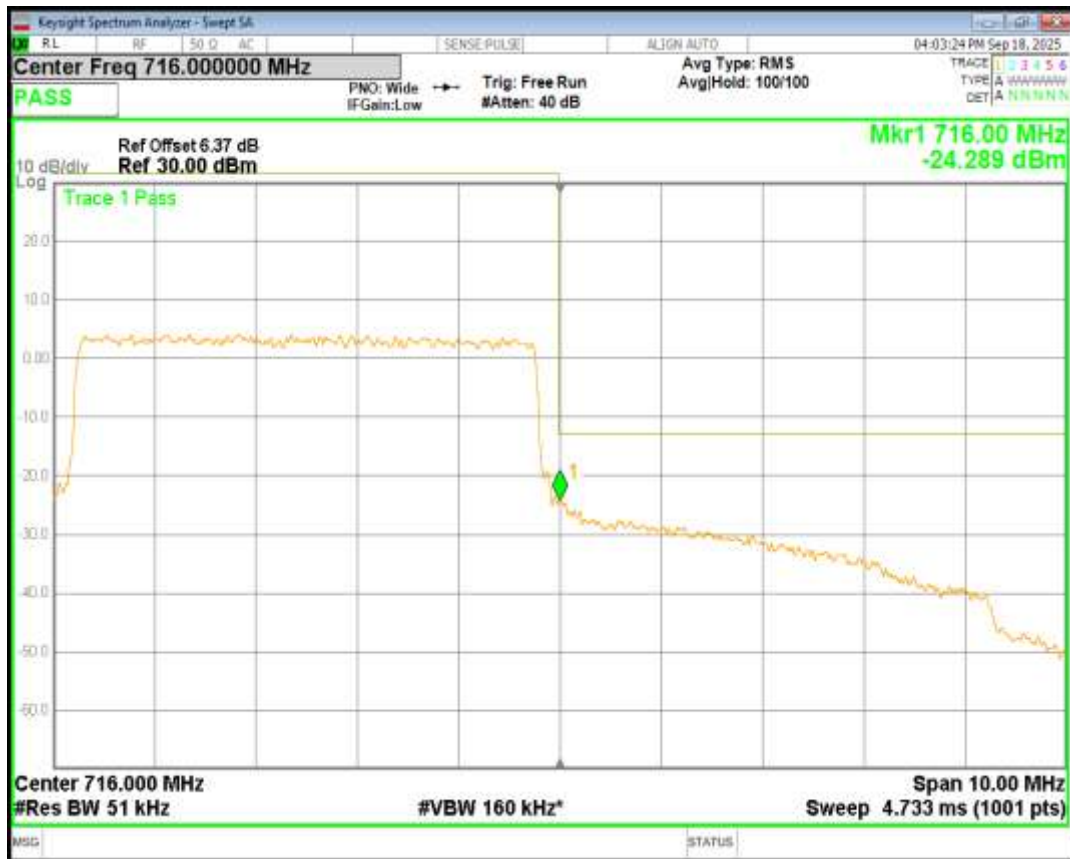
Band2 16QAM BW=1.4MHz Channel=18607 RB Size=6 Position=#0
