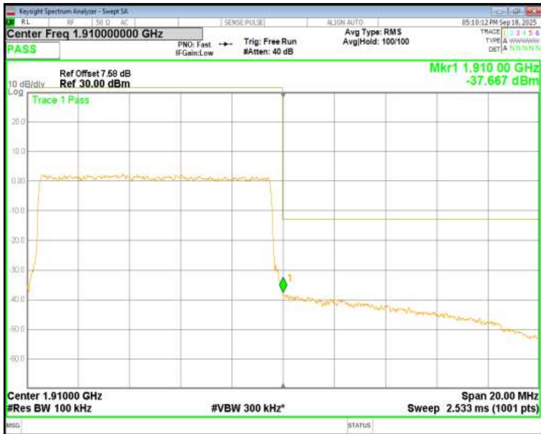
Band2 16QAM BW=15MHz Channel=18675 RB Size=75 Position=#0
