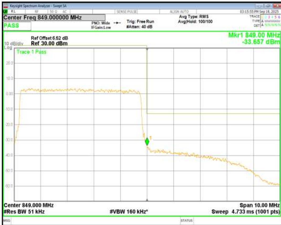
Band5 QPSK BW=1.4MHz Channel=20407 RB Size=6 Position=#0
