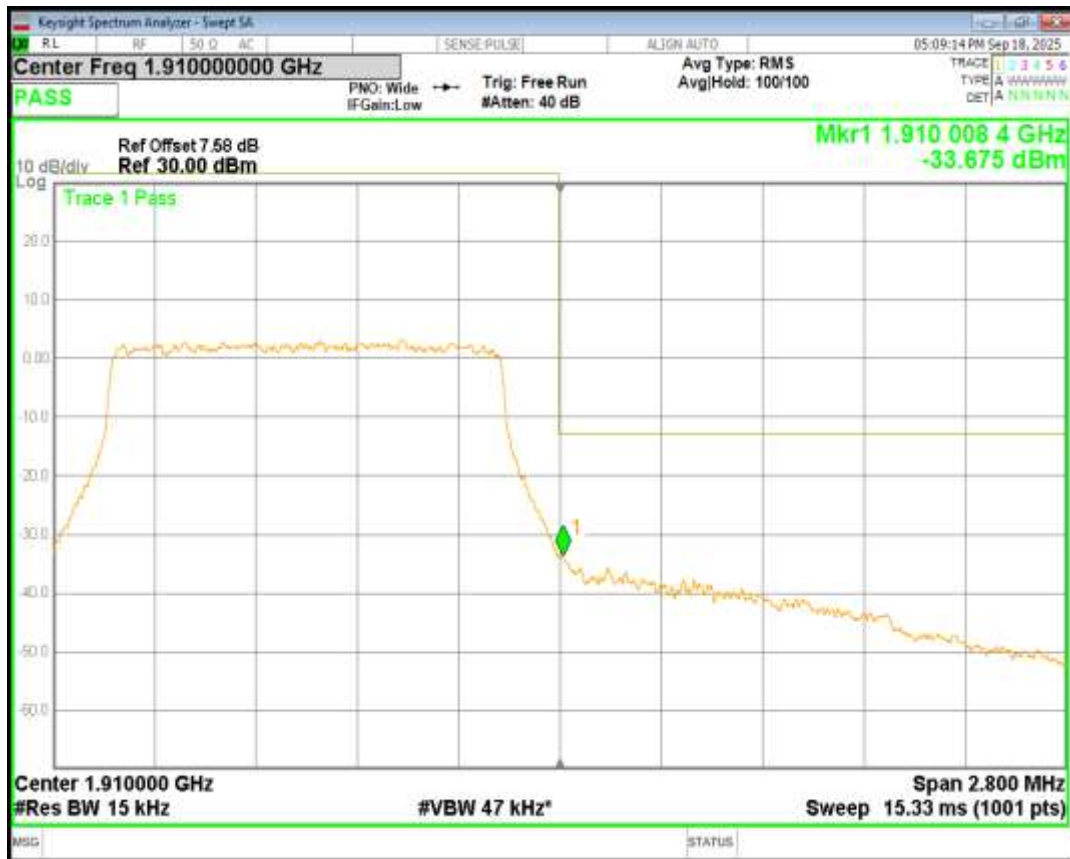
Band2 16QAM BW=10MHz Channel=18650 RB Size=50 Position=#0
