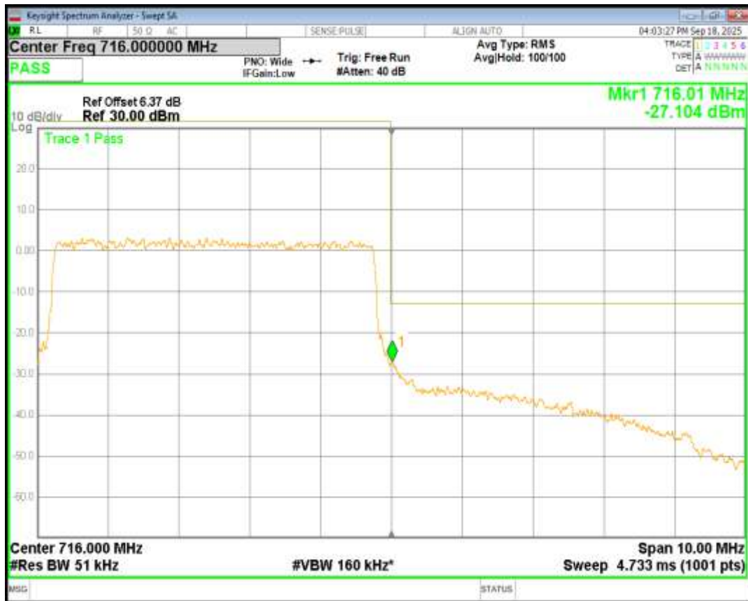
Band17 QPSK BW=10MHz Channel=23780 RB Size=50 Position=#0
