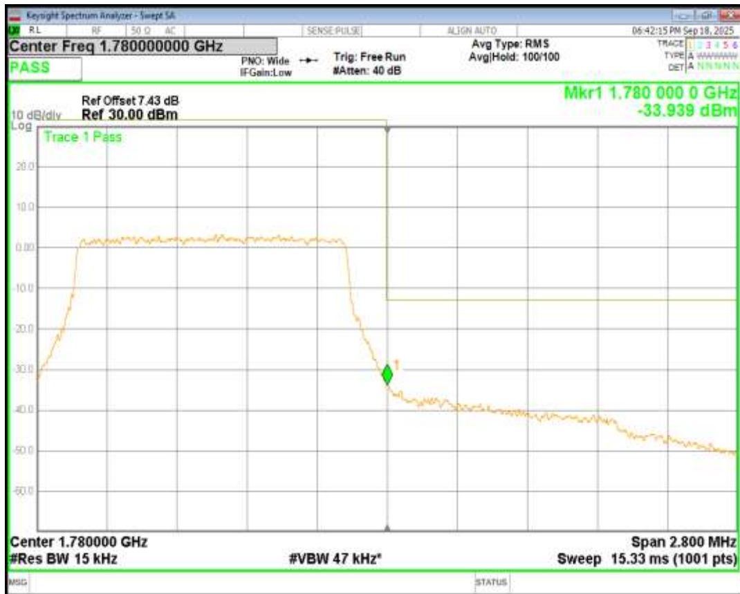
Band66 16QAM BW=10MHz Channel=132022 RB Size=50 Position=#0
