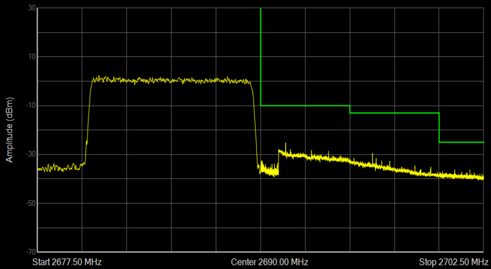
Band41 16QAM BW=10MHz Channel=41540 RB Size=50 Position=#0
