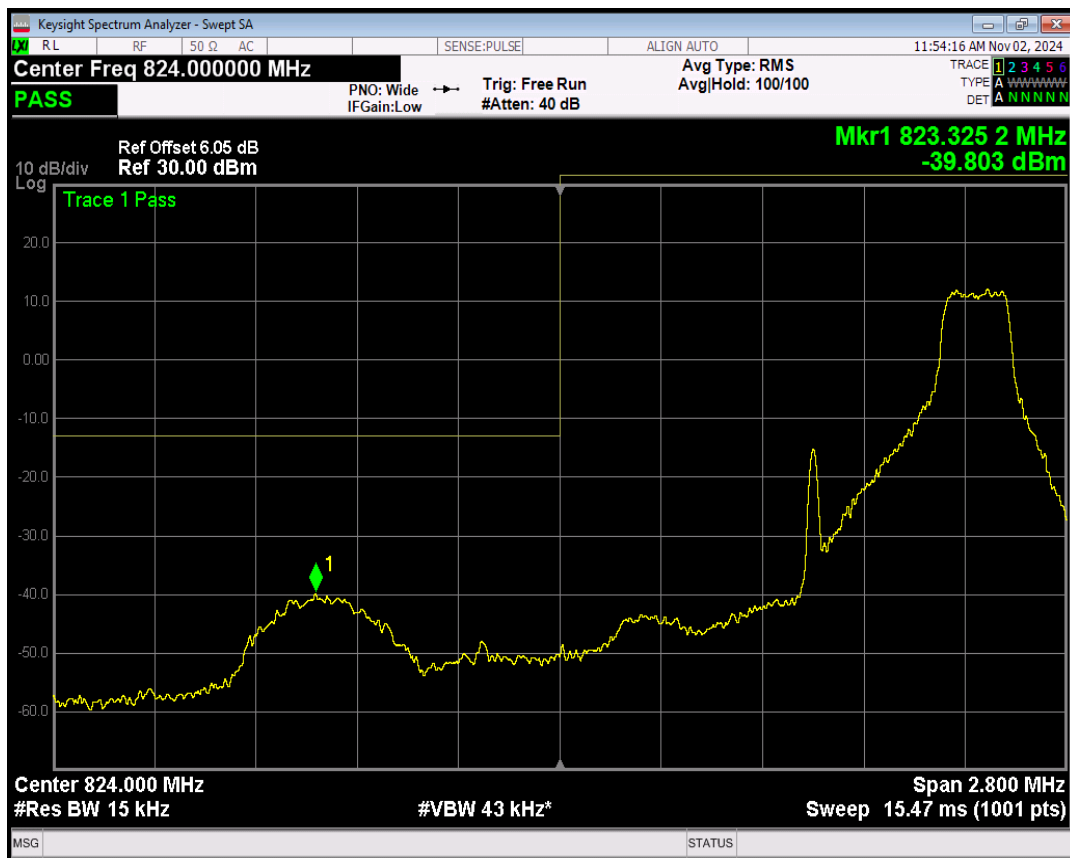
Band5 QPSK BW=1.4MHz Channel=20407 RB Size=6 Position=#0
