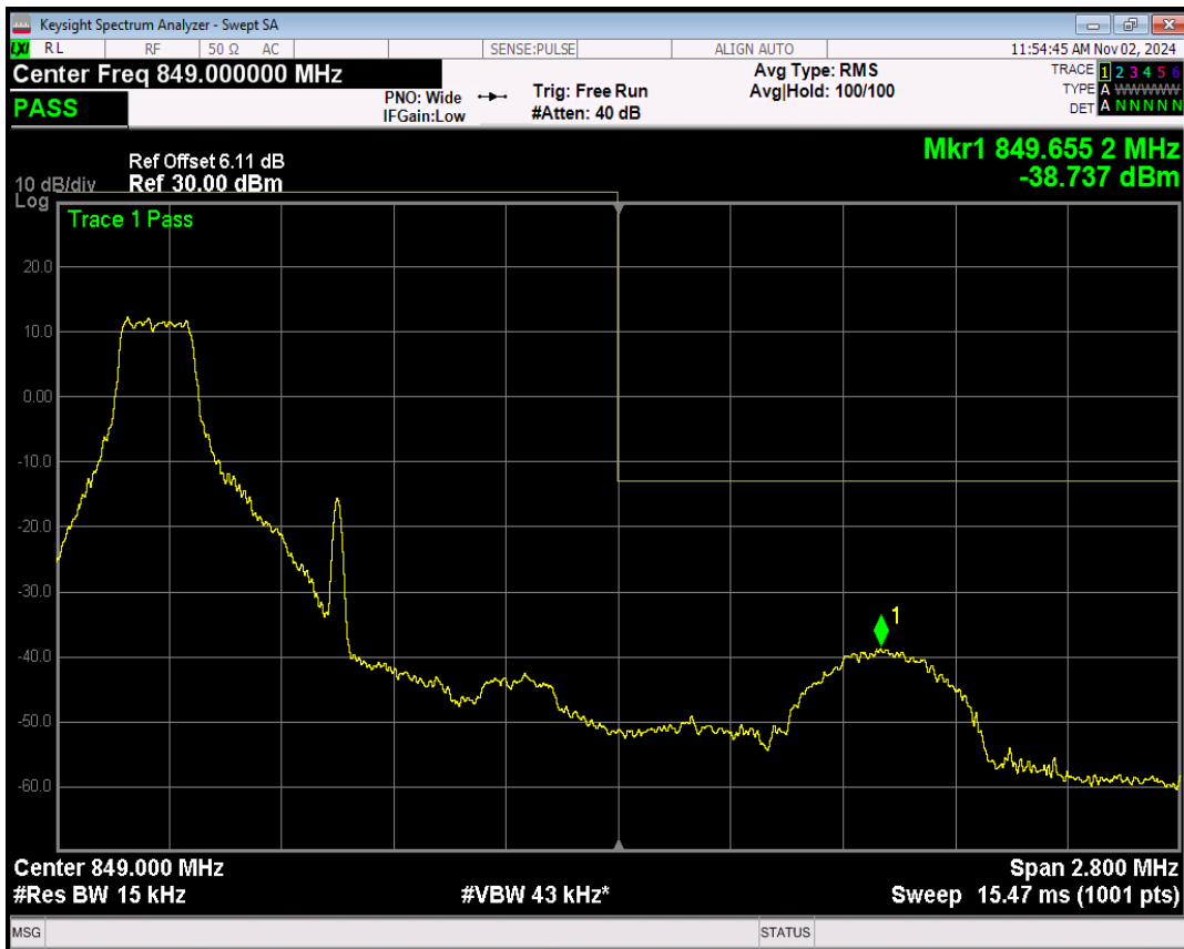
Band5 16QAM BW=1.4MHz Channel=20643 RB Size=1 Position=#Max
