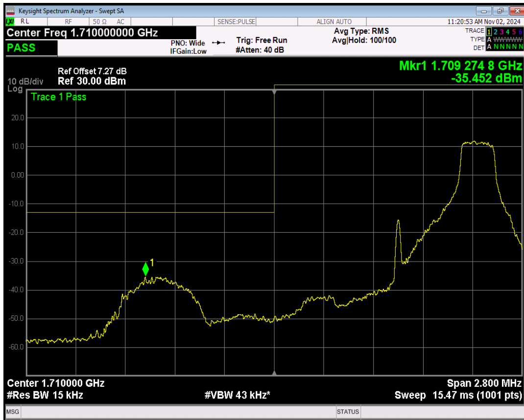
Band4 16QAM BW=1.4MHz Channel=19957 RB Size=6 Position=#0
