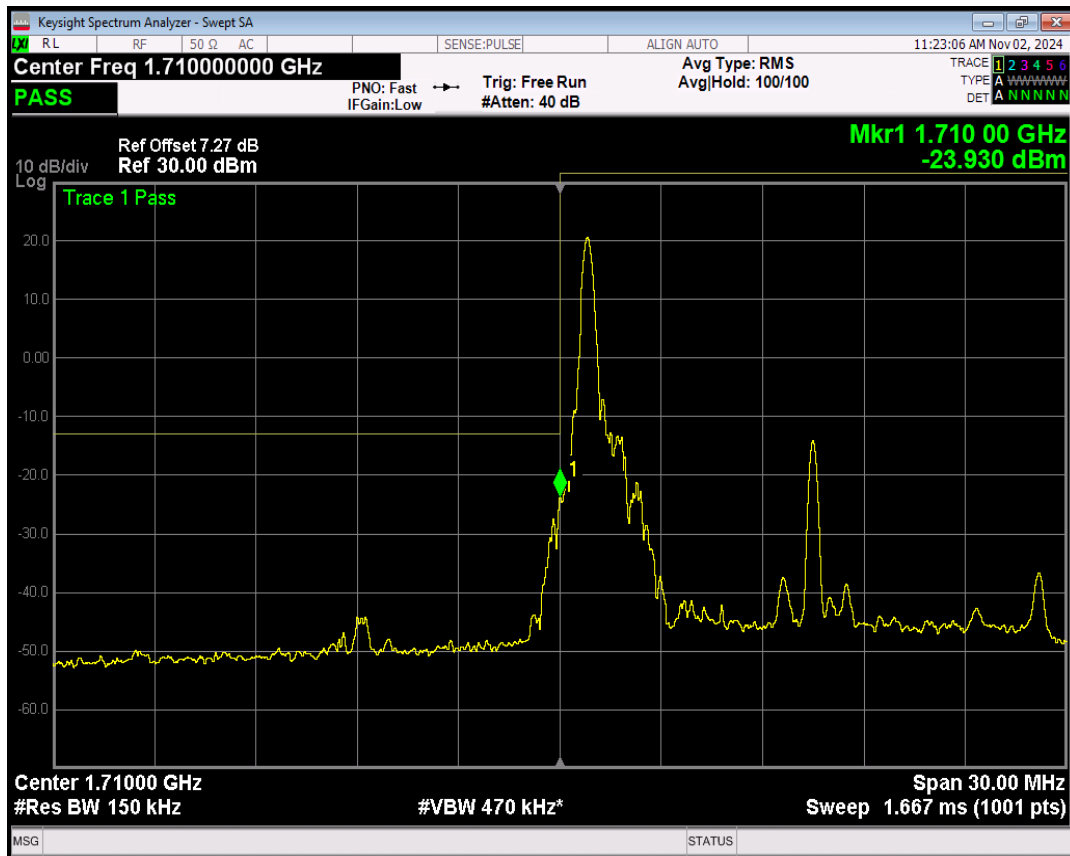
Band4 16QAM BW=15MHz Channel=20025 RB Size=1 Position=#Max
