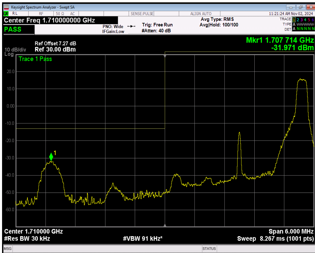
Band4 QPSK BW=3MHz Channel=19965 RB Size=15 Position=#0
