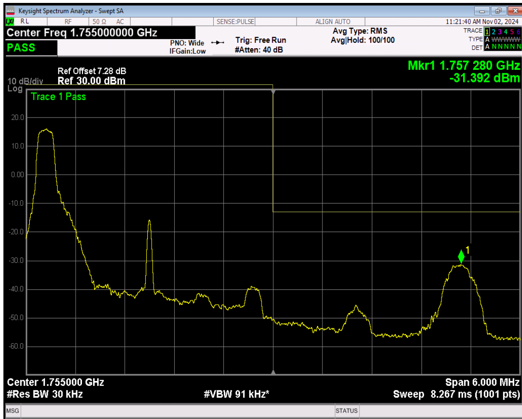
Band4 QPSK BW=3MHz Channel=20385 RB Size=1 Position=#Max
