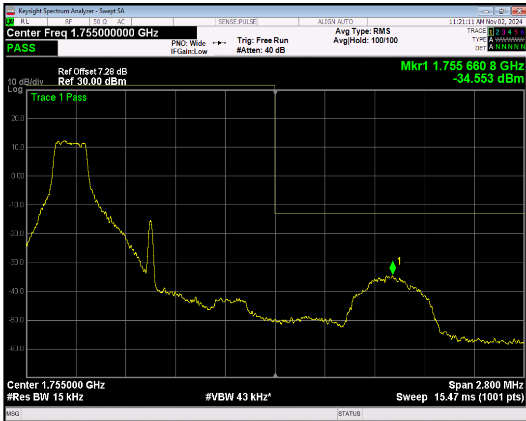
Band4 16QAM BW=1.4MHz Channel=20393 RB Size=1 Position=#Max
