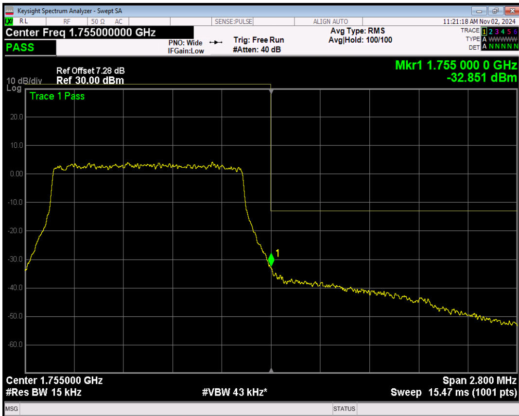
Band4 QPSK BW=3MHz Channel=19965 RB Size=1 Position=#0
