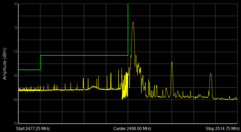
Band41 16QAM BW=15MHz Channel=39725 RB Size=1 Position=#0
