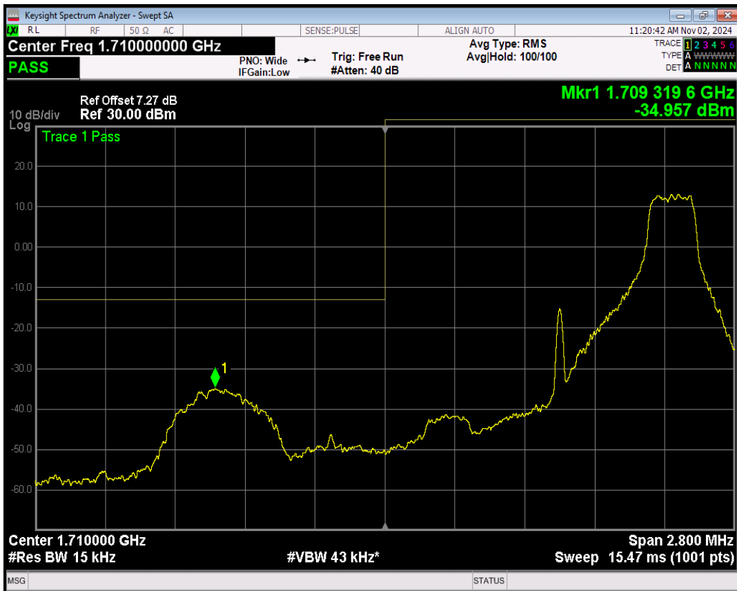
Band4 QPSK BW=1.4MHz Channel=19957 RB Size=6 Position=#0
