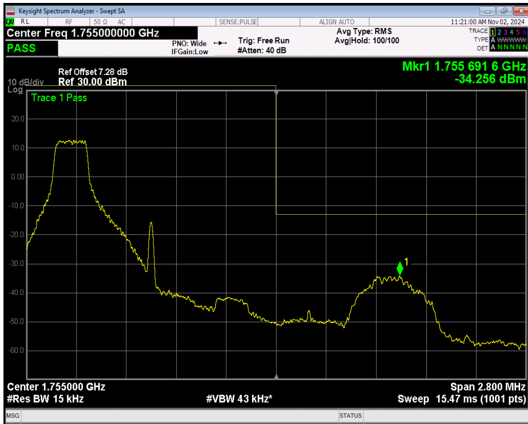
Band4 QPSK BW=1.4MHz Channel=20393 RB Size=1 Position=#Max
