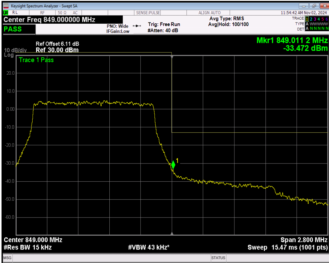
Band5 16QAM BW=1.4MHz Channel=20643 RB Size=1 Position=#0
