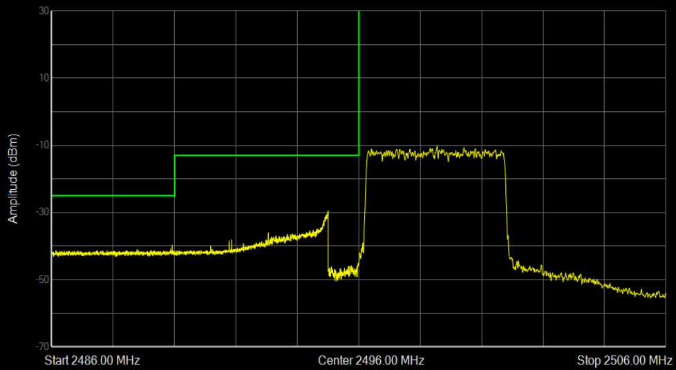
Band41 16QAM BW=5MHz Channel=39675 RB Size=25 Position=#0
