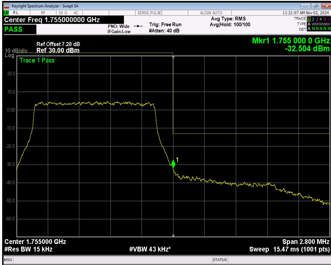
Band4 16QAM BW=1.4MHz Channel=20393 RB Size=1 Position=#0
