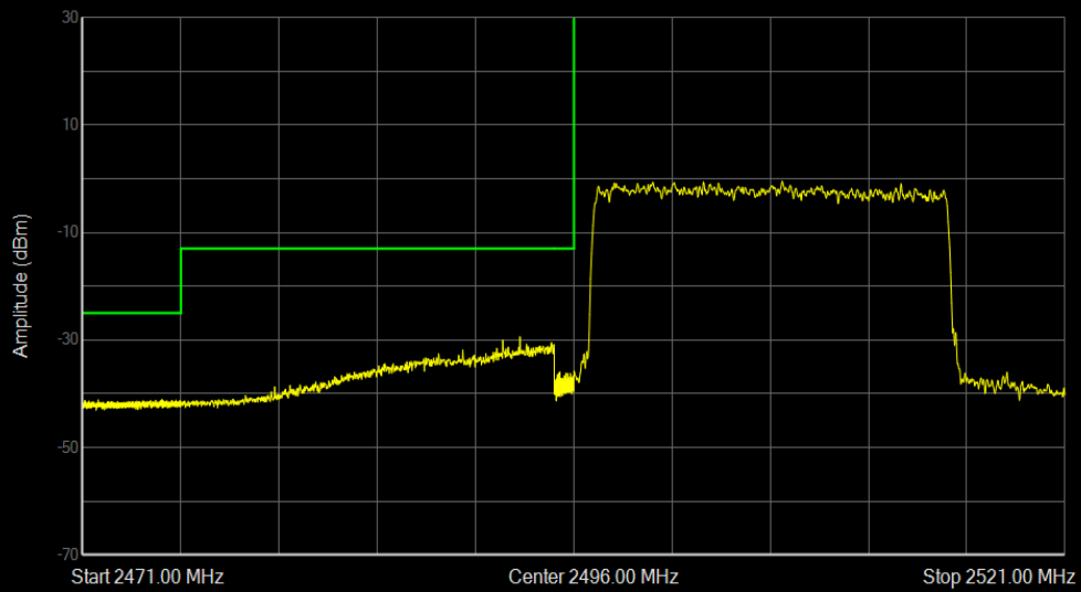
Band41 16QAM BW=20MHz Channel=39750 RB Size=100 Position=#0
