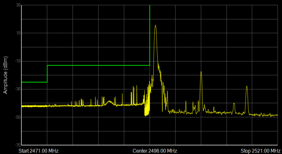
Band41 16QAM BW=20MHz Channel=39750 RB Size=1 Position=#0
