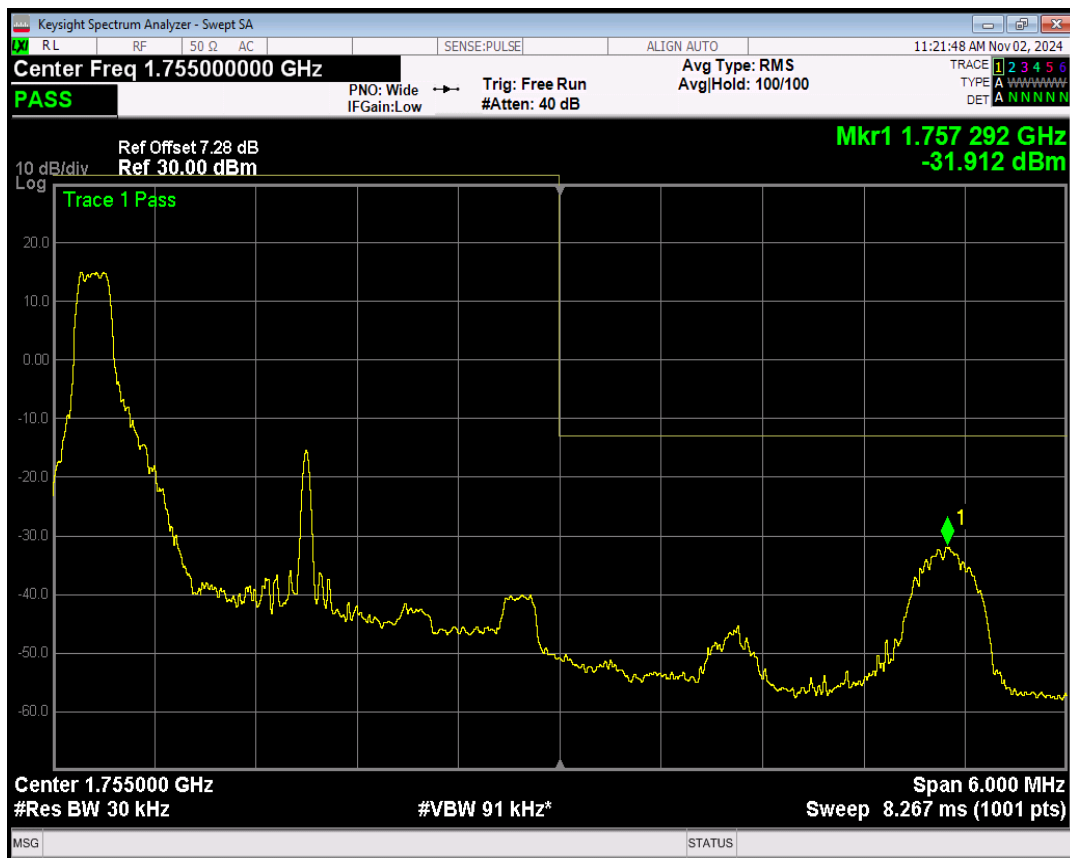
Band4 16QAM BW=3MHz Channel=20385 RB Size=1 Position=#Max
