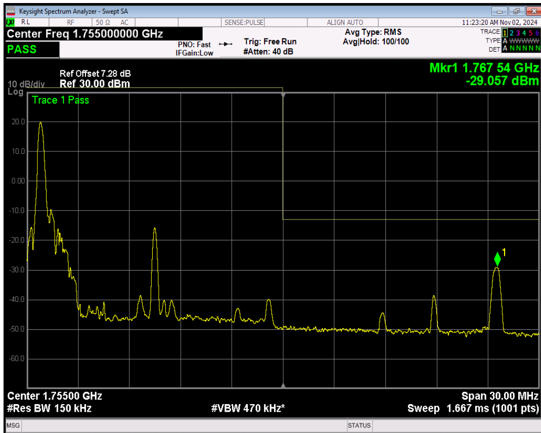
Band4 16QAM BW=15MHz Channel=20325 RB Size=1 Position=#Max
