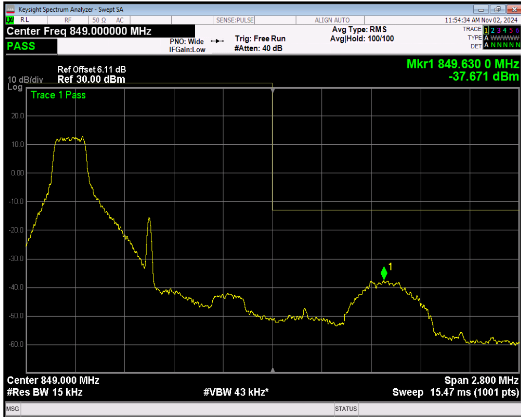
Band5 QPSK BW=1.4MHz Channel=20643 RB Size=1 Position=#Max
