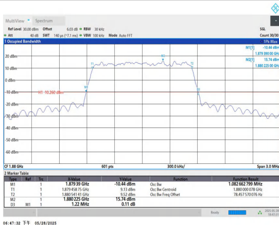
Band2-1.4MHz-16QAM-18900-6RB#0-PASS
