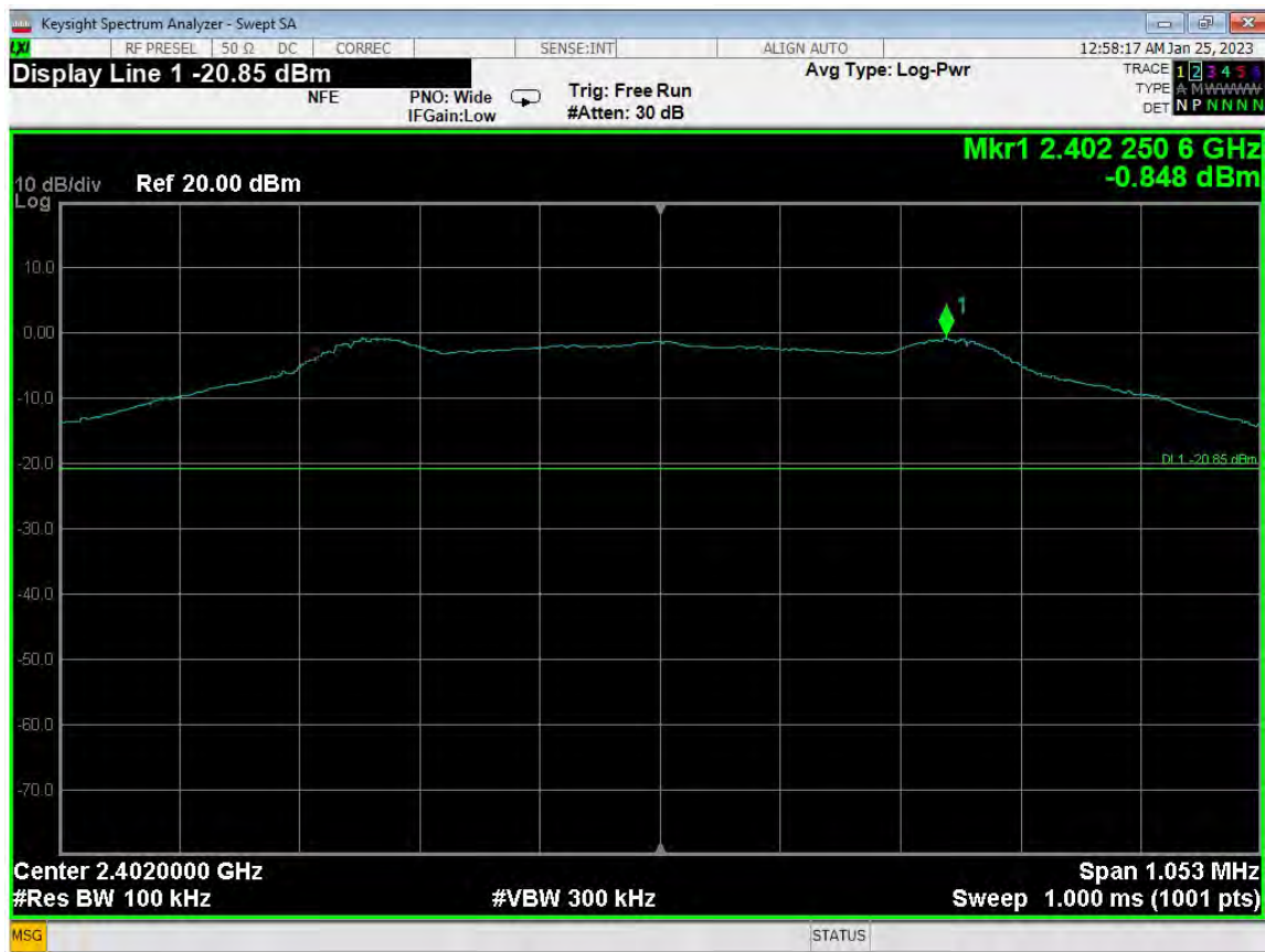
RF Antenna Conducted Test – Low Channel – Reference Level
