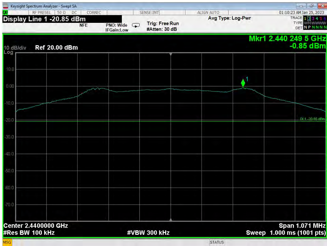
RF Antenna Conducted Test – Mid Channel – Reference Level
