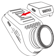
① Installing the GPS Mount
