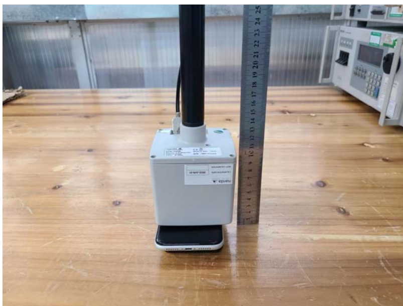
Test Position E-0cm from the edge of EUT to the geometric center of the probe
