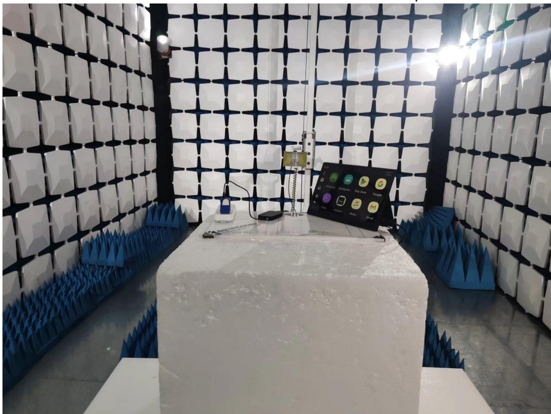
Above 1GHz for radiated emission test setup
