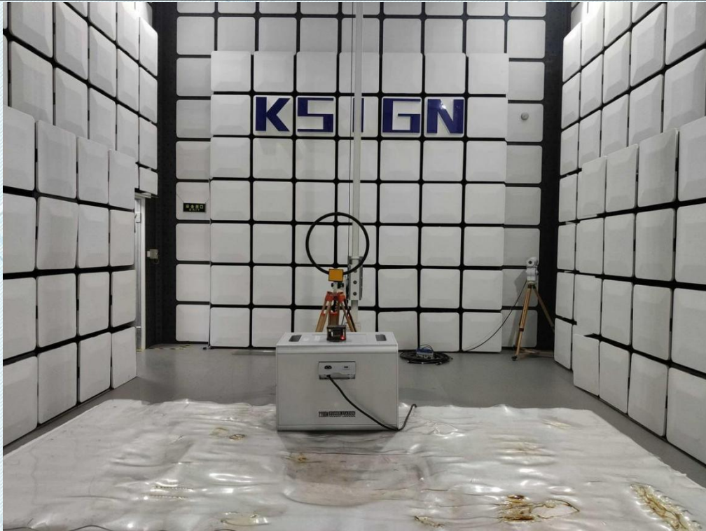
Emissions in restricted frequency bands (below 30MHz)
