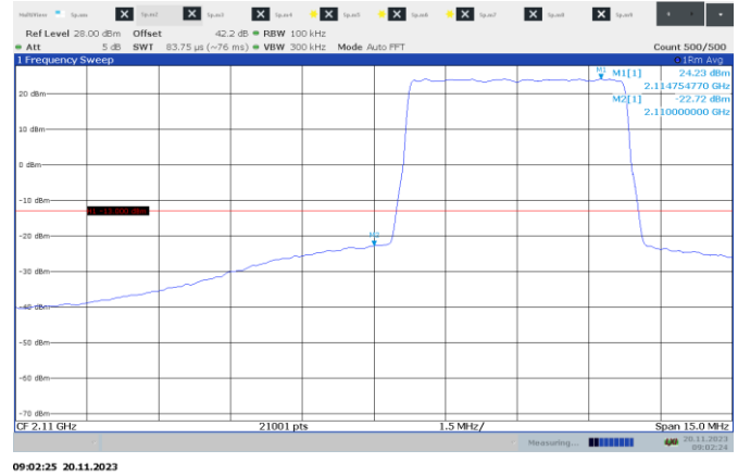
Figure 7.2-62 : Conducted band edge (RBW 1% of EBW), LTE, B 66, CH 66466
