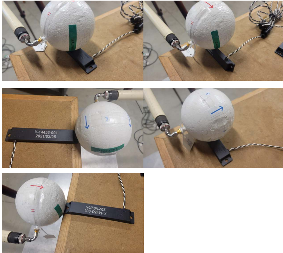
Figure 4: Radiated Emissions Test Setup Photograph(s).
