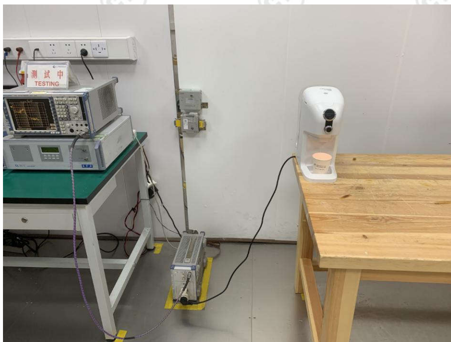
CONDUCTED EMISSION TEST SETUP
