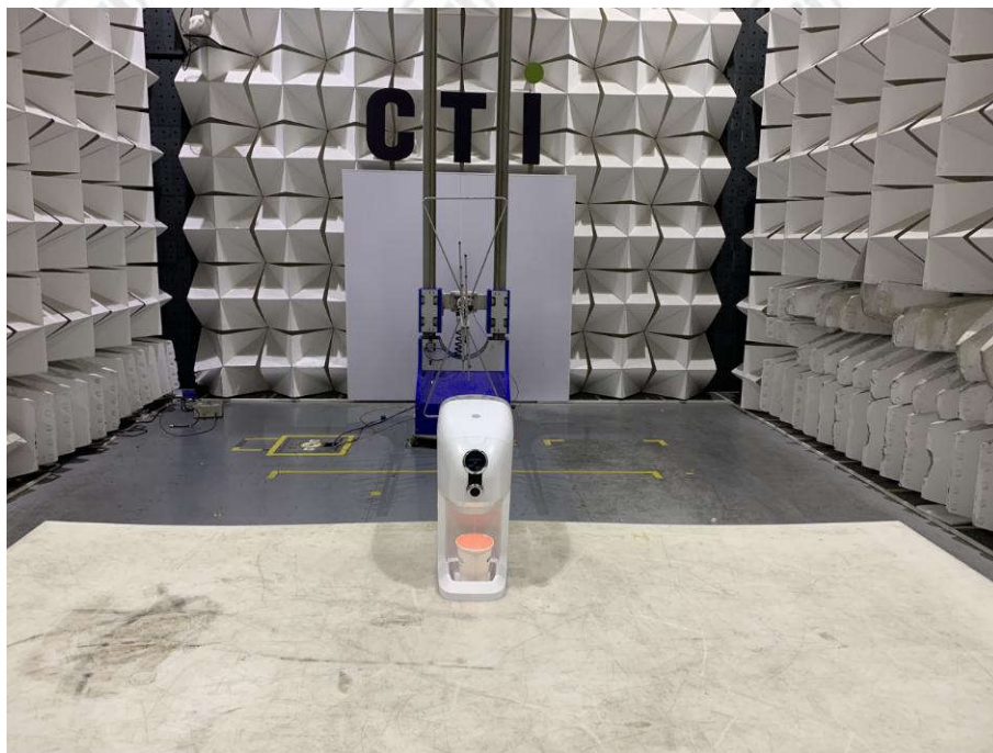
Radiated spurious emission Test Setup-1(Below 1GHz)
