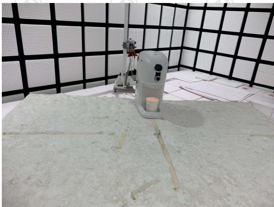
Radiated spurious emission Test Setup-2(Above 1GHz)
