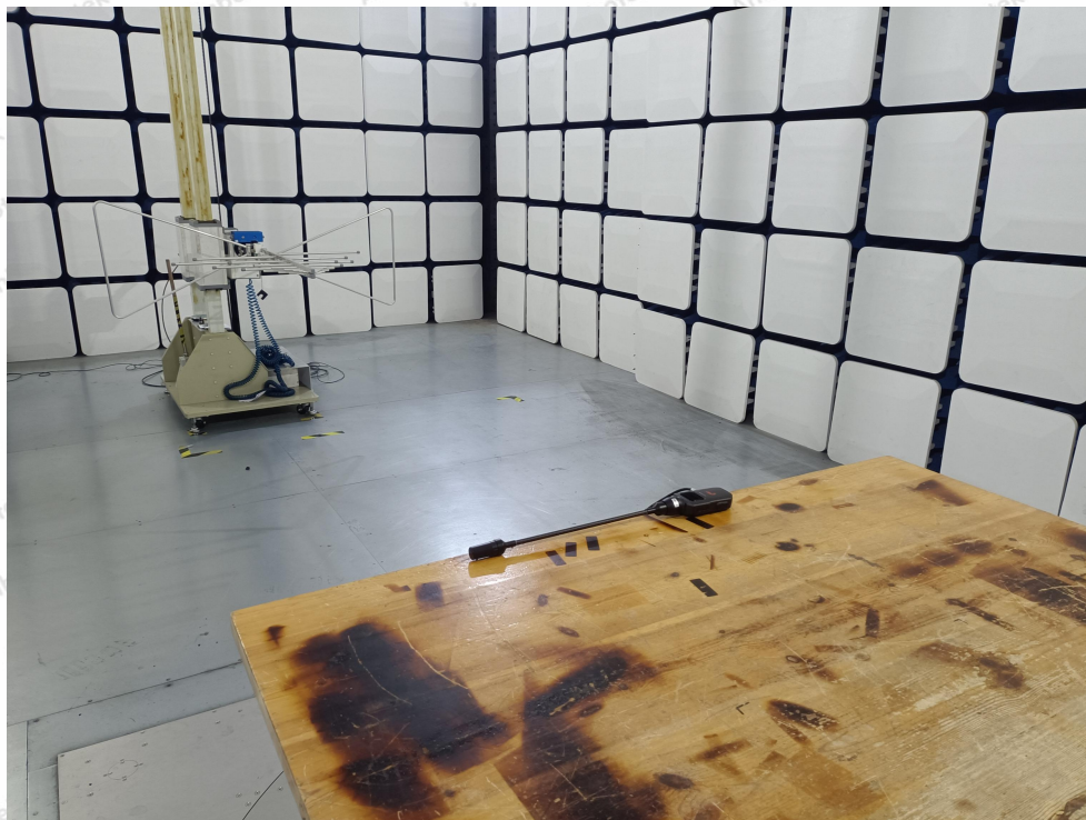
Photo of Radiation Emission Test
