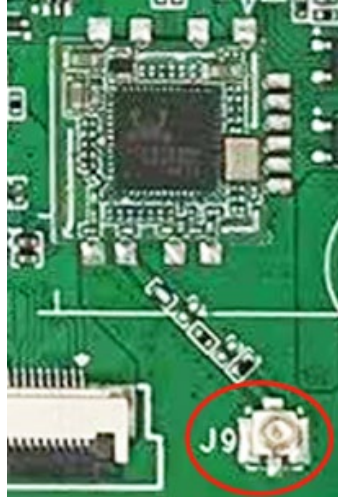
Figure 14Ido-evb3020 IPEX first generation seat
