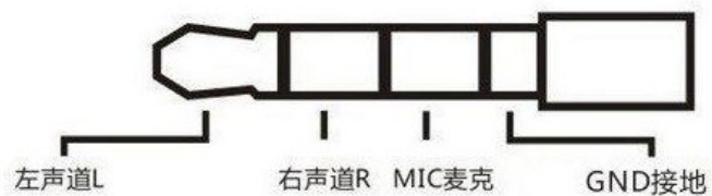
Figure 9Schematic diagram of ido-evb3020 earphone
