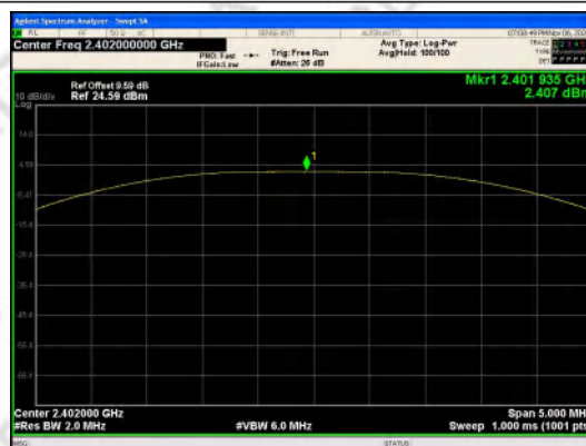
Peak Output Power BLE 2M_Channel 0
