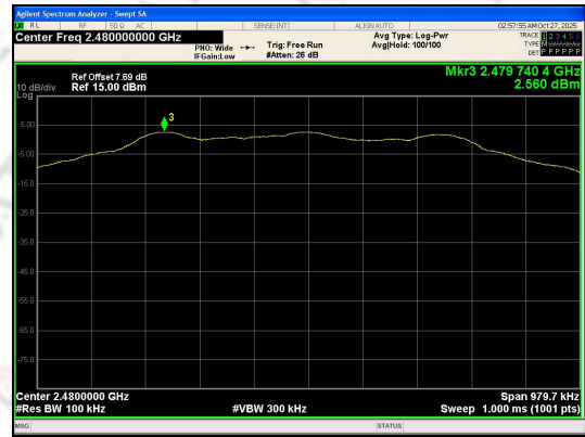
In-Band Reference Level BLE 1M_Channel 39
