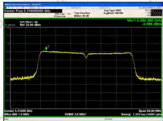
IEEE 802.11n_Channel 62_40MHz_Antenna 0
