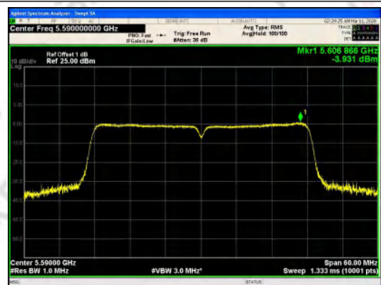
IEEE 802.11n_Channel 118_40MHz_Antenna 0
