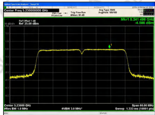
IEEE 802.11n_Channel 46_40MHz_Antenna 0
