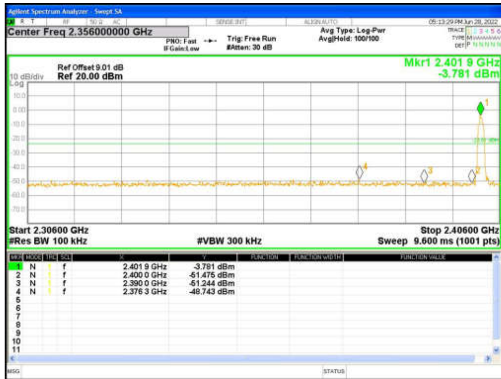
Band Edge NVNT 2-DH1 2480MHz Ant1 No-Hopping Ref
