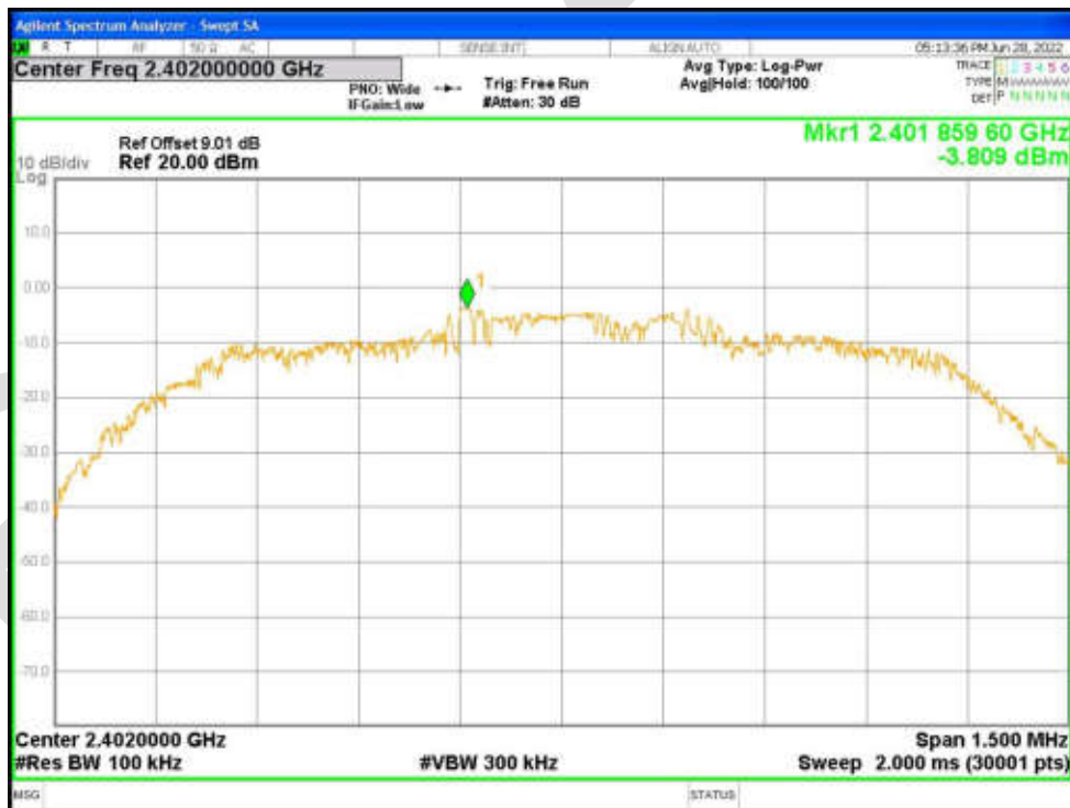
Tx. Spurious NVNT 2-DH1 2402MHz Ant1 Emission
