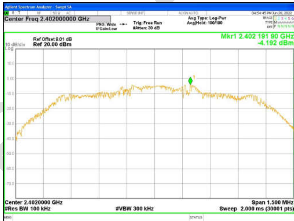
Tx. Spurious NVNT 3-DH1 2402MHz Ant1 Emission
