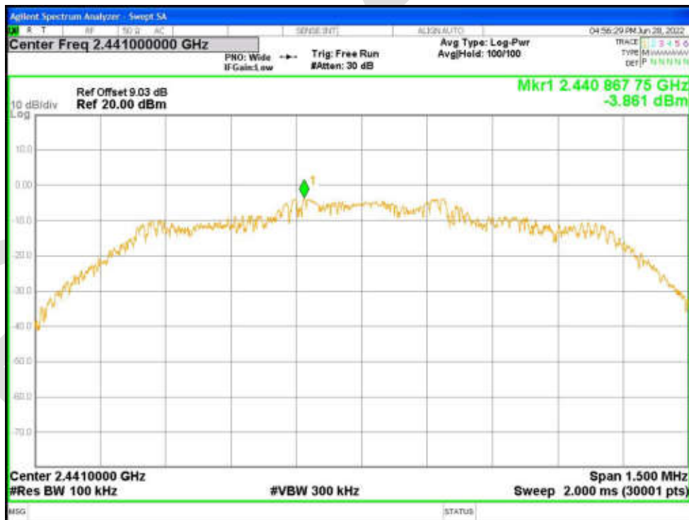
Tx. Spurious NVNT 3-DH1 2441MHz Ant1 Emission
