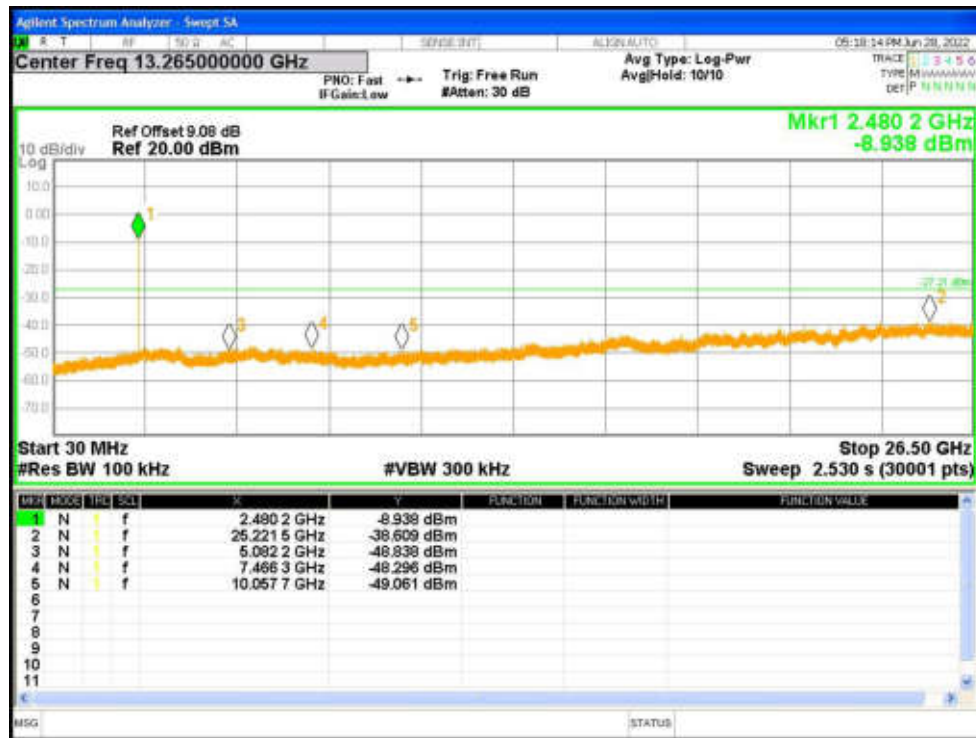
Tx. Spurious NVNT 3-DH1 2402MHz Ant1 Ref
