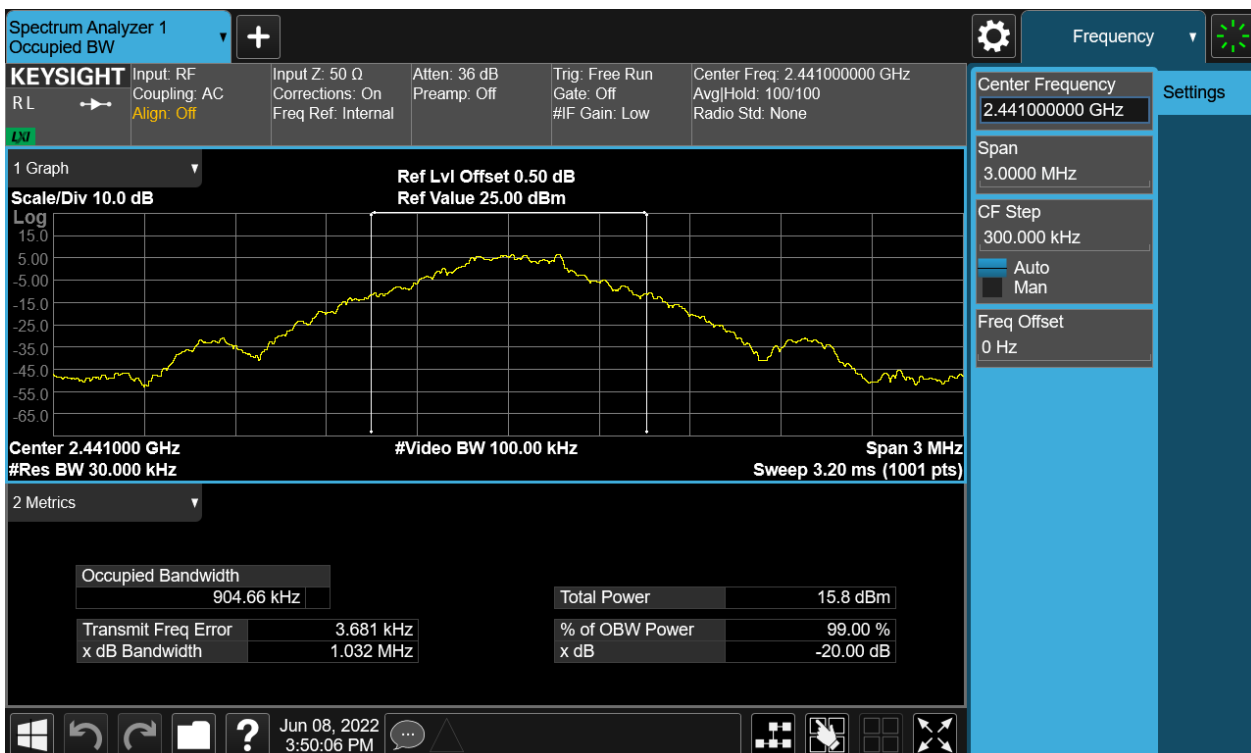
Figure 11: 20dB Bandwidth and 99% Bandwidth, 2441MHz, GFSK
