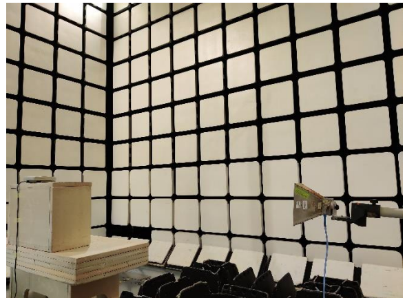
Fundamental & Spurious Emission & Restrict band radiated emission – FCC 15.231(b) and 15.205: 1 GHz – 6 GHz
