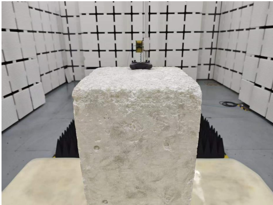
Set-up for Radiated Spurious Emission, Above 1GHz
