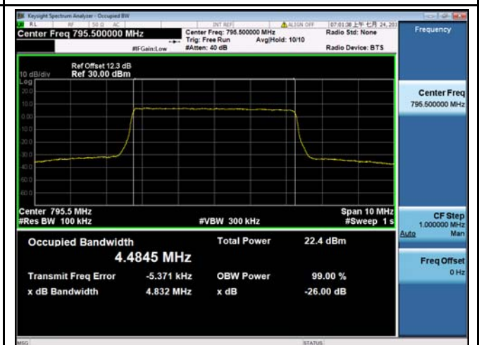
LTE band 14 - Middle CH 16QAM-5
