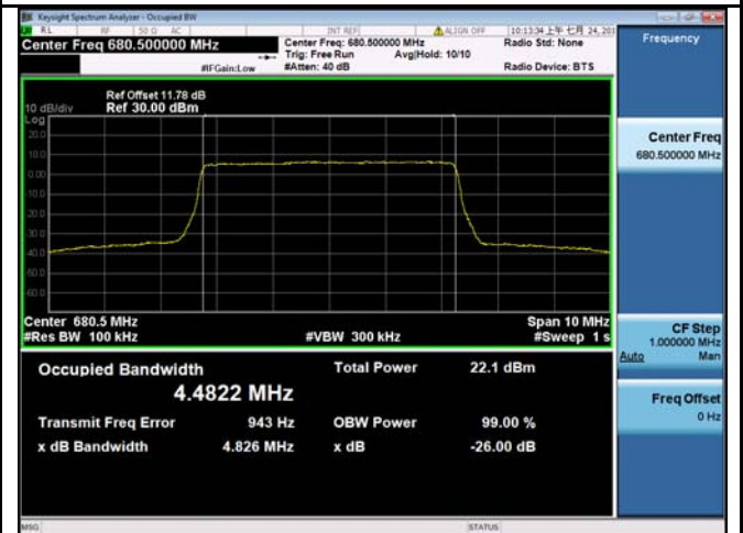
LTE band 71 - Middle CH 16QAM-5
