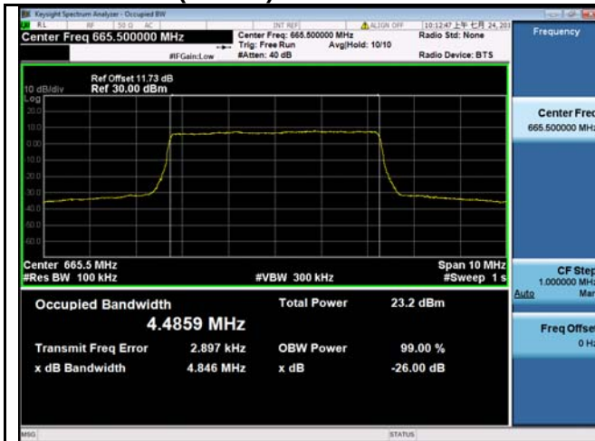
LTE band 71 - Low CH QPSK-5
