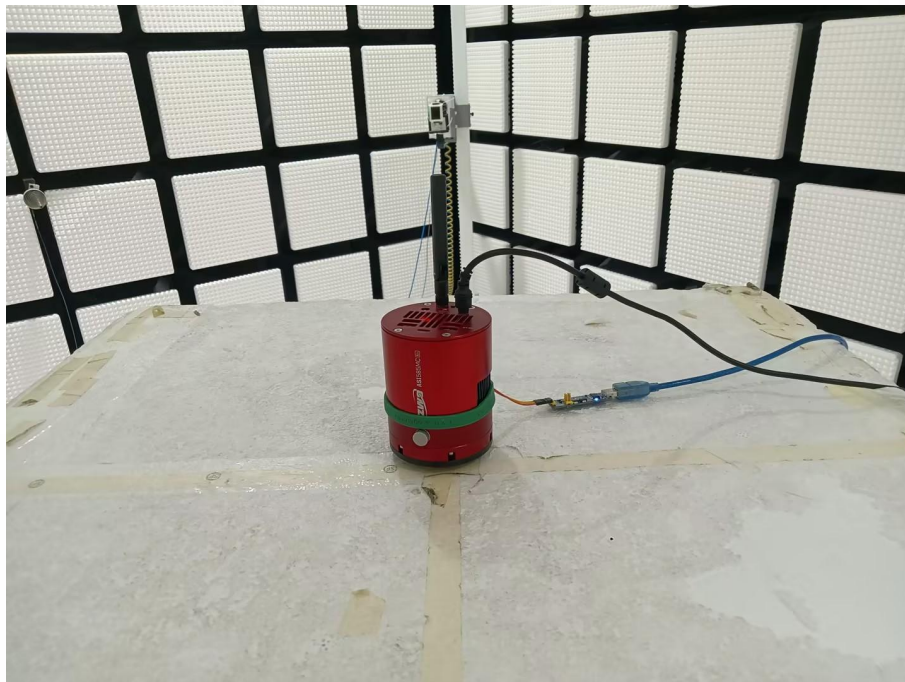
Radiated spurious emission Test Setup-3(Above 18GHz)
