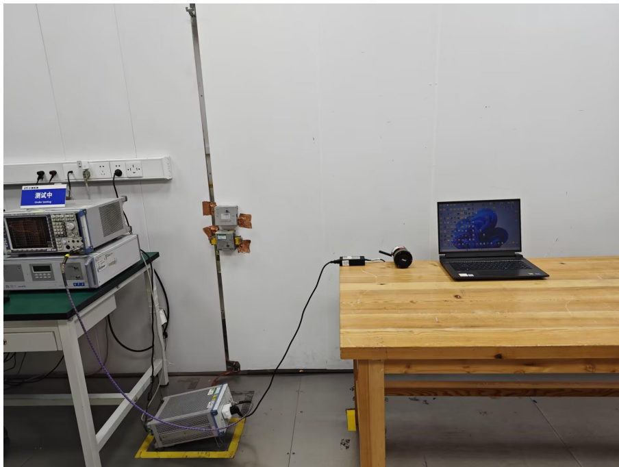
Conducted Emissions Test Setup
