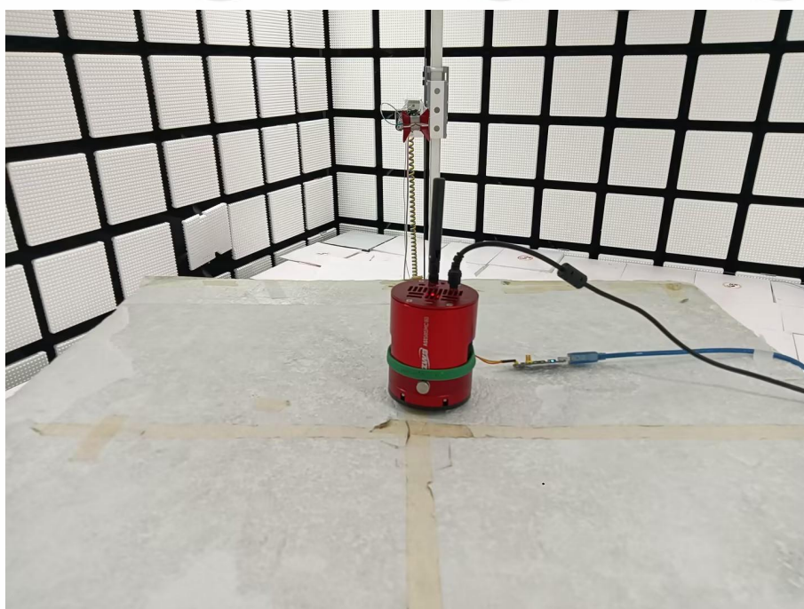
Radiated spurious emission Test Setup-2(Above 1GHz)
