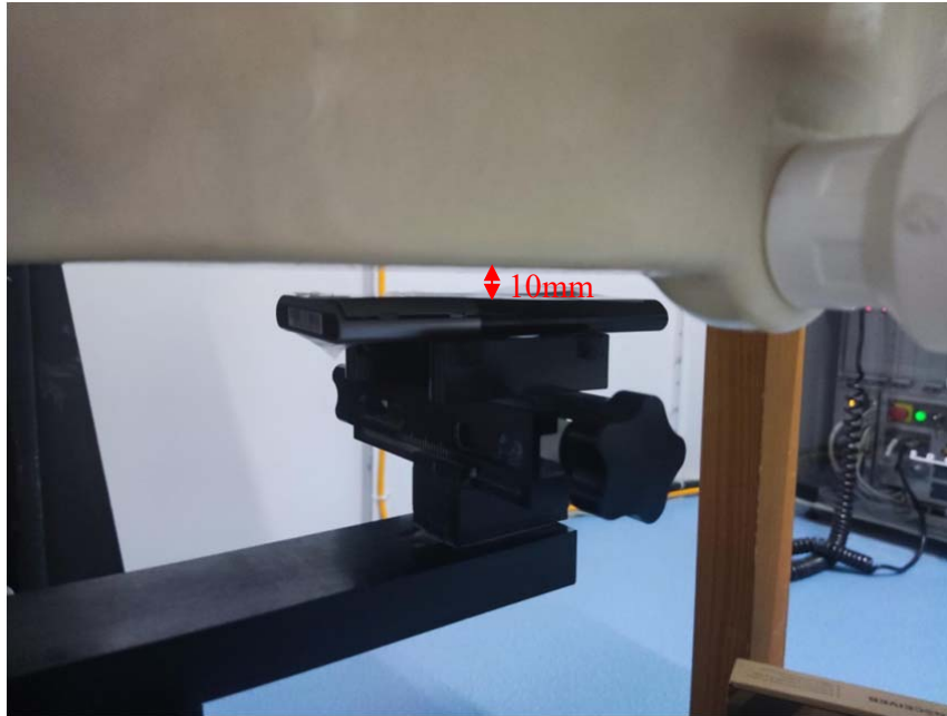
Body Back Setup Photo (10mm)
