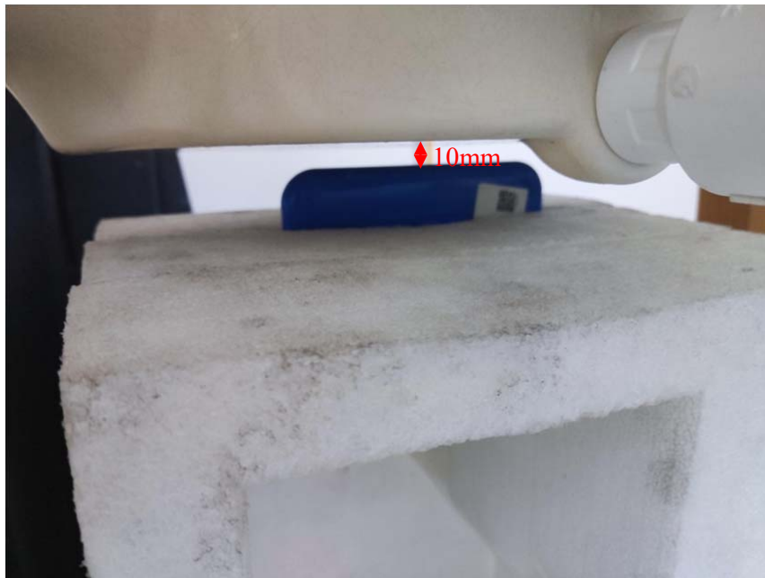
Body Right Setup Photo (10mm)
