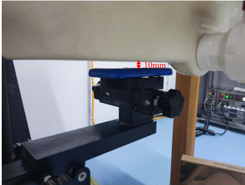
Body Back Setup Photo (10mm)
