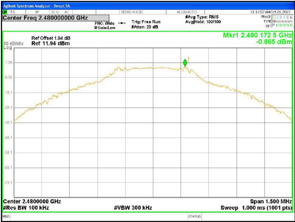
Tx. Spurious NVNT 1-DH5 2480MHz Ant1 Ref
