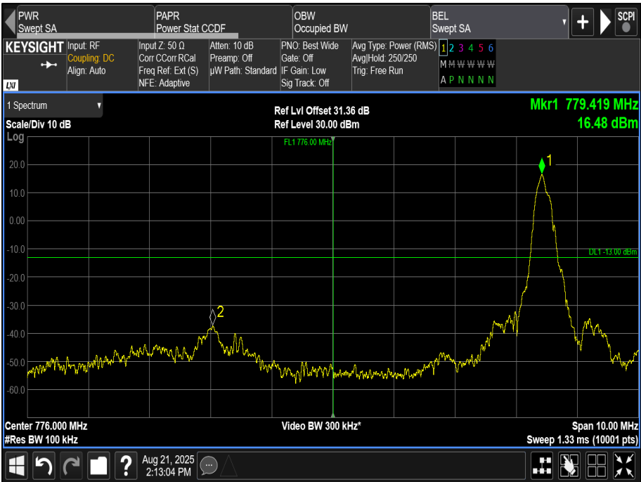
Figure 11 - Lower Band Edge, 779.5 MHz, Modulation: \pi/2 -BPSK, SCS: 15 kHz, Tone Number: 1, Start Sub-Carrier: 0
