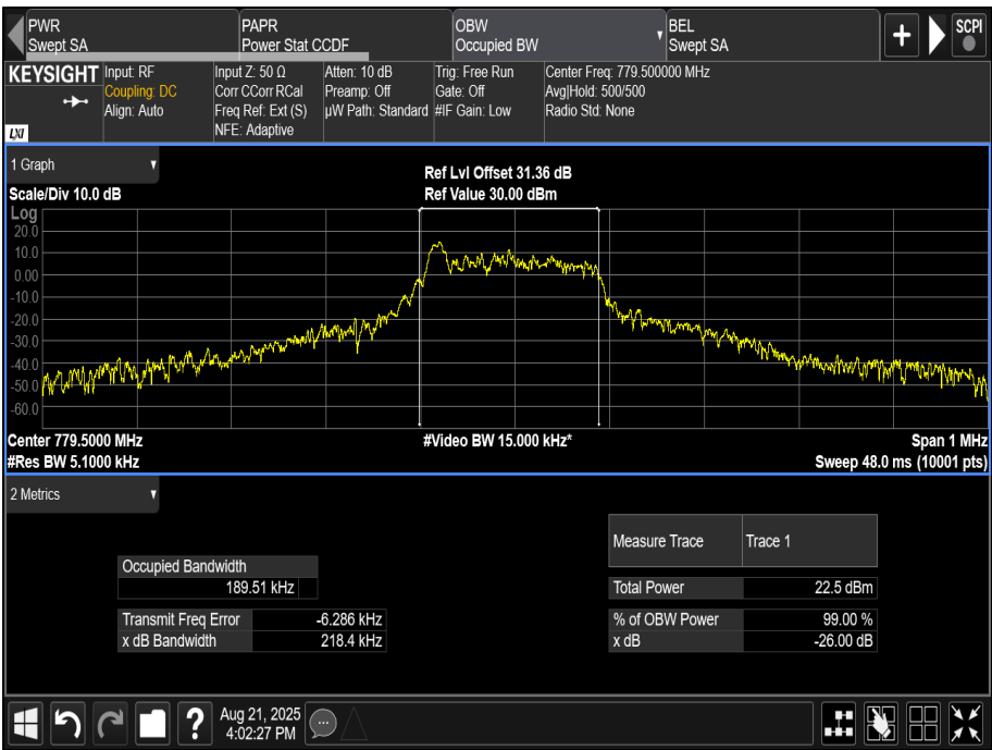
Figure 6 - Emission Bandwidth, 779.5 MHz, Modulation: QPSK, SCS: 15 kHz, Tone Number: 12, Start Sub-Carrier: 0
