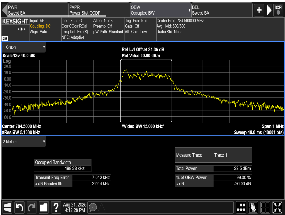
Figure 9 - Emission Bandwidth, 784.5 MHz, Modulation: QPSK, SCS: 15 kHz, Tone Number: 12, Start Sub-Carrier: 0
