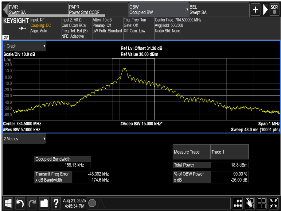
Figure 7 - Emission Bandwidth, 784.5 MHz, Modulation: \pi/2 -BPSK, SCS: 15 kHz, Tone Number: 1, Start Sub-Carrier: 0
